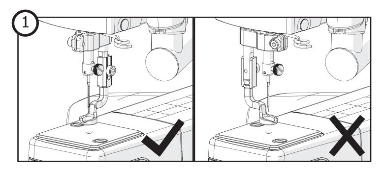
Check the position of your hopping foot. The couching attachment can only be used if the hopping foot is set directly behind the needle. See your machine manual for instructions on changing the hopping foot orientation.
