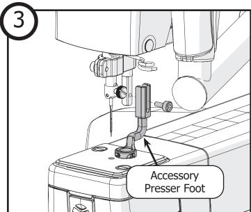
Remove the **screw** attaching the **hopping foot** to your machine using a 3 mm Allen wrench.
