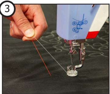
Hold the end of the top thread and move the machine to the side to pull the bottom thread (shown here in red) above the fabric. Pull up the entire tail of bottom thread.
