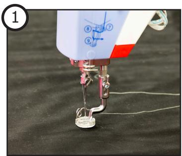
When you are ready to begin quilting with yarn or specialty thread and the couching foot has been installed, needle up and down one time.
