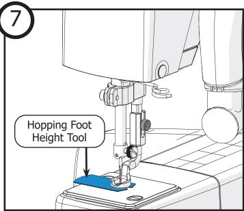
Set hopping foot height: move the machine off of the fabric and drop the needle to the lowest position. Slide the the **hopping foot height tool** beneath the foot. Tighten the hopping foot screw with the 3 mm Allen wrench.
