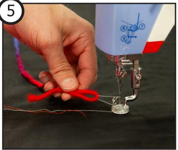
Make a loop with the yarn, and then pull it forward, under the needle so that it catches on the thread. Do a single stitch (needle down once and back up) to anchor the yarn.
