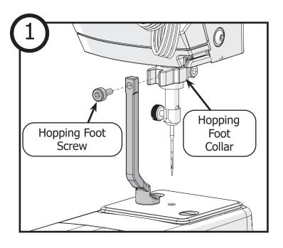
Use a 3 mm Allen wrench to remove the **screw** attaching the hopping foot to the **hopping foot collar** on your machine.
