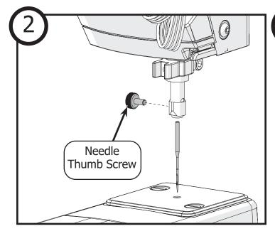
Remove the **needle thumb screw** and pull the needle from the machine.
