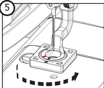
Align the black mark on the accessory presser foot with the red mark on the attachment, and press the attachment up onto the foot.
