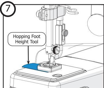
Loosen the **hopping foot screw** holding the accessory presser foot to the collar rod with a 3 mm Allen wrench. Use the hand wheel to drop the needle to the lowest position.
