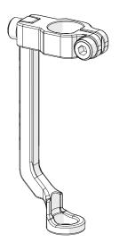
If this is the hopping foot on your machine, go to "Upgrading the Hopping Foot" on page 4.
