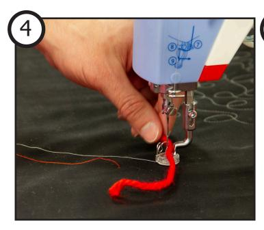
Insert the tail of the yarn or specialty thread between the needle and hopping foot, behind the thread.
