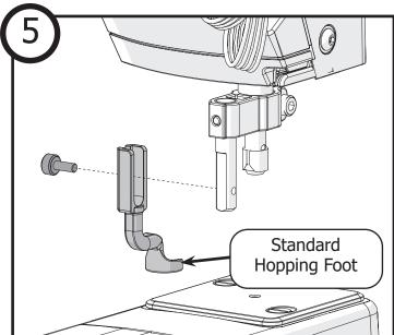
Slide the hopping foot collar that came with this kit onto the press bar. Hold in place with the hopping foot collar screw.
