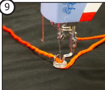
Lay the tails of the yarn and thread aside. Then take the side of the yarn on the hopping foot and tuck it into the wire guide on the couching foot.
