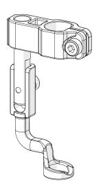
**If this is the hopping foot on your machine**, go to "Installing the Accessory Foot" on page 6.
