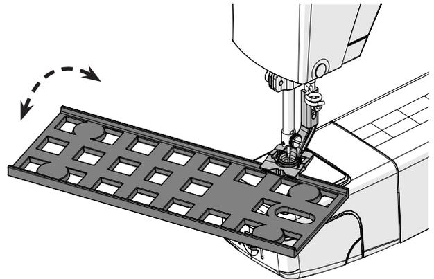
4 To release the ruler, press down on the back of the clip behind the foot and pull the ruler away from the foot.
