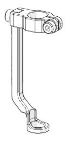
If this is the hopping foot on your machine, go to "Upgrading the Hopping Foot" on page 4.
