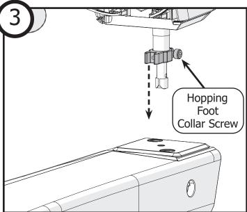
Loosen the **collar screw** with a 3 mm Allen wrench just enough that hopping foot collar can be pulled down off the machine.
