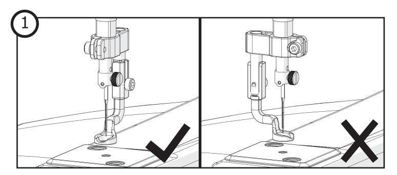
Check the position of your hopping foot. The open toe and stippling accessory feet can only be used if the hopping foot is set directly behind the needle. See your machine manual for instructions on changing the hopping foot orientation.
