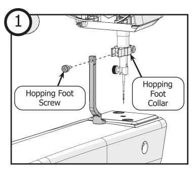
Use a 3 mm Allen wrench to remove the **screw** attaching the hopping foot to the **hopping foot collar** on your machine.
