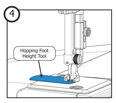
Set hopping foot height: move the machine off of the fabric and drop the needle to the lowest position. Slide the the **hopping foot height tool** beneath the foot. Tighten the hopping foot screw with the 3 mm Allen wrench.
