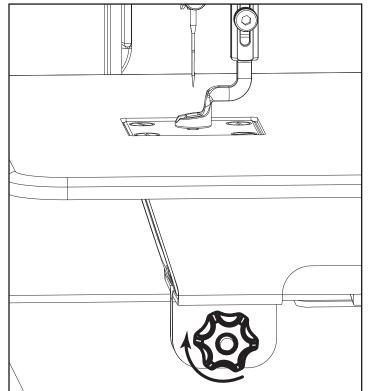
Press the ruler base onto the sewing machine until it has fully seated.
