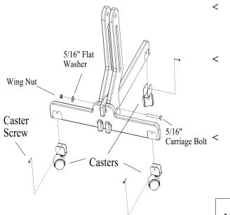
With the parts in place as pictured (left), thread the carriage bolt through the holes at the bottom of the Lower Stands and the Front Base Leg.
