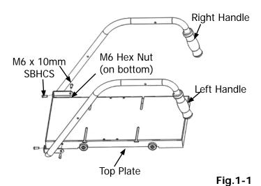
Attach the Right and Left Handles to the Bottom Plate using (4) M6 x 10mm SBHCS and (4) M6 Hex Nuts (see Fig.1-1). Place the Handle Brace across the two Handles (see Fig.2-2).
