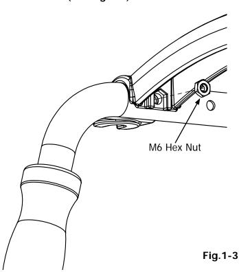
While holding the M6 Hex Nuts in place, insert (2) M6 x 40mm SBHCS into the holes on the outside of the Handle Brace and secure them into the M6 Hex Nuts with the 4mm Allen Wrench (see Fig.1-4).
