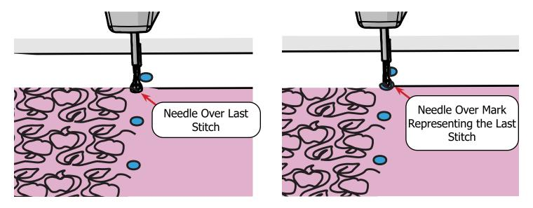
3 With the needle in position, tap the left node on the screen.
