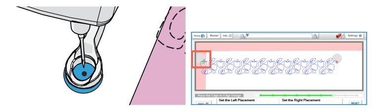
2 Move your needle directly over the hole you made in the sticker on the right side of the frame. Press the gray node on the right side of the screen so the node turns green.
