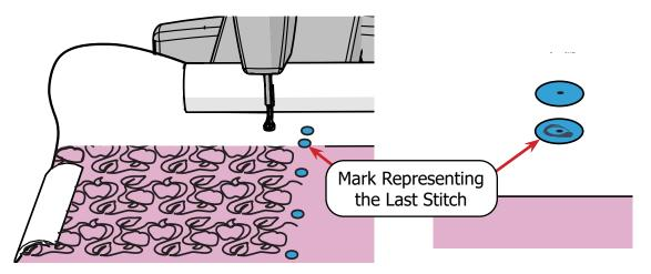
2 Move the machine so the needle is directly over the last stitch or over the mark representing the last stitch.
