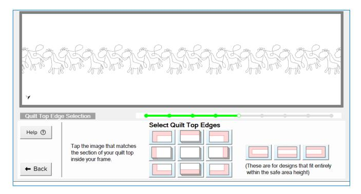
Measure out 9 inches from the frame's right side rail. If 9 inches from the rail is over the quilt-top, select the top-middle button. If 9 inches from the rail is over batting, select the top-right button.
