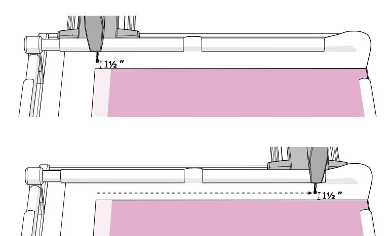
If your machine can do this without bumping into anything on the take-up rail, your fabric is positioned very well on the frame.
