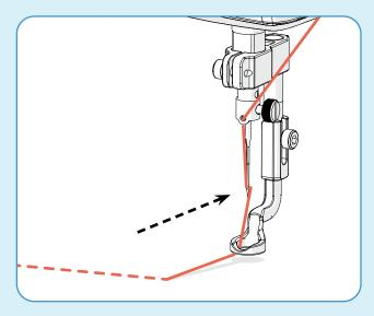
b Hold the top thread to make a loop and return the needle to the last stitch.
