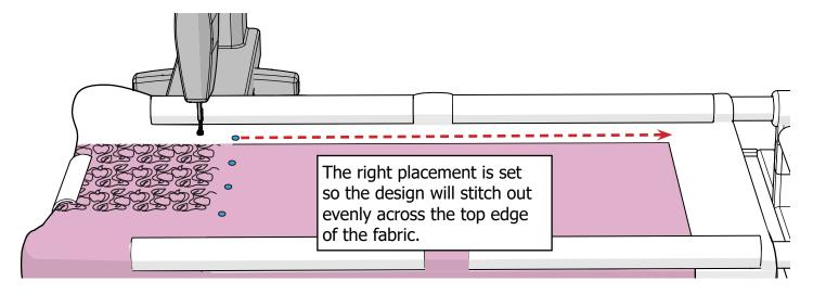
On the screen, tap **Move Right**. The machine travels to the corresponding right placement point.
