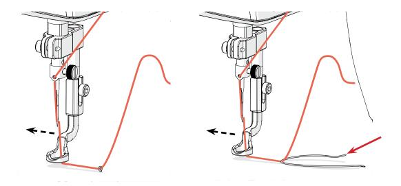
3 Move the machine back to the first stitch. Lay the two thread tails out of the way (onto the batting, if possible). You don't want automation to stitch over the tails accidentally.
