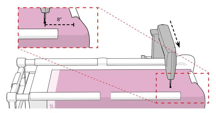
4 With the needle positioned, tap the button on the screen that says **Bottom Right**.
