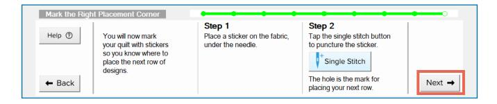
5 If you're working along the left edge of your quilt, the machine travels to the left side of the frame and the Mark the Left Placement Corner screen opens. Repeat steps 2–4 with a new sticker on the left side of the frame.
