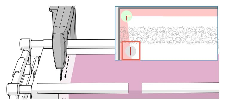
5 Slide the machine to the other side of the frame and align the needle with the top edge and tap the corresponding node.
