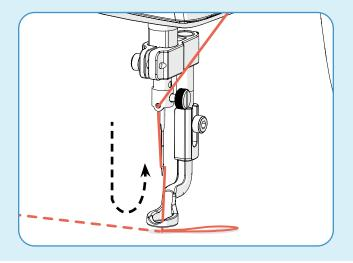
d Still holding the loop, move the machine away from the last stitch.
