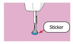
3 Press **Single Stitch** on the screen to puncture the sticker. The hole is the exact point you will use when placing the row later.
