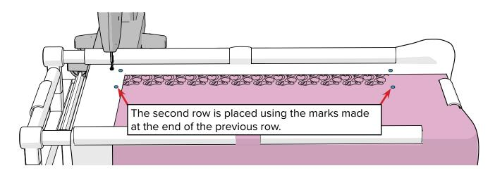
Using the skills you have already practiced, you will point with your machine's needle and press the nodes on the screen to tell the software where to stitch out the next row of designs.
