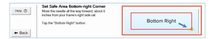
The safe area determines where the automation allows you to place designs. It important to get as much of the quilt top in the safe area as you can while still ensuring the machine cannot bump into the frame's sides or rails.
