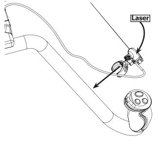
2- Plug laser into the back of the display hub in to the DC Connecter Port.
