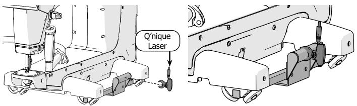
Change the diameter of the laser beam by switching between the four **laser tips**. The tips can be popped on or off the end of the laser. **For your safety:** turn off the laser before swapping out the laser tips. Never look into the laser beam.
