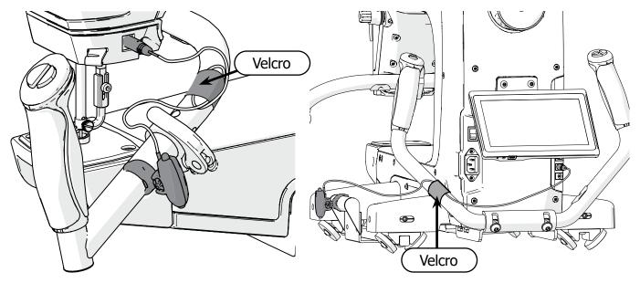
**Note:** Cable path will vary by machine model.
