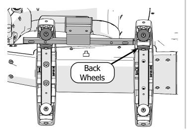
4 Align the holes in the bracket with those between the wheels. Use two **M6 x 20 mm SBHCS** and the 4 mm Allen wrench to screw the bracket in place.
