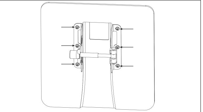
If it is difficult to get the ruler base onto the sewing machine, slightly loosen the screws on the bottom of the ruler base. Slide the metal supports farther apart, then tighten the screws. Do not over-tighten; only tighten until the ruler base feels secure.
