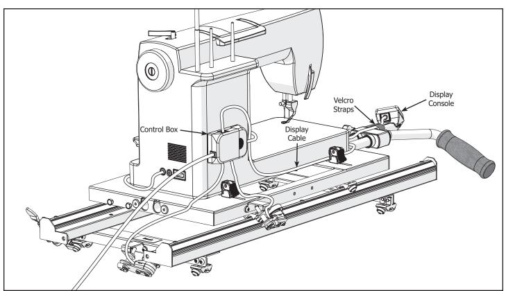
3-6 Attach the Display Cable to the Display Console and the Control Box. **Be sure the pins line up to avoid bending them**. Secure the cable to the Carriage using the Velcro Straps.
