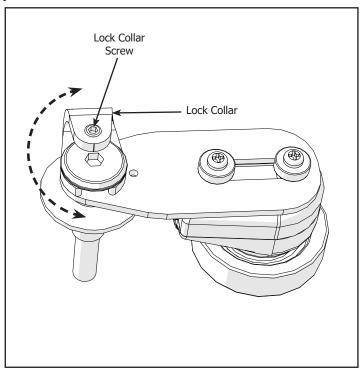
1-1 With the 2mm Allen Wrench, loosen the Lock Collar Screw so that the Lock Collar twists freely.
