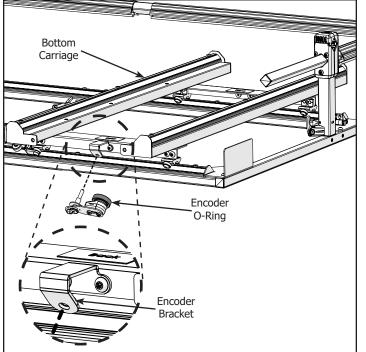
1-2 Install the Encoder onto the Bottom Carriage Encoder Bracket with the 4mm Allen Wrench. Orient the Encoder so the O-ring is to the right of the Bracket.
