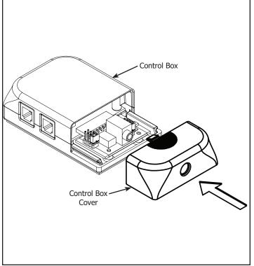
3-3 Reinstall the cover on the Control Box.
