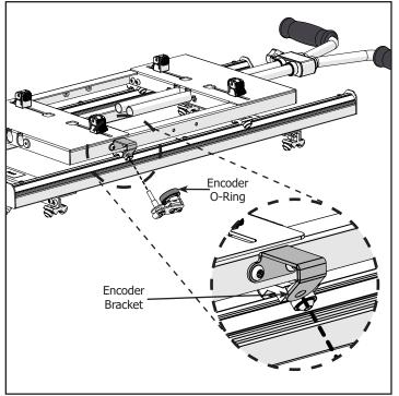
2-2 Install the Encoder onto the Top Carriage Encoder Bracket with the 4mm Allen Wrench. Orient the Encoder so the O-ring is to the right of the Bracket.
