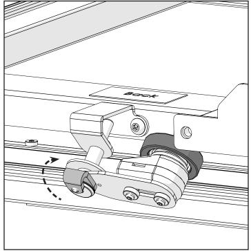
1-3 With the Bottom Carriage installed on the Tabletop Frame tracks, turn the Encoder Lock Collar to point up, and tighten the Encoder Lock Collar Screw with the 2mm Allen Wrench.
