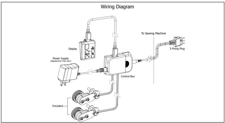
3-7 Attach the cables from each Encoder to the Control Box and secure with Zip Ties and Zip Tie Mounts. Connect the Sewing Machine Control Cable to the Control Box, and to your sewing machine's foot pedal port.
