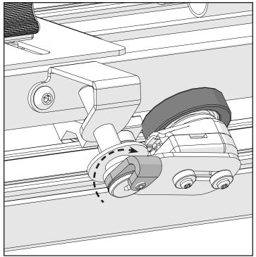
2-3 With the Top Carriage on the Bottom Carriage, turn the Encoder Lock Collar to point up, and tighten the Encoder Lock Collar Screw with the 2mm Allen Wrench.
