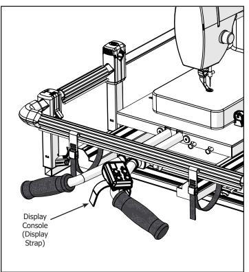
3-5 Using the Display Strap, connect the Display Console to the handles in a convenient location. **Recommendation:** Point handles downward slightly so display will not bump into fabric roll during use.
