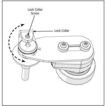
2-1 With the 2mm Allen Wrench, loosen the Lock Collar Screw so that the Lock Collar twists freely.
