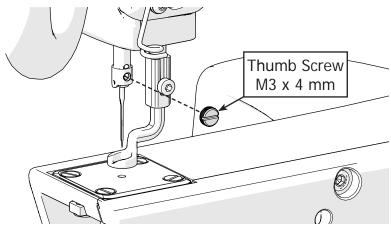
4) Use the **needle magnet** that came with your machine to align the needle, and tighten the thumb screw.
