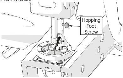
11) When moving your machine onto the fabric, slide the **inside circlet** of the hopping foot away from the **fabric edge**.
