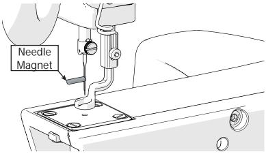
(5) Remove the standard hopping foot with the 3 mm Allen wrench.
