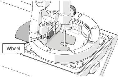
Tighten the **hopping foot screw** with the 3 mm Allen wrench.
