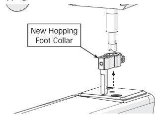
5 Place the **new standard hopping foot** onto the hopping foot collar bar. Attach with a hopping foot screw loosely enough that the hopping foot can slide up and down.
