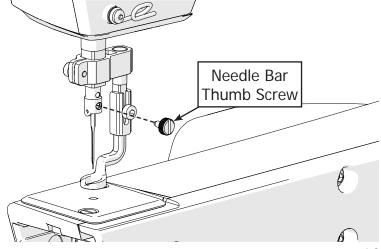
3 Hold the needle in place, and loosely attach the M3 x 4 mm thumb screw that came with the Wonderfoot.
