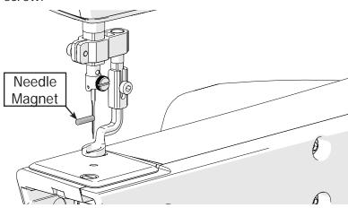
Semove the standard hopping foot with the 3 mm Allen wrench.
