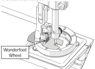
10 Tighten the **hopping foot screw** with the 3 mm Allen wrench.
