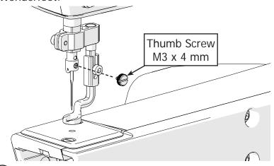
4 Use the **needle magnet** that came with your machine to align the needle, and tighten the thumb screw.
