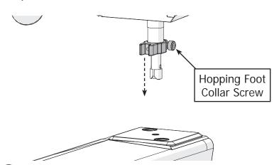
4 Slide the **new hopping foot collar** that came with this kit onto the press bar. Hold in place with the hopping foot collar screw.
