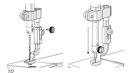
8 Slide the **height tool** under the foot, and tighten the hopping foot screw with a 3 mm Allen wrench.
