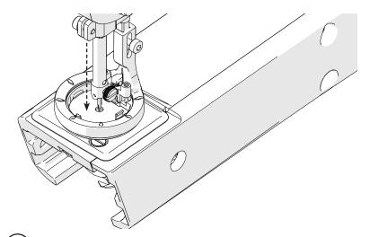
8 Slide the **height tool** under the foot.
