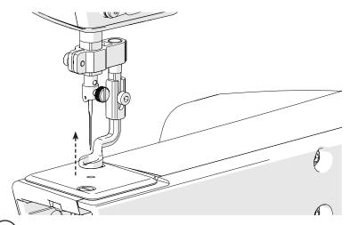
2) While holding the needle in place, remove the needle bar thumb screw.
