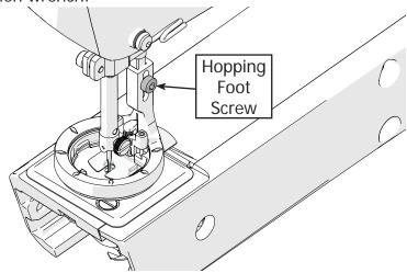
When moving your machine onto the fabric, slide the **inside circlet** of the hopping foot away from the **fabric edge**.
