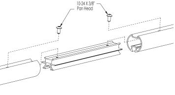
The you will put the other end of the coupler into either the "B" Pole (14"), if you are setting your frame up in Twin. If you are setting up in Queen or King you will attach the "C" Pole (36") to the coupler on the "A" Pole (57-11/16). If you are setting up in the king size then you will attach the "B" Pole (14") to the "C" Pole (36").
