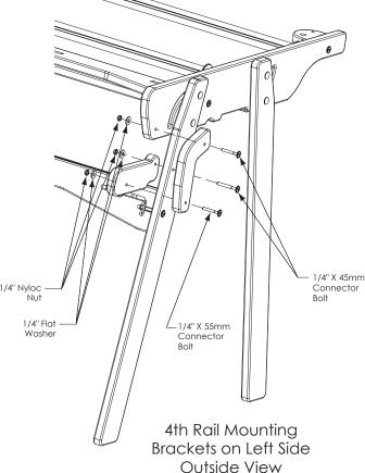
With this bracket assembly in place on both the Left and Right Ends, you are ready to insert your pole. Follow pole assembly instructions on pages 11
