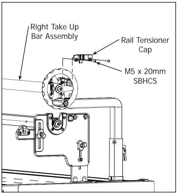
Take Up Bar Assembly using (2) M5 x 20mm Rail Bracket using (2) M5 x 20mm SBHCS. SBHCS. You will have to push down on the Rail Tensioner Cap to insert the (2) M5 x 20mm SBHCS.
