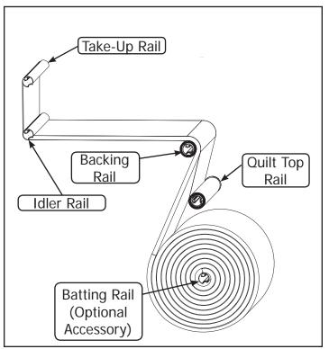
13-2 Attach the Backing Leader to the Backing Rail and ratchet the remaining fabric onto the rail. Similarly, attach the Top Leader to the Top Rail and ratchet the remaining fabric onto the rail.
