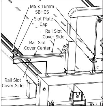
4-1 Install the Rail Slot Covers and Slot Plate Caps using (2) M6 x 16mm SBHCS from Step 1-3.
