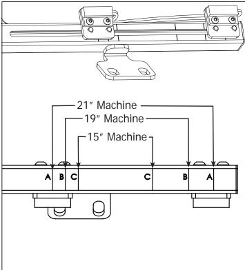
8-1 Loosen the M4 x 25mm SBHCS that secure the 8-2 Adjust each Sensor to the proper setting for your machine with the Sensor centered on the correct indication line and tighten screws.
