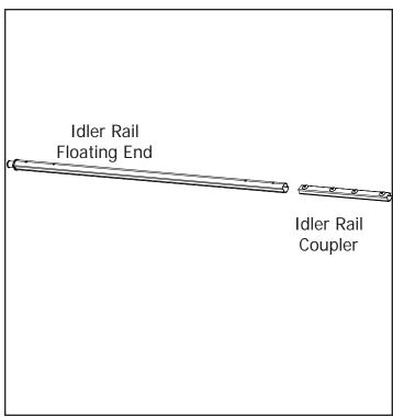
10-1 Slide the Idler Rail Coupler into the Idler 10-2 Slide the Idler Fixed End Section onto Idler Rail Floating End Section half way and align the Rail Coupler, tight against the appropriate Rail screws with the holes in the Idler Rail Floating End Section (see Step 10-3), and secure rail by backing Section. Secure Idler Rail Coupler by backing the screws out. screws out.
