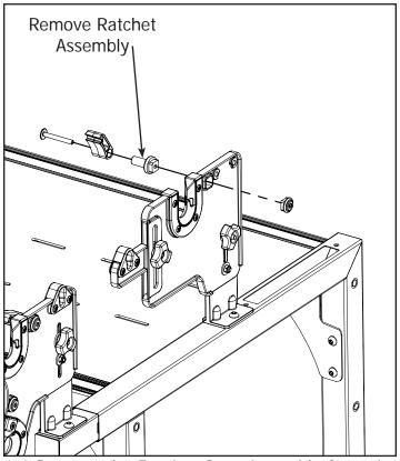
1-4 Remove the Ratchet Stop Assembly from the Ratchet Back Rail Support using the 4mm Allen Wrench.
