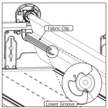
13-4 Place the lower side of the Fabric Clip into the 13-5 Press the Fabric Clip over the fabric until it lower groove of the Idler Rail.
