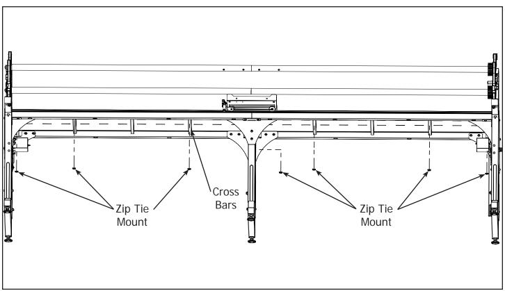
7-3 Secure (7) Zip Tie Mounts to the bottom of the frame by removing the paper from the double faced tape and sticking them to the cross bars on the underside of the tables.
