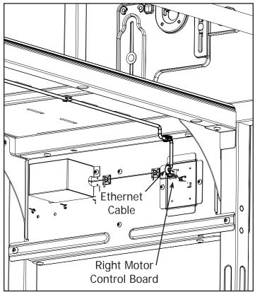
7-2 Connect the Ethernet Cable to the Right Motor Control Board.
