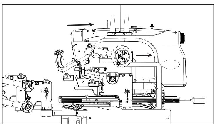
15-2 As you move your Sewing Machine back past the rear Sensor on the Open Market Bracket, the Take Up Rail will move backwards to allow for increased quilting area.
