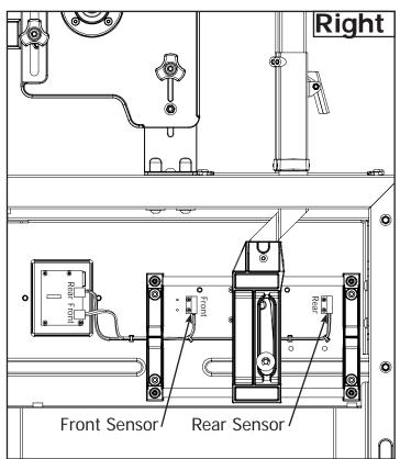
Verify the Sensors are plugged into the correct Verify the Sensors are plugged into the correct ports on the Motor Control Board for the Left ports on the Motor Control Board for the Right Frame Side.
