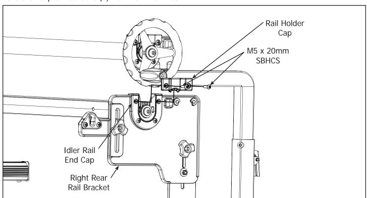
11-5 Install the Rail Holder Cap onto the Right Rear Rail Bracket using (2) M5 x 20mm SBHCS. Note: Make sure the the Idler Rail End Cap inserts into the Rail Holder Cap.
