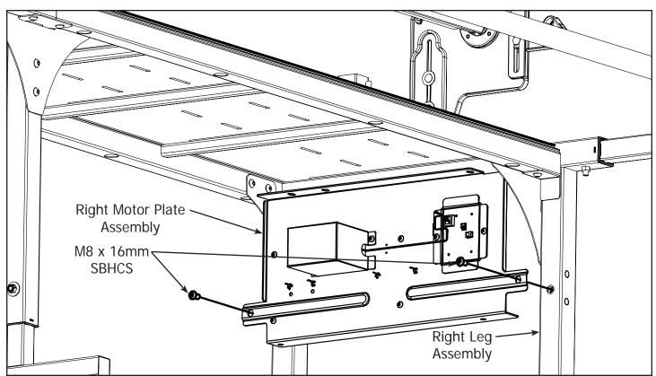
2-3 Secure the Right Motor Plate Assembly to the Right Leg using (2) M8 x 16mm SBHCS.
