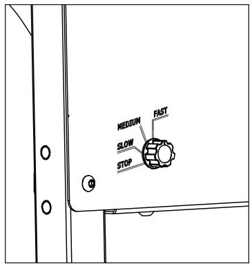
12-6 Turn the Speed Control Knob to the desired speed to turn on the Gliding Rail. Turn the Speed Control Knob to Stop to center the rail and stop movement.
