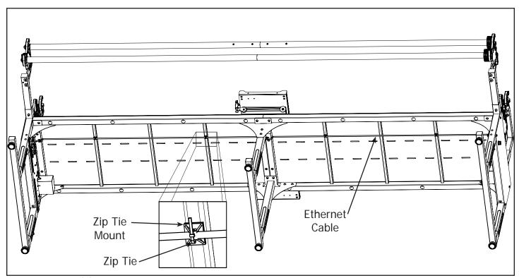
7-4 Insert the (7) Zip Ties into the Zip Tie Mounts and use them the secure the Ethernet Cable to the bottom of the table.
