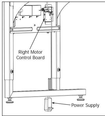
12-1 Plug the Power Supply into the back of the Right Motor Plate Assembly.
