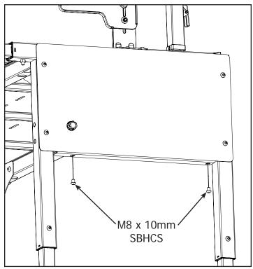
6-5 Install the (2) M8 x 10mm SBHCS and tighten all (6) screws.
