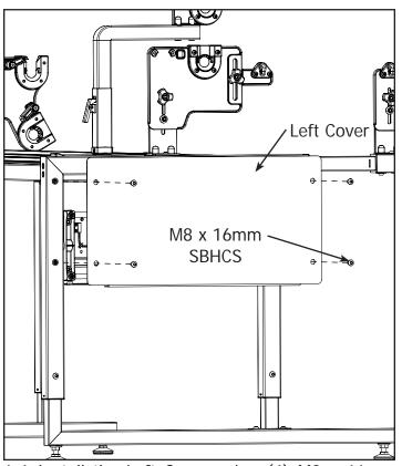
6-1 Install the Left Cover using (4) M8 x 16mm 6-2 Install the (2) M8 x 10mm SBHCS and tighten SBHCS.
