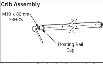
10-1a Loosen the M10 x 80mm SBHCS to remove Floating Rail Cap from the Floating Rail Section.
