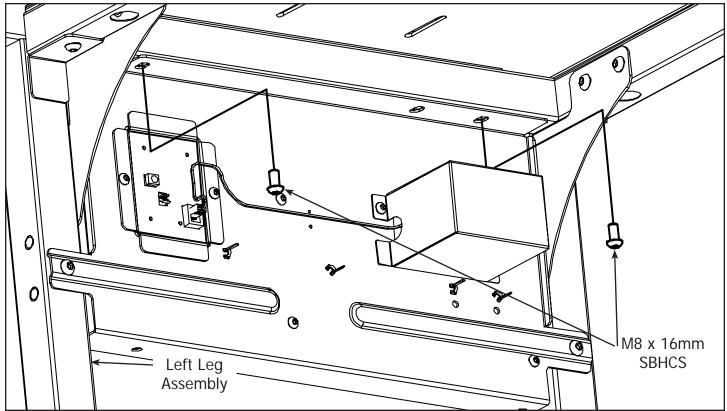
2-2 Secure the Left Motor Plate Assembly to the Left Leg using (2) M8 x 16mm SBHCS.
