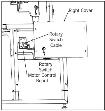
6-3 Plug the Rotary Switch into the Motor Control 6-4 Install the Right Cover using (4) M8 x 16mm Board.
