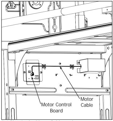
5-1 Plug in the Motor Cable to the correct port on the Motor Control Board for each side.
