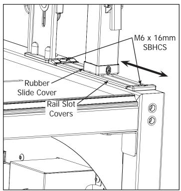
12-7 Move the Sewing Machine forward and back to verify there is no binding on the Slot Covers. If binding occures, adjust the Rail Slot Covers.
