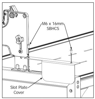
1-3 Remove the Slot Plate Covers from the right and left side by removing the (2) M6 x 16mm SBHCS from each side using the 4mm Allen Wrench.
