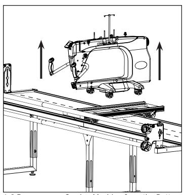
1-2 Remove your Sewing Machine from the Bottom Carriage.
