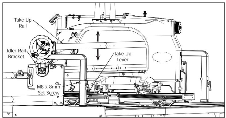
12-4 Adjust the height of the Take Up Rail by pressing in on the lower side of the Take Up Lever. Raise or lower the Take Up Rail so it is approximately centered in your machine, and the Gliding Rail does not rub on the Idler Rail Bracket. Make sure the Take Up Rail is level. Tighten the M8 x 8mm Set Screw on each side.
