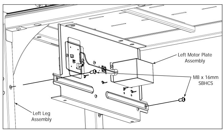
2-1 Secure the Left Motor Plate Assembly to the Left Leg using (2) M8 x 16mm SBHCS.
