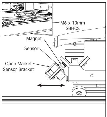
9-3 Adjust the Open Market Sensor Bracket so there is less than 1/4" between the Sensor and the Magnet. Tighten the (2) M6 x 10mm SBHCS on the Open Market Sensor Bracket.
