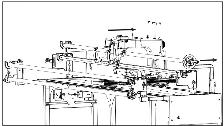
14-1 Move your sewing machine forward and backward a minimum of 10 times slowly making sure the Rail moves forward and back completely in order to calibrate the Gliding Rail System.
