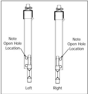
3-1 Identify the difference between the Right Take Up Rail Mount Assembly and the Left Take Up Rail Mount Assembly.
