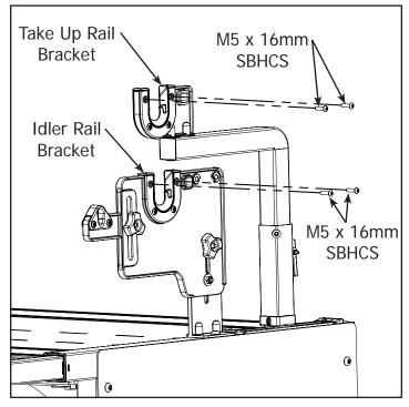
11-1 Remove the (2) M5 x 16mm SBHCS from the top of the Right Take Up Rail Bracket and the Right and Left Idler Rail Bracket.
