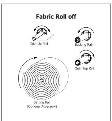
13-3 Fabric should roll off of the rails as shown in the images above. The Take-Up Rail has no particular direction of rotation and can be rotated either way without effecting the frames performance.
