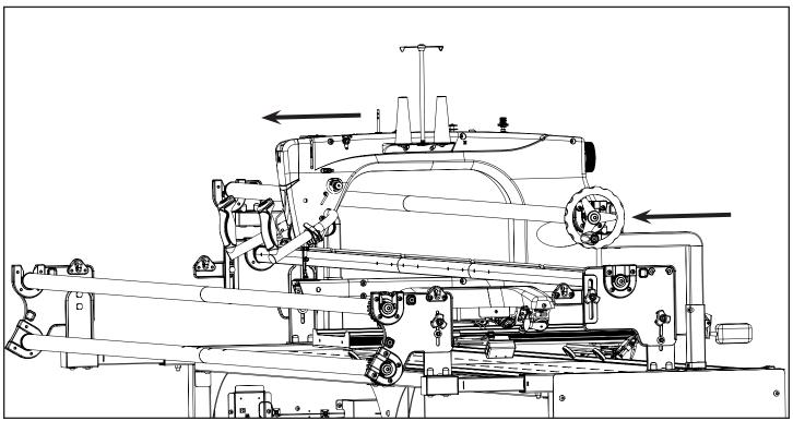
15-1 As you move your Sewing Machine forward past the front Sensor on the Open Market Bracket, the Take Up Rail will move forward to allow for increased quilting area.
