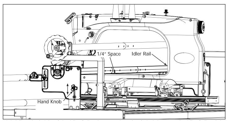
12-5 Adjust the height of the Idler Rail to be approximately 1/4 inch between the Idler Rail and the sewing machine. Make sure the Idler Rail is level and does not rub on your machine. Tighten the Hand Knob on both sides.
