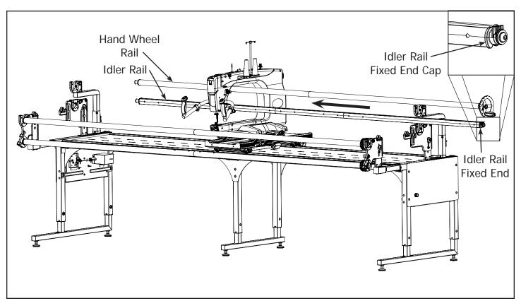
11-2 Install the Hand Wheel Rail and the Idler Rail by sliding through the throat of the Sewing Machine and inserting into the Rail Brackets.
