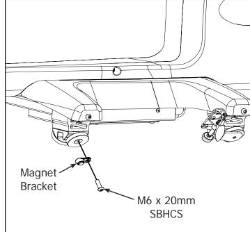
9-1 Install the Magnet Bracket onto the right front wheel of the sewing machine using (1) M6 x 20mm SBHCS.
