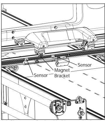
9-2 Place your Sewing Machine on the bottom carriage with the Magnet Bracket located between the (2) Sensors.
