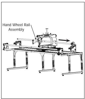
1-1 Remove the Hand Wheel Rail Assembly.
