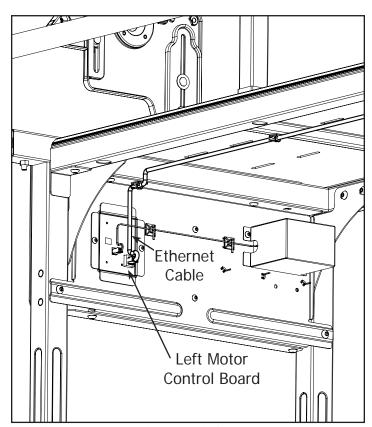
7-1 Connect the Ethernet Cable to the Left Motor Control Board.
