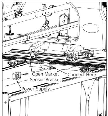
12-2 Plug the Power Supply into the Open Market Sensor Bracket.
