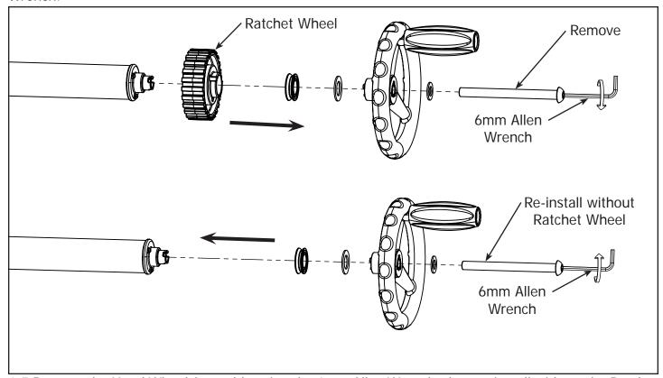
1-5 Remove the Hand Wheel Assembly using the 6mm Allen Wrench, then re-install without the Ratchet Wheel.
