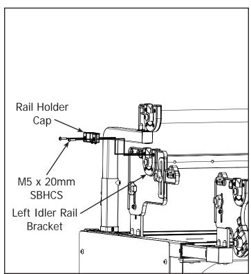
11-3 Install the Rail Tensioner Cap onto the Right 11-4 Install the Rail Holder Cap onto the Left Idler
