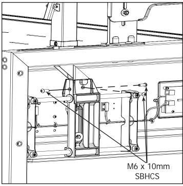
3-4 Secure the Take Up Rail Mount Assemblies into 3-5 Unused holes in the Take Up Rail Mounts should the Cam Slots using (3) M6 x 10mm SBHCS.
