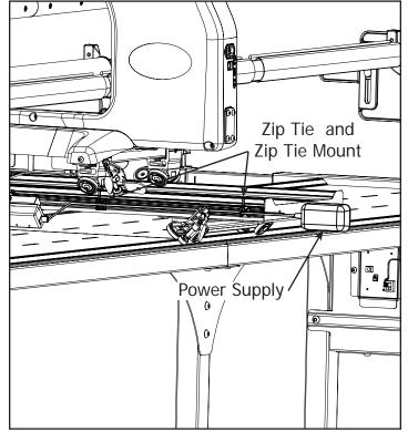
12-3 Secure cable with (2) Zip Ties and (2) Zip Tie Mounts. Plug in both Power Supplies into a power source.
