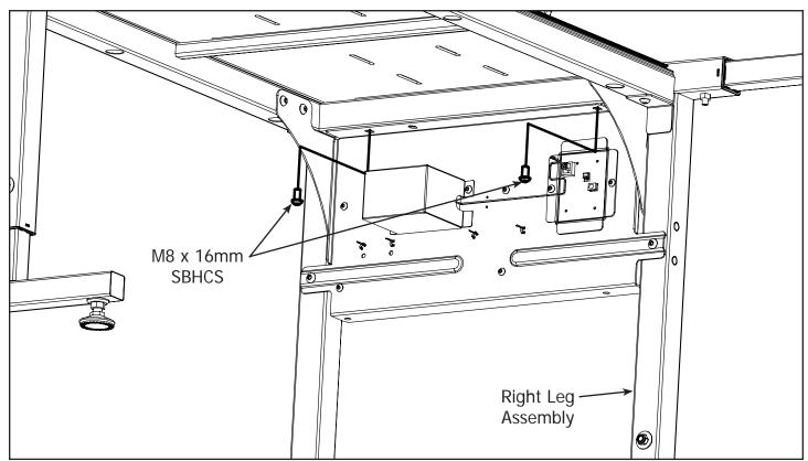
2-4 Secure the Right Motor Plate Assembly to the Right Leg using (2) M8 x 16mm SBHCS. **Note:** Tighten all screws at this time.
