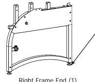
Leveling Foot (6) (Pre-installed on Frame Ends and Middle Lea) 03-10943
