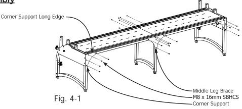
**4-1:** Align the Corner Supports so that the long edge follows the table surface and fasten with M8 x 16mm SBHCS. The Corner Supports should lay flush with the Table Assembly and Frame End surfaces. (Fig. 4-1)
