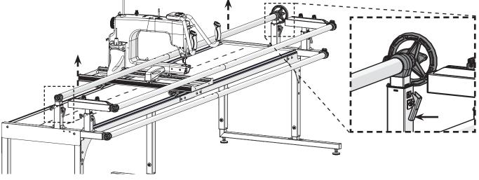
10 The mount holding the idler rail is installed on two of the 3 holes on the take-up rail arm. Choose whether to install the mount on the top two or bottom two holes by considering the size of your machine.
