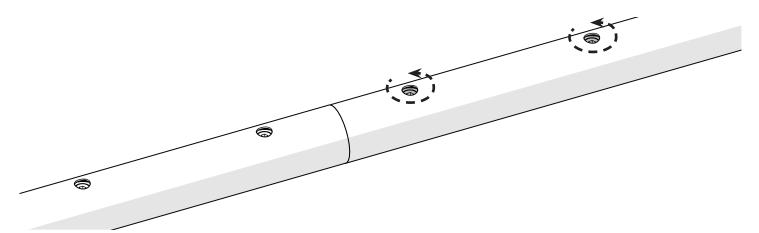
Loosen the 3-armed knobs on the take up rail arms on both sides of the frame. 5
