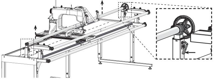
7 The mount holding the idler rail is installed on two of the 3 holes on the take-up rail arm. Choose whether to install the mount on the top two or bottom two holes by considering the size of your machine.
