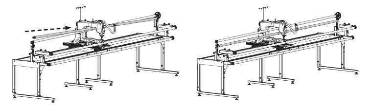
15 Push in on the mount and install the **3-armed knob**. To remove the frame in the future, simply loosen the **3-armed knob** and lift the rail out of the mounts.
