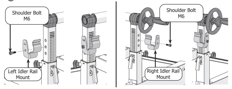
Pass the idler rail through the throat of the machine and place each end into the mounts.
