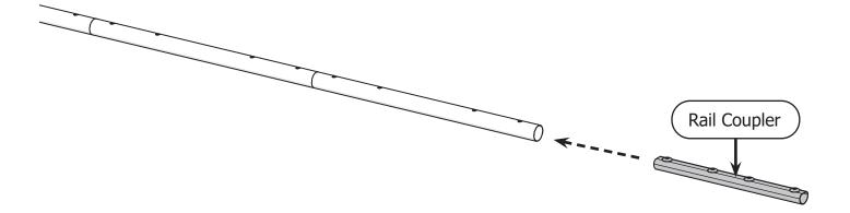
9 Install the remaining **non-ratcheting rail section** onto the other side of the rail coupler. Use the 4 mm Allen wrench to turn the coupler screws counter-clockwise.
