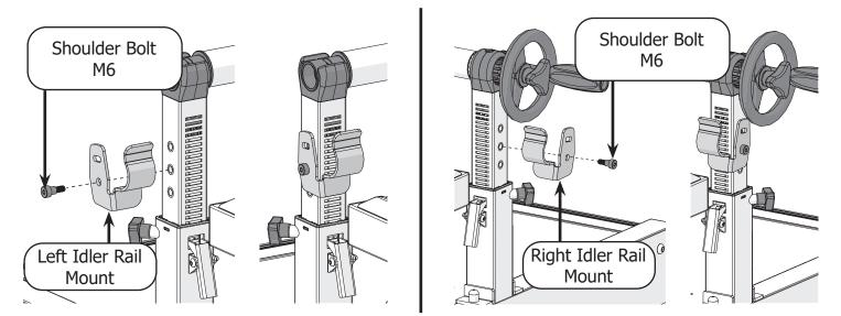
Pass the idler rail through the throat of the machine and place each end into the mounts.
