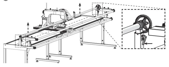
12 The mount holding the idler rail is installed on two of the 3 holes on the take-up rail arm. Choose whether to install the mount on the top two or bottom two holes by considering the size of your machine.
