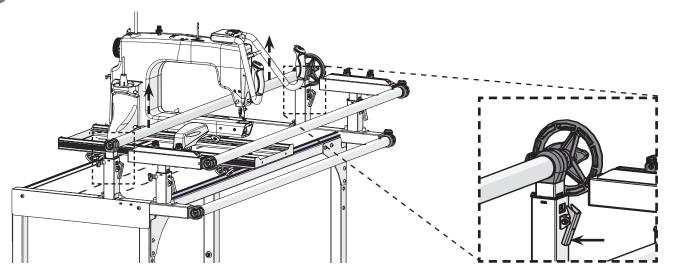
5 The mount holding the idler rail is installed on two of the 3 holes on the take-up rail arm. Choose whether to install the mount on the top two or bottom two holes by considering the size of your machine.
