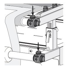
Re-install the idler rail into the idler mounts, over the top of the fabric.
