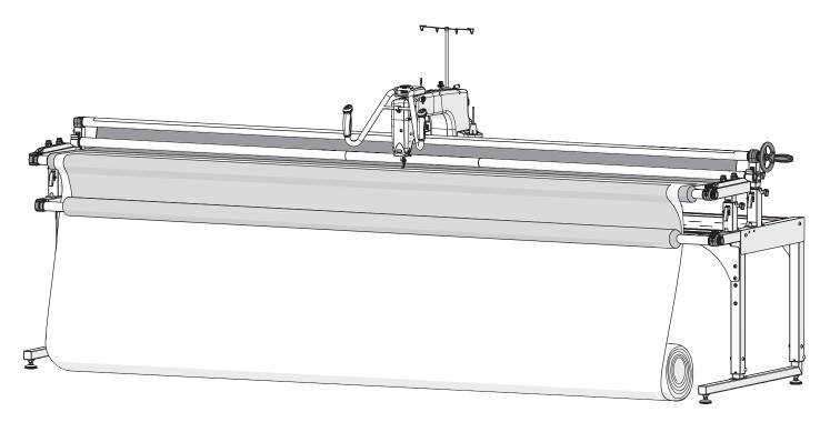
Check your rail height to make sure there is a finger's width of space between the idler rail and the floor of the machine. See "Setting the Rail Height" on page 29 for detailed instructions.
