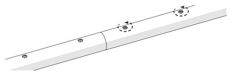
5 Now insert a second coupler into the 2 ft rail section.
