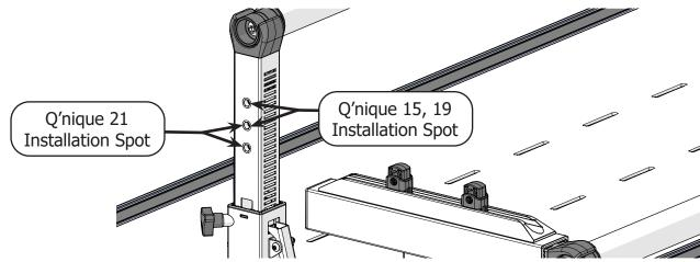
**11** Use the **shoulder bolt** and 4 mm Allen wrench to screw the **idler rail mounts** to each arm.
