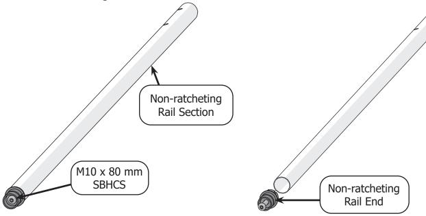
Use the 6 mm Allen wrench to screw the **non-ratcheting rail ends** to the free ends of one of the **5 foot rail segments** from your base frame.
