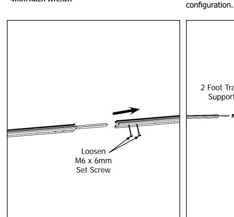
5-2 Remove one side of the Track Support from 5-3 Assemble Track Support Making sure there is your current configuration.
