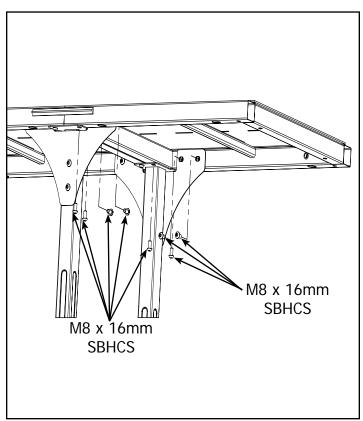
2-3 Secure using the (8) screws from step 1-4. **Note:** Leave all bolts loose until step 4.
