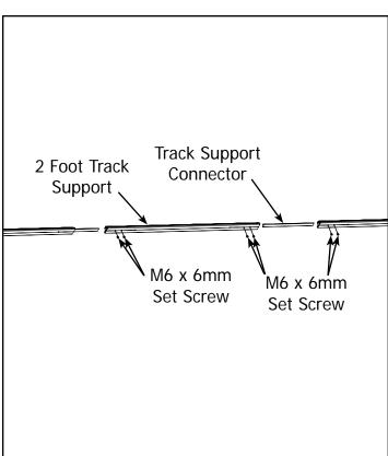
no gap between the Track Support Extrusions.
