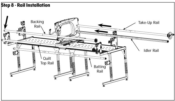
8-1 Install extended rail assemblies into position.
