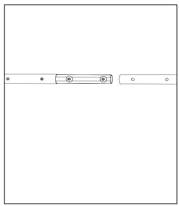
1-7 Remove one side of each rail assembly.
