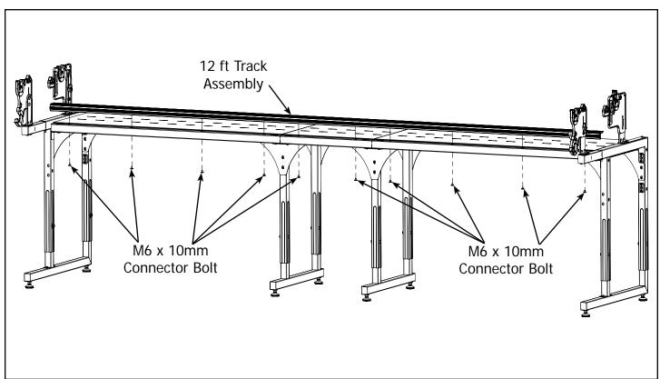
6-1 Install front Track Assembly using (10) M6 x 10mm Connector Bolts.
