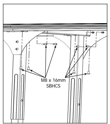
1-4 Remove (8) Center Leg screws and set aside.
