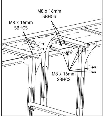
4-1 Position Middle Leg Braces and secure with (12) M8 x 16mm SBHCS.
