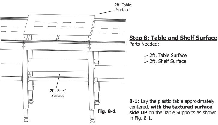
**8-2:** Attach the Shelf Table, **with the textured surface side UP** to the Shelf Supports with the pre-installed double sided tape, as shown in Fig. 8-1.
