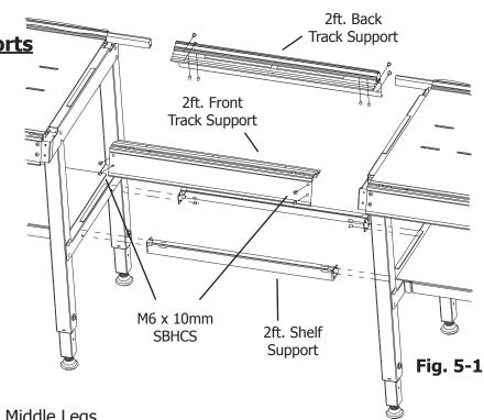
**6-2:** Take (2) 2ft. Shelf Support and attach them to the Middle Legs using (8) M6 X 10mm SBHCS, as shown in Fig. 5-1.
