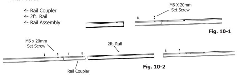
**10-1:** Pull Rail Assembly apart by removing (2) M6 X 20mm Set Screws from left side of Rail Assembly, as shown in Fig. 10-1.
