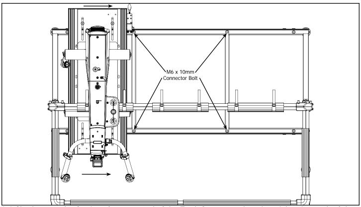
2-2 Slowly move the Carriage from one end of the Track Support to the other, tightening each of the (4) M6 x 10mm Connector Bolts as you go.
