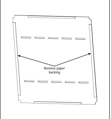
3-3 Remove the paper backing from the double faced tape on the Plastic Table Surface Center Section.
