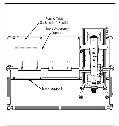
3-2 Align the Plastic Table Surface Left Section with the center of the Table Accessory Support making sure the edge of the Plastic Table Surface is parallel with the Track Supports.
