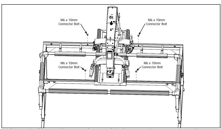
1-2 Remove the (4) center M6 x 10mm Connector Bolts from the track support and set aside.
