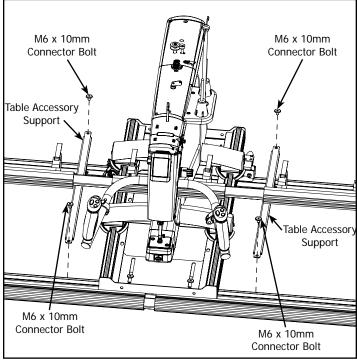
2-1 Install the (2) Table Accessory Supports using the (4) M6 x 10mm Connector Bolts from Step 1-2.
