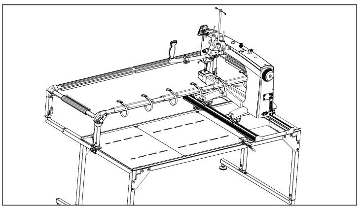
3-8 Press down on all edges of the Plastic Table Surfaces to make sure the double faced tape is secure.
