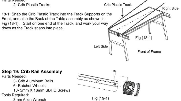
19-1: Attach a Ratchet Wheel to one end of each rail with a 5mm X 16mm SBHC Screw, as show in Fig. (19-1). (Slide the Ratchet Wheel onto the Rail until you can see the entire hole in the nut); repeat this for all three (3) sides of the Ratchet Wheel on both ends of the rail. Follow above steps to complete the other Rails. Now return to page 9, step 7.
