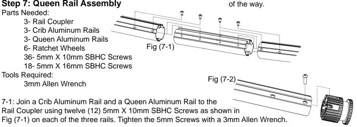
7-2: Attach a Ratchet Wheel to one end of each rail with a 5mm X 16mm SBHC Screw, as show in Fig. (7-2).( Slide the Ratchet Wheel onto the Rail until you can see the entire nut in the hole); repeat this for all three (3) sides of the Ratchet Wheel on both ends of the rail. Follow the same method to complete the other Rails.
