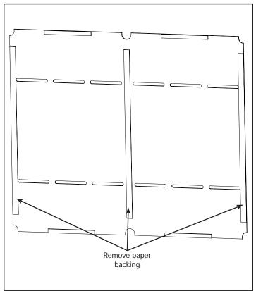
3-4 Remove the paper backing from the double faced tape on (1) of the Plastic Table Surface Section 2.
