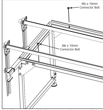
2-1 Remove the (2) M6 x 10mm Connector Bolts from the far left end of the frame and set aside.
