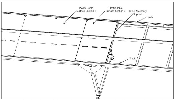
3-7 Position the Plastic Table Surface Section 3 against the Plastic Table Surface Section 2 making sure the edge of the Plastic Table Surface is parallel with the Track Supports.
