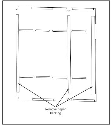
3-11 Remove the paper backing from the double faced tape on the Plastic Table Surface Section 4.
