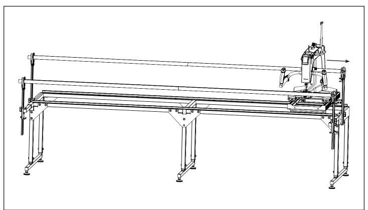
3-2 Move the Carriage to the far right side of the frame and secure with the Channel Lock.
