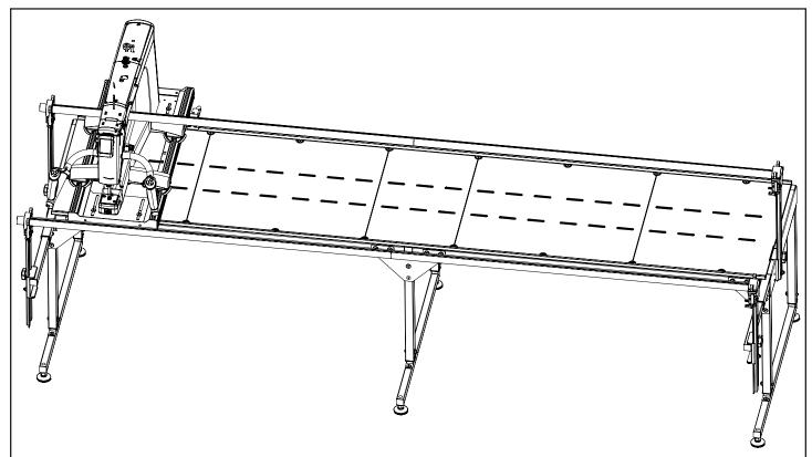
3-13 Press down on all edges of the Plastic Table Surfaces to make sure the double faced tape is secure.
