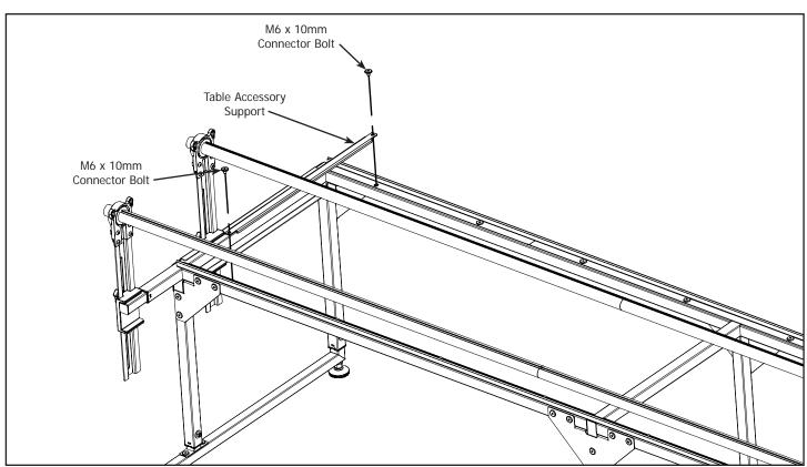
2-2 Using the (2) M6 x 10mm Connector Bolts from Step 2-1 install (1) Table Accessory Support.
