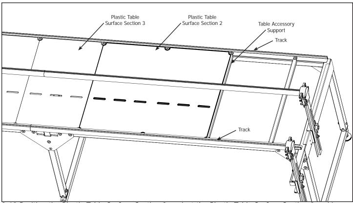
3-10 Position the Plastic Table Surface Section 2 against the Plastic Table Surface Section 3 making sure the edge of the Plastic Table Surface is parallel with the Track Supports.
