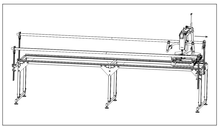
1-2 Move the Carriage to the far right side of the frame and secure with the Channel Lock.
