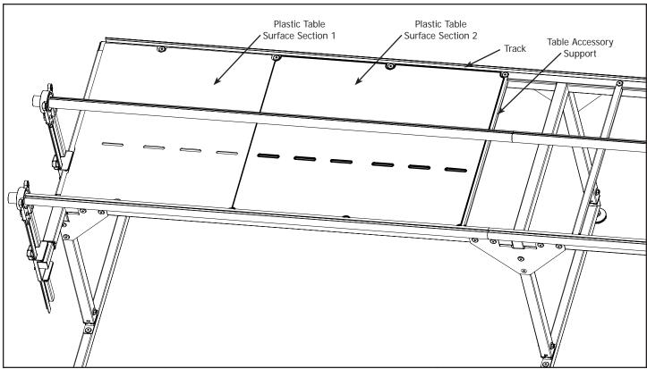
3-5 Position the Plastic Table Surface Section 2 against the Plastic Table Surface Section 1 making sure the edge of the Plastic Table Surface is parallel with the Track Supports.
