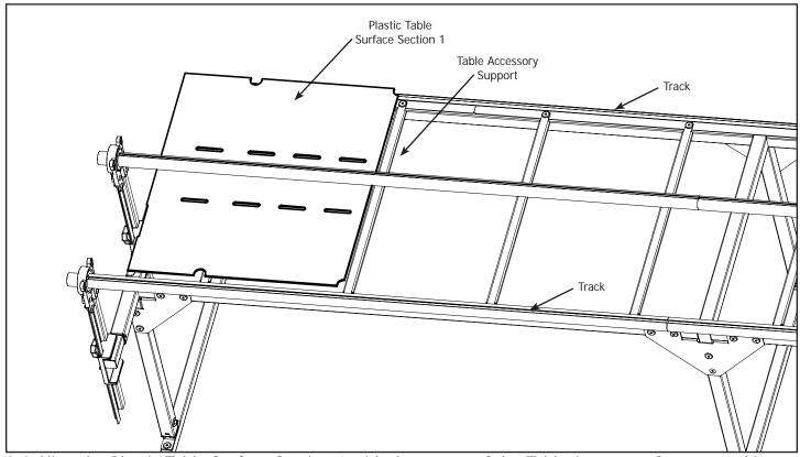
3-3 Align the Plastic Table Surface Section 1 with the center of the Table Accessory Support making sure the edge of the Plastic Table Surface is parallel with the Track Supports.
