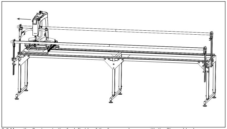
2-3 Move the Carriage to the far left side of the frame and secure with the Channel Lock.
