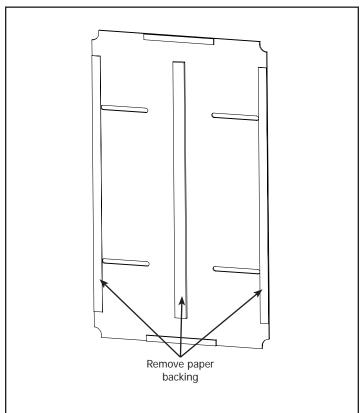
3-6 Remove the paper backing from the double faced tape on the Plastic Table Surface Section 3.
