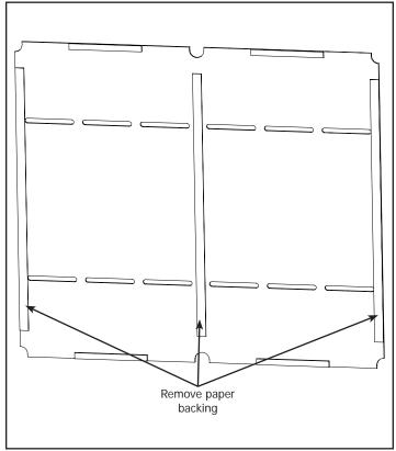
3-9 Remove the paper backing from the double faced tape on (1) of the Plastic Table Surface Section 2.
