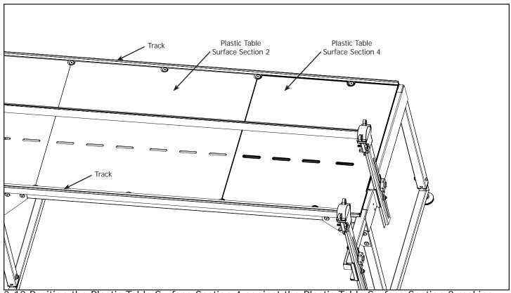
3-12 Position the Plastic Table Surface Section 4 against the Plastic Table Surface Section 2 making sure the edge of the Plastic Table Surface is parallel with the Track Supports.
