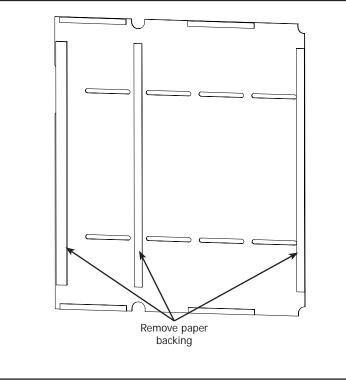
3-1 Remove the paper backing from the double faced tape on the Plastic Table Surface Section 1.
