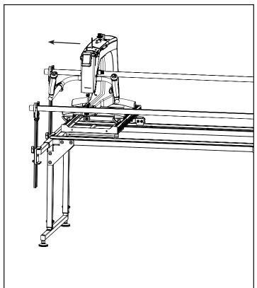
3-8 Move the Carriage to the far left side of the frame and secure with the Channel Lock.
