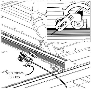
9-11 Remove Back Left Wheel and Screw from Bottom Plate
