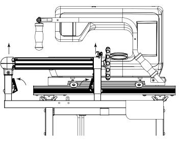
6-4 Insert Back Rail through the throat of the Sewing Machine
