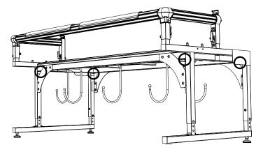
3-9 Tighten (16) loose screws on the Coner Braces from Step 1-7
