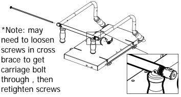
4-4 Place Bottom Plate onto Frame and Top Plate onto Bottom Plate
