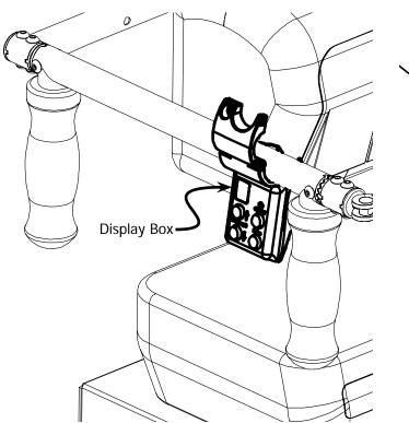
9-3 Secure the Display Box with (1) M4 x 16mm SBHCS
