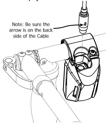
9-7 Plug in the other end of the Display Cable into the Control Box
