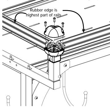
3-7 Tighten each bolt with the Allen Wrench oriented verticle as shown in Fig. **3-7a until difficult to turn, then turn each** bolt 1/4 rotation with the Allen Wrench oriented horizontal as shown in Fig. 3-7b. 3-8 Tighten the (4) loose screws on the underside of the table from Step 1-5
