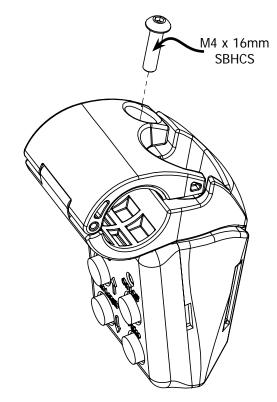
9-2 Clamp Display Box onto Crossbar next to the Handle on the Left or Right Side
