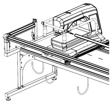
6-5 Insert the left end of the Back Rail into the left back Rail Holder
