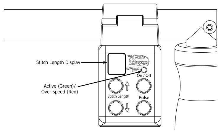
**Note:** When the SureStitch is in the "on" mode, the sewing machine WILL BEGIN TO STITCH! When you stop moving the machine, it will continue to stitch at the sewing machine's minimum speed until you press the off button. This feature ensures the machine will maintain as consistent a stitch length as possible with the intial movement of the machine.
