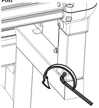
6-3 Loosen each Knob on the back of each Rail Holder
