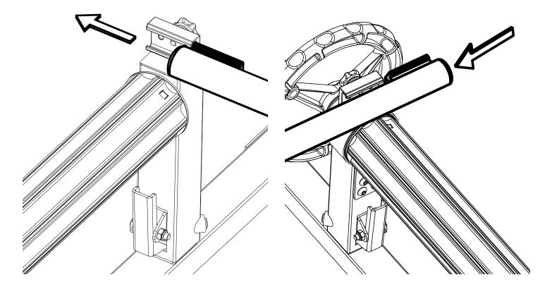
6-7 Tighten each Knob on the back of each Rail Holder
