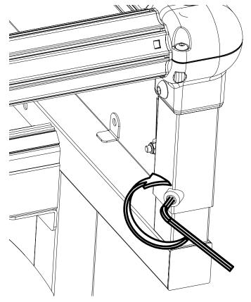
7-3 Move the Sewing Machine so that the Needle is 1" away from the Back Rail. Hold the Machine in place as you adjust the Carriage Stop by loosening the knob and sliding the Sewing Machine stop against the back wheel. This will be adjusted again in the Fabric Installation instructions.
