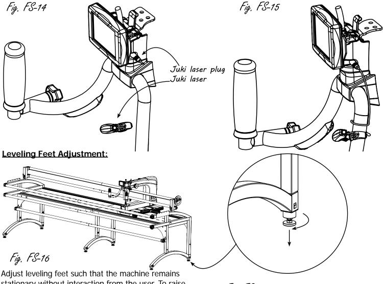
stationary without interaction from the user. To raise the leg of the machine simply turn the foot clock-wise shown in figure FS-17 and reverse action to lower the foot.
