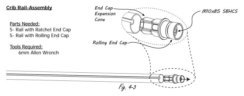
**4-1-C:** Using the 6mm Allen Wrench, loosen the M10 x 85mm SBHCS in the Rolling End Cap, but do not completely unthread it. Loosen the bolt until it protrudes just beyond the Rolling End Cap. Hold the rail vertically with the rolling end cap down and tap the protruding bolt head on the floor. This will free the compressed end cap from the rail. Then remove the Rolling End Cap from the rail (Fig. 4-3).
