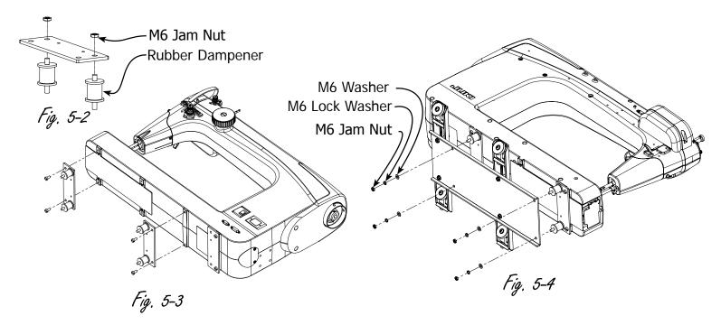
**<u>5-3</u>**: Re-install the 2 Mounting plates using a 5mm Allen Wrench. Be sure that the Rubber Dampener side of each plate is pointing towards the middle of the machine as show in Fig. 5-3.
