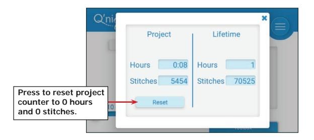
**Tip:** It's recommended to oil your machine after 20 hours of use. The "Hours Run" counter can help keep track of when your machine is due to be oiled. After cleaning and oiling your machine, press **Reset** to start the counters under **project** back at zero.
