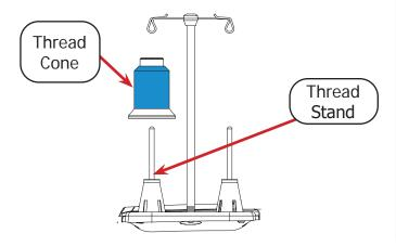
Pull the thread straight up, through the thread mast guide loop above the thread stand.
