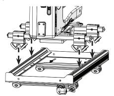
8 Place the **front wheel support assembly** under the front of the machine, with the **set screws** facing the rear. Loosen the set screws on one side with the 4 mm Allen wrench.
