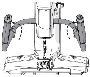
9 If desired, extend the handles outward to improve the reach of the machine.
