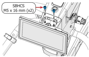
4 Tilt the display to the desired angle and use the 3 mm Allen wrench to tighten down the M5 x 8 mm SBHCS to secure it in place.
