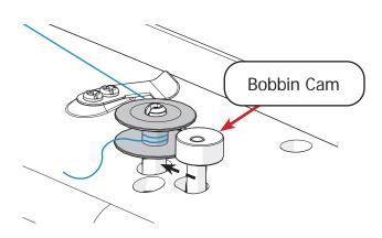
5 Winding stops automatically when the bobbin is full. Cut the thread with the **thread cutter** near the bobbin cam.
