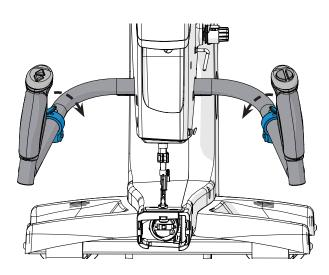
**Tip:** For micro-stippling, angle the handlebars down toward the needle plate in step 4, and leave the controls horizontal in step 7.
