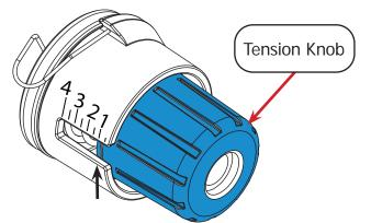
**Note:** Setting "1" is the lowest tension for your machine, and is an ideal starting place to find the correct top tension. Do not over loosen: the tension knob may unscrew and fall off.
