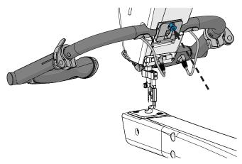
5 Hold the handlebars at the desired angle and tighten the clamp screw.
