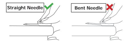
To avoid damage to the machine, please choose an approved needle style from the list below:
