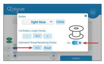
The **bobbin estimator symbol** will also show on the left side of the quilting mode screen when the estimator is on. Color changes notify when the bobbin is estimated to be nearing the end of the thread.
