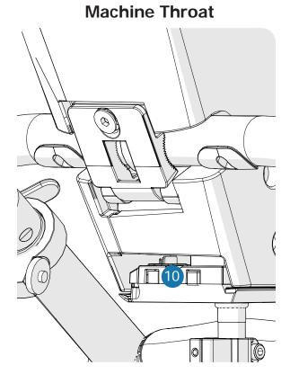
**10** Handlebar Ports (page 15) Connects handlebar controls to machine.
