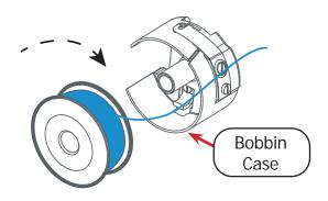
5 Slip a few inches of thread through the slot and out of the **hole**.
