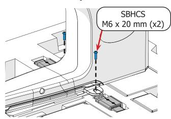
6 Use the L-shaped 4 mm Allen wrench and the two **M6 shoulder bolts** to attach the front wheel assembly to the machine.
