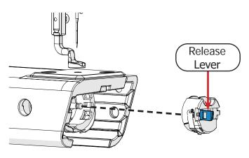
4 Place the wound bobbin into the **bobbin case**. Note the direction that the thread is coming off the bobbin in relation to the case.
