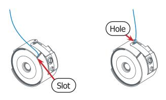
**Note:** If the bobbin is wound correctly it will turn clockwise when the thread is pulled.
