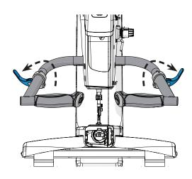
8 Twist the controls until they are comfortable to hold and operate.
