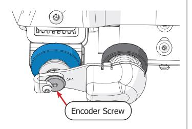
7 Turn the encoder lock collar (shown in blue) to point up and tighten the lock collar screw with the 2.5 mm Allen wrench.
