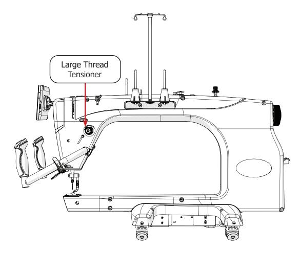
Loosen the tension knob on the large thread tensioner to set the tension to "1." The bottom of the tension knob will line up with the number that the tension is set to.
