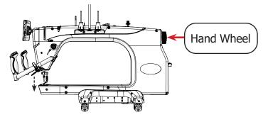
3 Use the 3 mm Allen wrench to remove the **hopping foot screw** and **the hopping foot**.
