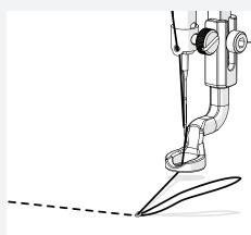
e Keep moving away from the tie-off until a loop of bobbin thread is pulled up above the fabric. Cut all threads close to the tie-off.
