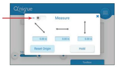
3 Move the machine so that the needle is at the position where you want to start your measurement and click the **Reset Origin** button. This origin will be saved until you reset it again.
