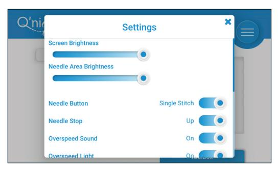
**Note:** The machine is unable to stitch while the Settings menu is pulled up.
