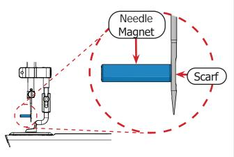
6 Use the needle magnet as a visual guide. Twist the needle until the **magnet** (shown in blue) points as straight out from the machine as possible. **Note:** Do not attempt to adjust the needle by moving the magnet directly.
