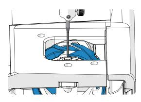
11 Slip the **timing spacer tool** (shown in blue) into the hook assembly with the flat side facing up. Then turn the timing tool until the flat side faces down.
