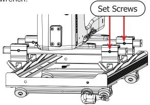
Slide the machine up and down the bottom carriage tracks several times so that the machine can settle and ride smoothly.
