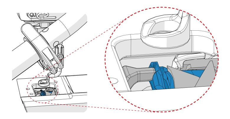
9 Tighten the hook holder screw to fasten the hook holder in place. The inside part of the hook assembly should no longer rotate freely by hand.
