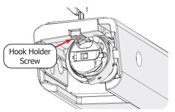
4 Remove the **hook holder** (shown in blue) from the hook assembly.
