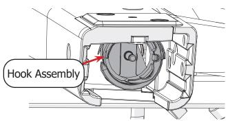
7 Rotate the **hand whee**l until the needle is halfway down. This will put the hook in the best position for oiling.
