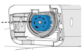
12 Turn the hand wheel the clockwise to bring the **needle** back down until it rests on top of the timing spacer. Do not let the needle rise to the top before bringing it back down or you will need to repeat steps 8-11.
