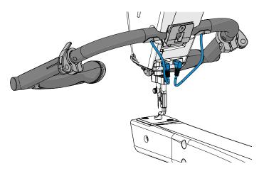
7 Open the **handlebar levers** (shown in blue).
