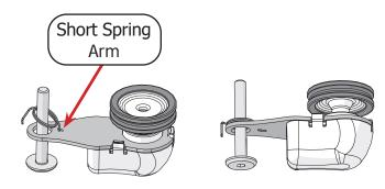
8 Place the long arm of the encoder spring arm into the hole on the encoder **lock** collar.
