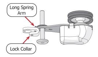
9 Without allowing the arm to slip out of the lock collar, rotate the collar until it wraps around the encoder bolt.
