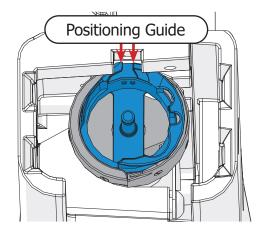
6 Slide the finger of the **hook holder** (shown in gray) into the middle of the hook assembly's positioning guide.
