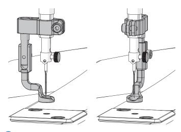
6 Lift the hopping foot collar back up to the press bar so that the bottom of the collar is even with the bottom of the press bar, and re-tighten the **collar screw**.
