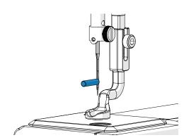
7 Hand-tighten the **needle thumb screw**. Do not over-tighten if using the flat-head screwdriver.
