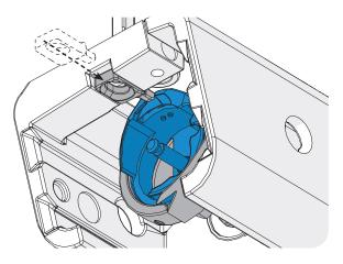
7 Attach loosely with the **hook holder screw**. Do not tighten.
