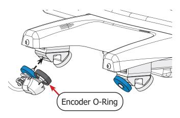
6 Tighten the **encoder screw** with the 4 mm Allen wrench.
