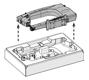
4 Place the machine on the wheels in level one of the packaging so that the holes in the **wheel mounts** align with the holes in the **front and back wheel assemblies**.
