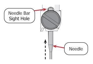
5 The **scarf**, a cut-out on the back of the needle, should face the throat of the machine. Place the **needle magnet** on the opposite side of the scarf.
