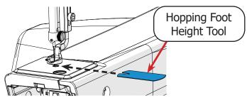
Note: The height tool prepares the machine for standard sized guilt batting and two layers of fabric. For thicker guilts, stack sheets of printing paper over the gauge to increase room underneath the hopping foot.
