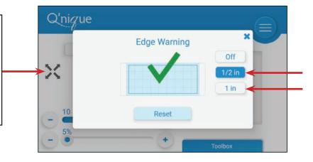
5 To return to the main quilting screen, press the X in the top right corner or press anywhere outside of the edge warning screen.
