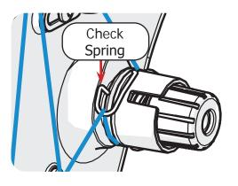
10 Next, pass the thread down and around the **thread guide** next to the large thread tensioner.
