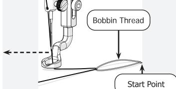
d Pull on the loop of **bobbin thread** until the loose end of the thread comes up from underneath the fabric.
