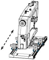
10 Use the 4 mm Allen wrench to re-tighten the wheel assembly **set screws** you loosened earlier.
