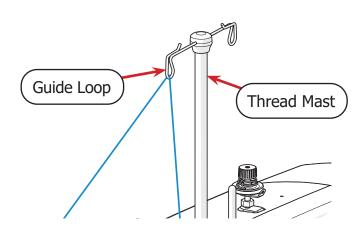
5 Feed the thread through the top hole of the **thread guide rod**. Wrap the thread around to the back of the guide and insert through the bottom hole.
