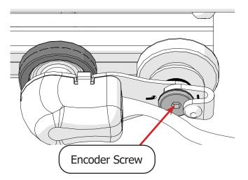
8 Turn the encoder **lock collar** (shown in blue) to point up. Then tighten the **lock collar screw** with the 2.5 mm Allen wrench.
