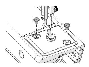
5 Turn the inside part of the **hook assembly** (shown in blue) so that the **positioning guide** is at the highest point.
