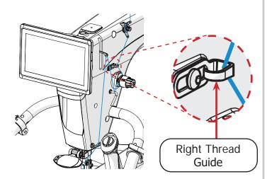
8 Pull the thread around the **large thread tensioner**, between the tension discs.
