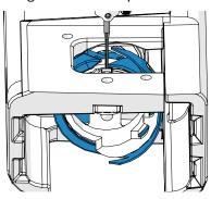
10 Stop raising the needle once the eye is about level with the **hook** (shown in blue). Do not continue to raise the needle. If the needle goes too high, start over at step 9.
