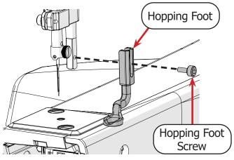
With the 3 mm Allen wrench, loosen the collar screw that holds the hopping foot collar to the press bar.
