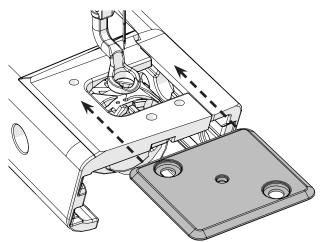
3 Align the screw holes on the needle plate with those on the machine.
