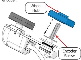
6 Place the encoder screw into the left rear wheel hole on the carriage so the **O-ring** is between the rear wheels.
