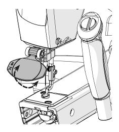
7 You can change the lens by lifting the lens out of the right angle mount and replacing it with a different magnification.
