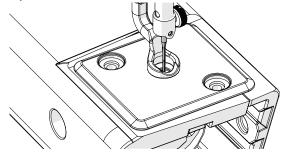
5 Place the two **needle plate screws** (shown in gray) into the plate. Make sure the needle plate is centered around the needle, and then tighten the screws with the flat-head screwdriver.
