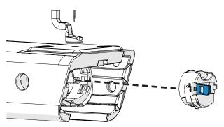
5 Take the bobbin from the case and set it aside. Clean the bobbin case with the lint brush or compressed air. Be sure to clean the area under the **bobbin tension thread arm**.
