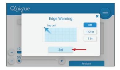
Tip: You can also use the start/stop guilting button on the right handlebar to set the corners of the "safe area."
