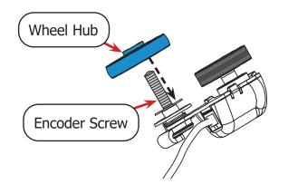
5 Place the encoder screw into the left rear wheel hole so the **encoder O-ring** is between the two left machine wheels.
