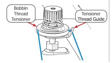
4 Tightly wrap the thread clockwise around the bobbin a few times to hold the thread in place. Push the **bobbin cam** toward the bobbin to start winding.
