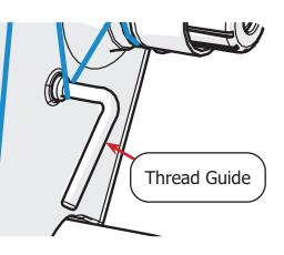
11 Pull the thread through the hole in the **take-up lever**.
