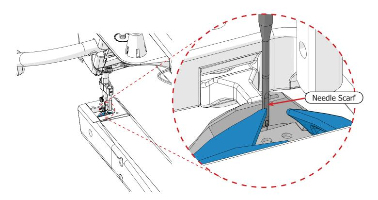
14 Pull the hook assembly toward the front of the machine until the hook is as close to the needle as possible without touching.
