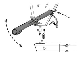
6 Plug the cables from the handlebars into the machine.
