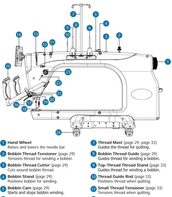
6 **Bobbin Wind Thread Stand** (page 29) Holds a cone of thread.
