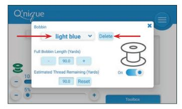
6 To return to the main quilting screen, press the **X** in the top right corner or press anywhere outside of the bobbin estimator screen.
