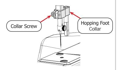
5 Drop the hopping foot collar below the **press bar** and turn it to the desired position.
