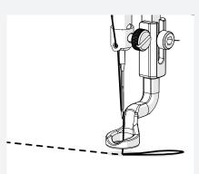
d Hold the loop and move the machine away from the tie-off again.
