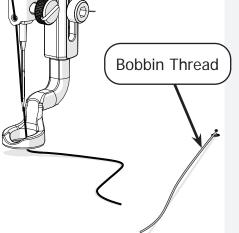
e Pull on the bobbin thread while moving the machine back to the start point. This makes sure that there is no loose thread underneath the fabric.
