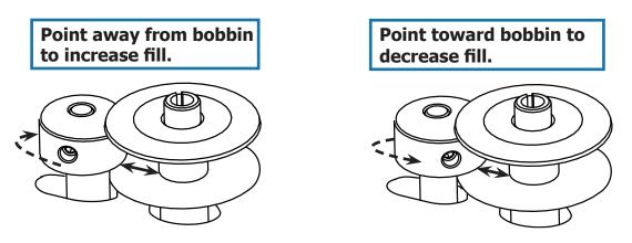
5 After choosing the desired distance, tighten the set screw with a 1.5 mm Allen wrench.
