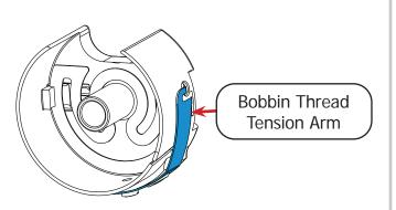
6 In and around the **hook assembly**, clear away any lint, cloth, and thread remnants using the lint brush or compressed air.
