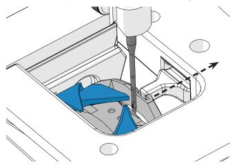
15 Use the 2 mm Allen wrench to tighten one of the three **set screws** through the timing cut-out window on the left.
