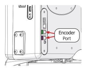
4 Use the 4mm Allen wrench to loosen the **encoder screw** and remove the encoder and wheel.
