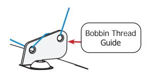
3 Pull the thread through the hole in the **tensioner thread guide** and then around the back of the **bobbin thread tensioner**, between the two discs.
