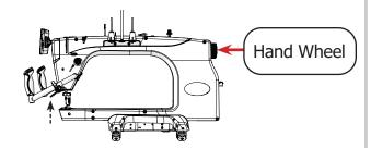
3 Use the 3 mm Allen wrench to remove the hopping foot screw and the hopping foot.
