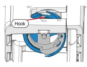
9 Hold the Hook Assembly and carefully rotate the hand wheel counter-clockwise to drop the **needle** (shown in gray) to its lowest point. Continue rotating the hand wheel the same direction. The needle should begin to raise up.
