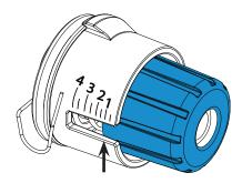
• If the top thread is pulled down through the bottom layer of fabric, there is too little top tension. Increase the tension on the top by slowly turning the large thread tensioner knob toward setting "4." Stop turning the knob when desired tension is achieved.
