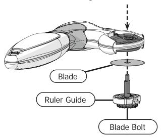
3 Reinstall the bolt and ruler guide with a **new** or sharpened blade.
