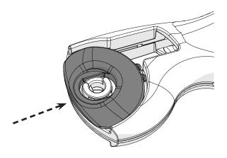
6 Reinstall the safety guard on the right side of the cutter by inserting it at an angle and then pulling it out.
