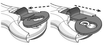
Reinstall the bolt, blade, and ruler guide so that they are on the right side of the cutter.
