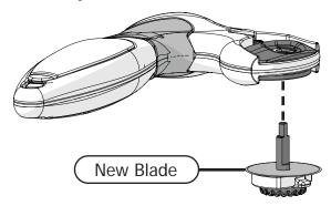
4 Reinstall the plastic nut, spring, and plastic washer.
