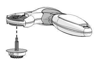
8 Reinstall the nut, spring, and washer so that they are on the left side of the cutter and tighten to hold in place.
