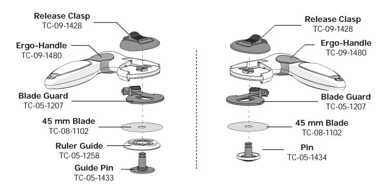
**Shown:** Right-handed setup using ruler guide.
