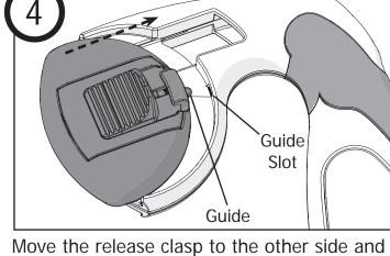
Move the release clasp to the other side and push the **guide** into the **guide slot**.
