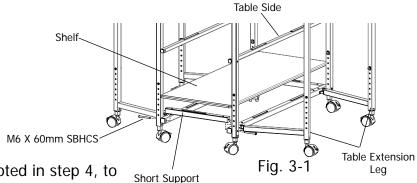
**Note:** Do not tighten SBHCS screws until noted in step 4, to help prevent the table from getting out of square.
