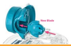
**4.** Remove the blade cover by twisting a little and pulling. Keep it in a safe place.
