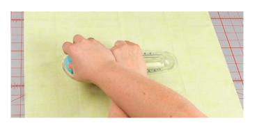
**3.** Apply pressure to the blade and sizing knobs, and in one smooth motion, rotate the blade knob in a full circle.
