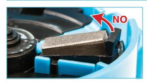
Make sure the stones are placed all the way down in their holders. If part of the stone is raised, or not all the way in, it will not sharpen your blade.
