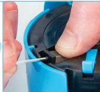
4. Gently tighten the screw. Hold down the stone during tightening or it will raise up. Overtightening the screw may cause stones to sit incorrectly.
