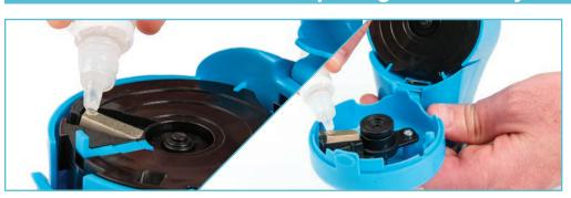
1. Make sure the sharpener is plugged in. Apply one drop of oil to both the top stone and the bottom stone. Add an additional drop of oil for every 60 seconds of sharpening.
