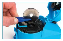
**5.** Open the sharpener, lift the blade with the blade lever, and flip the blade over with the included blade handlers.
