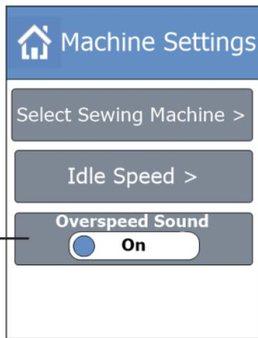
If you move the machine too quickly across the frame, the machine motor won't be able to stitch quickly enough to maintain stitch regulation. The overspeed sound lets you know that you are moving too fast.
