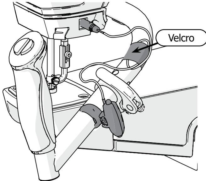
**If the laser is mounted on the laser bracket and plugged into the back of the machine, attach the velcro to the back handles.**
