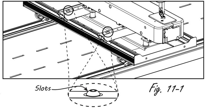
**11-2: Align Front Track** Slowly roll the Carriage from one end of the Quilting Frame to the other several times. This will adjust the Track so that it is centered under the Front Wheels and parallel to one another. Once adjusted, move the sewing machine to one end of the frame and using the 4mm Allen Wrench, tighten each of the (8) M6 x 12mm Connector Bolts as you roll the machine above each one.
