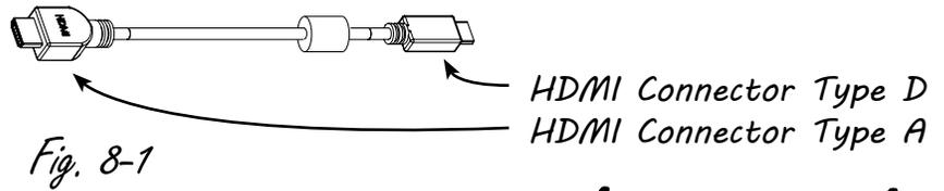
**8-1:** Take the HDMI cable end (HDMI connector Type A see figure 8-1) and plug it into the front handles. Pass the cable through the LCD from the bottom (Fig. 8-2).
