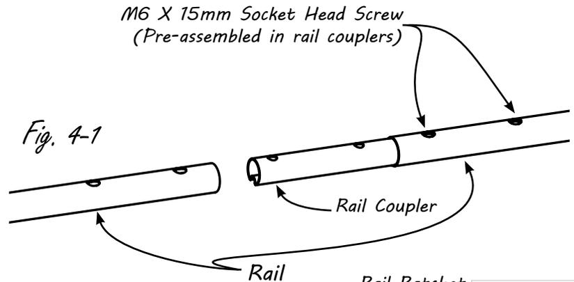
**4-1:** Slide a Rail Coupler into a Rail with Ratchet End Cap. Align the holes on the Rail with the holes in the Rail Coupler. Tighten the (2) pre-installed M6 X 15mm Socket Head Screws using the 4mm Allen Wrench. (Locations shown in Fig. 4-1.)
