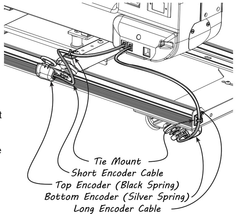
**10-10:** Test front to back Carriage travel to make sure that the Encoder Cables allow the full range of Carriage movement, as well as staying off of the Table Surface, and the Plastic Tracks.
