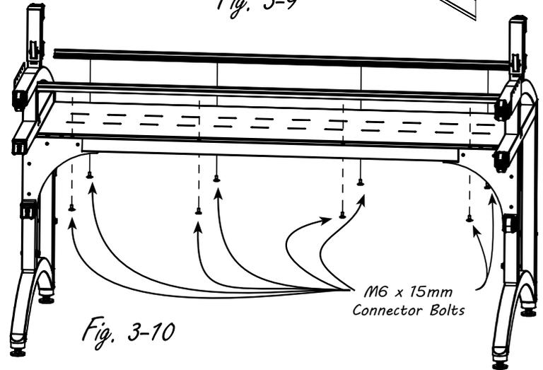
**3-5-C:** Now attach a Track Support to the front of the Table Structure, but this time leave the Bolts a turn loose (Fig. 3-10). You will adjust and secure the width of this Track Support in step 11.
