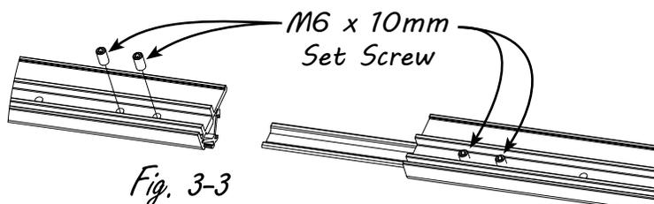
**3-5:** Insert the exposed end of the Track Support Coupler into the end of an unused Track Support.
