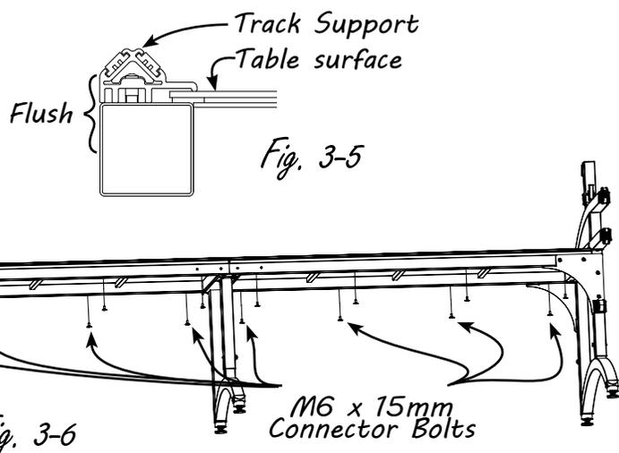
**3-9:** Now attach a Track Support to the front of the Table Structure, but this time leave the Bolts a turn loose. You will adjust and secure the width of this Track Support in step 11.
