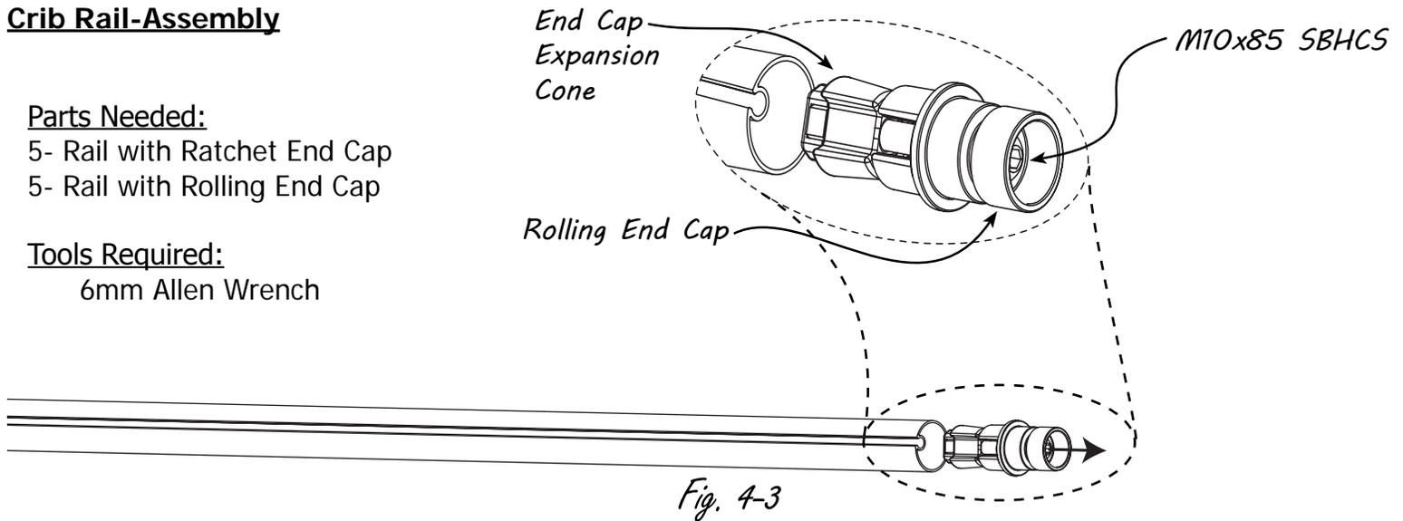
**4-1-C:** Using the 6mm Allen Wrench, loosen the M10 x 85mm SBHCS in the Rolling End Cap, but do not completely unthread it. Loosen the bolt until it protrudes just beyond the Rolling End Cap. Hold the rail vertically with the rolling end cap down and tap the protruding bolt head on the floor. This will free the compressed end cap from the rail. Then remove the Rolling End Cap from the rail (Fig. 4-3).
