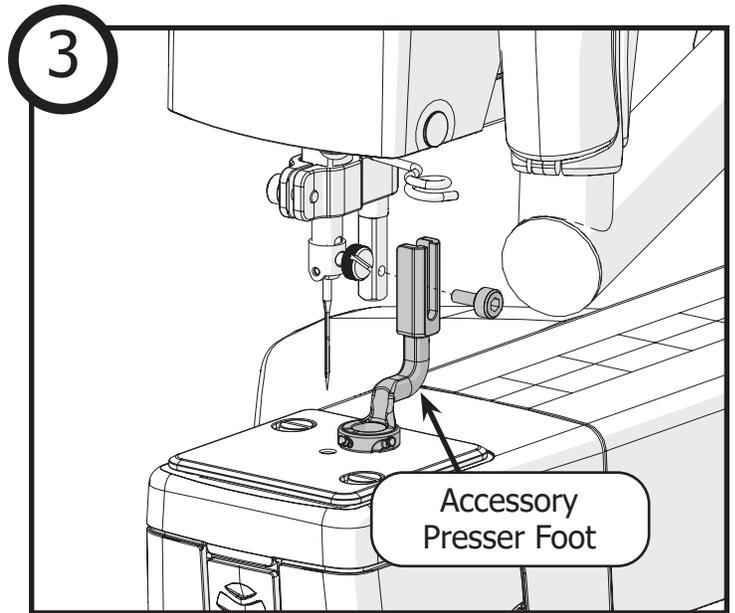
Place the **accessory presser foot** onto the collar bar with a hopping foot screw. Leave extra room under the bottom of the hopping foot for the attachments.
