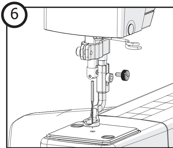
Reinstall your machine's needle and needle thumb screw.
