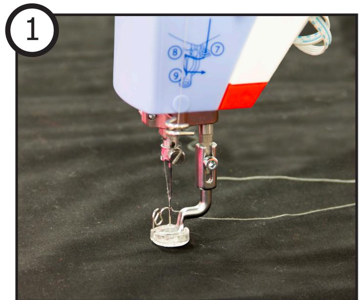
When you are ready to begin quilting with yarn or specialty thread and the couching foot has been installed, needle up and down one time.
