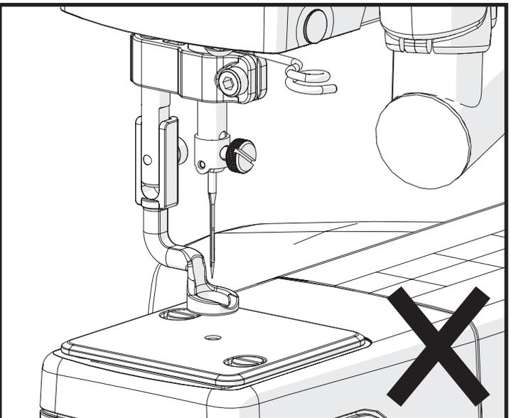
Check the position of your hopping foot. The couching attachment can only be used if the hopping foot is set directly behind the needle. See your machine manual for instructions on changing the hopping foot orientation.
