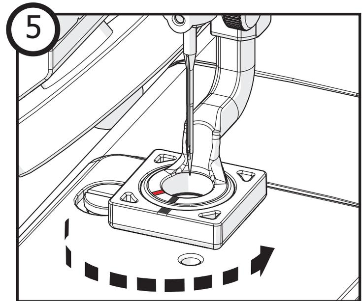
Twist the foot until the black mark aligns with the black mark and it is locked into place.
