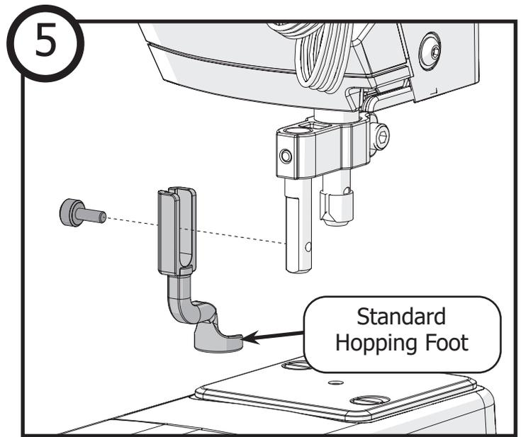
Place the upgraded **standard hopping foot** onto the hopping foot collar bar. Attach with a hopping foot screw loosely enough that the hopping foot can slide up and down.
