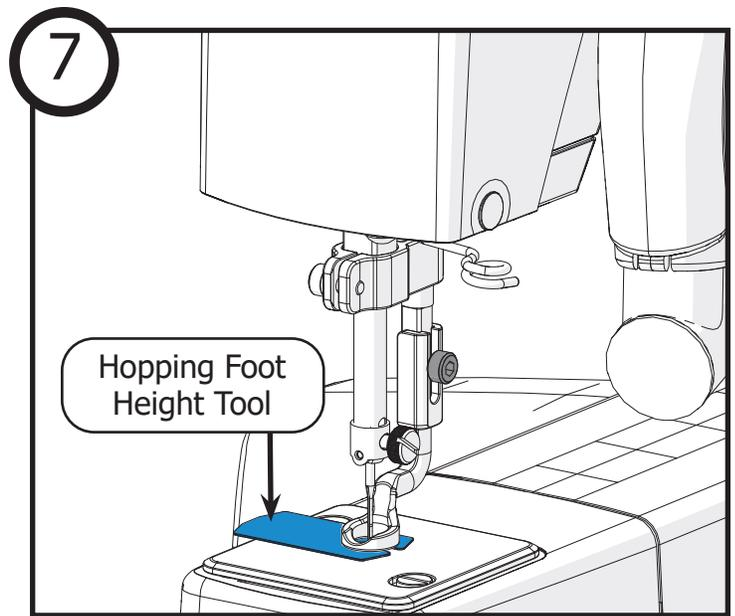
Set hopping foot height: move the machine off of the fabric and drop the needle to the lowest position. Slide the the **hopping foot height tool** beneath the foot. Tighten the hopping foot screw with the 3 mm Allen wrench.
