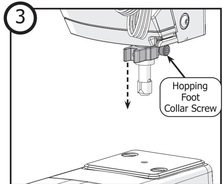
Loosen the **collar screw** with a 3 mm Allen wrench just enough that hopping foot collar can be pulled down off the machine.
