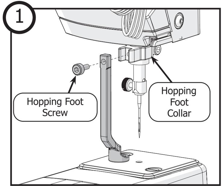
Use a 3 mm Allen wrench to remove the **screw** attaching the hopping foot to the **hopping foot collar** on your machine.
