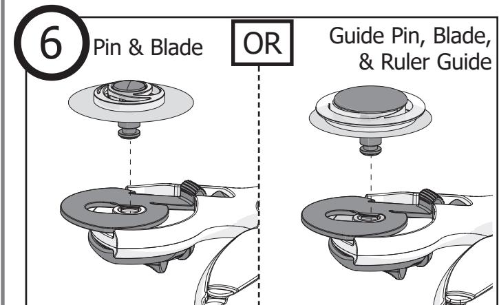
Re-install the blade and pin, or blade, ruler guide, and guide pin.
