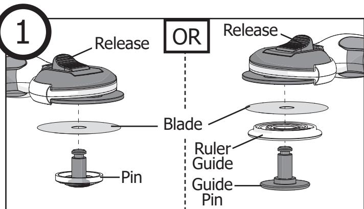
Extend the blade guard and pull in the **release** to drop the **blade** and **pin**.
