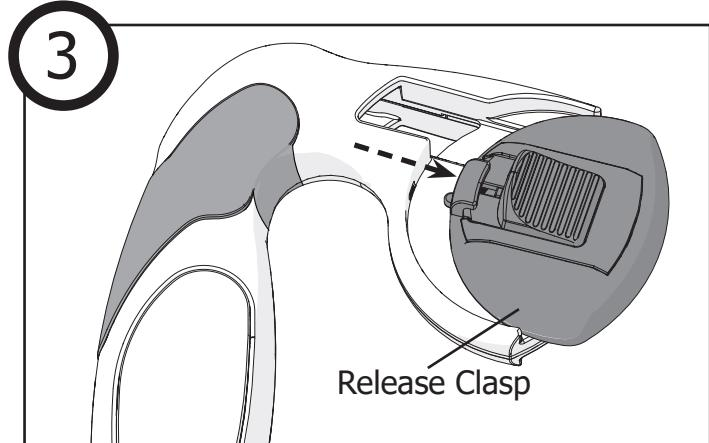
Push out on the blade release to detach the **release clasp** from the handle.
