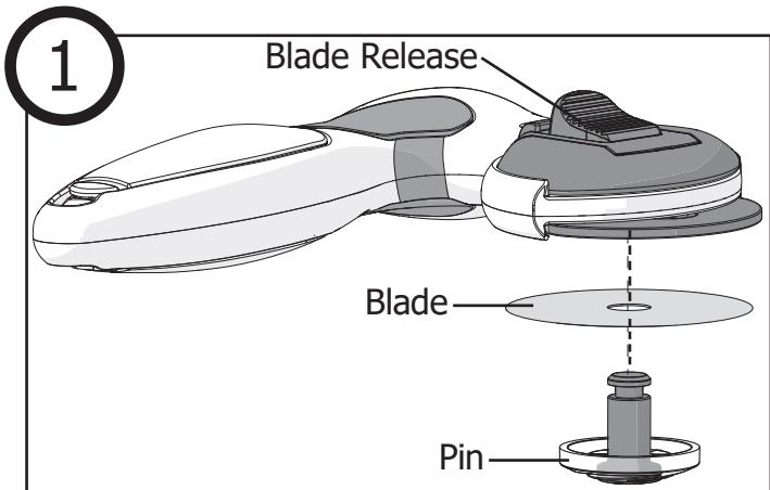
Pull in the **release** to drop the **blade** and **pin** from the cutter.
