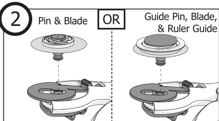
Place the new blade onto the **pin**, and press into the handle until it clicks.
