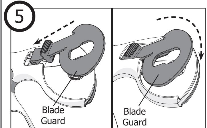
Flip over the handle. Insert the lever part of the **blade guard** into the handle. Lay it flat and extend the guard to lock it in place.
