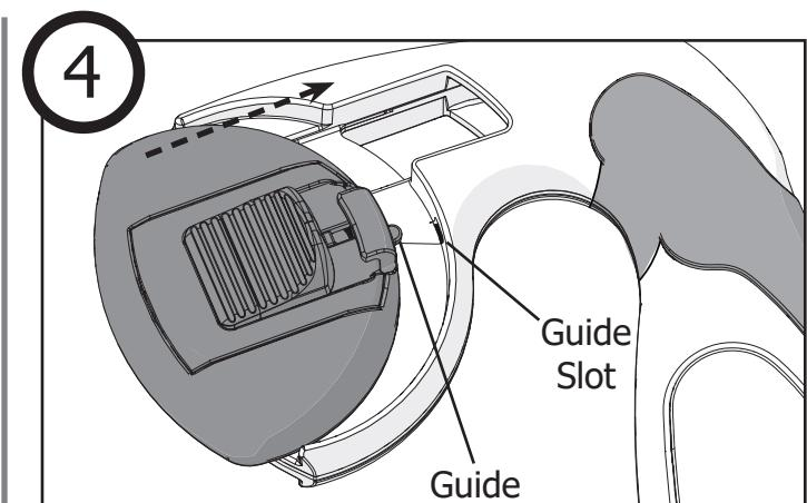
Move the release clasp to the other side and push the **guide** into the **guide slot**.
