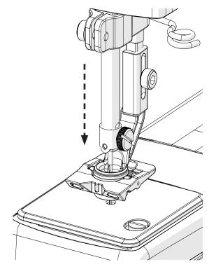
4 Slide the **Hopping Foot Height Tool** beneath the foot. Lower the foot until it rests on height tool. Tighten the M3 x 8 mm SBHCS with the 3 mm Allen wrench.
