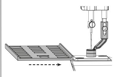
2 Hold the ruler against the foot to stitch straight lines and to measure stitch length. The swivel system allows you to slide the ruler along the foot and measure stitches in any direction.
