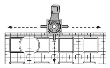
Press the lip side of the ruler to the front of the hopping foot. The ruler should align with the pointers on the hopping foot at right angles.
