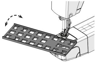
To release the ruler, press down on the back of the clip behind the foot and pull the ruler away from the foot.
