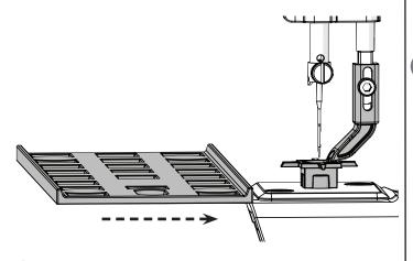
2 Hold the ruler against the foot to stitch straight lines and to measure stitch length. The swivel system allows you to turn the ruler to measure stitches in any direction.
