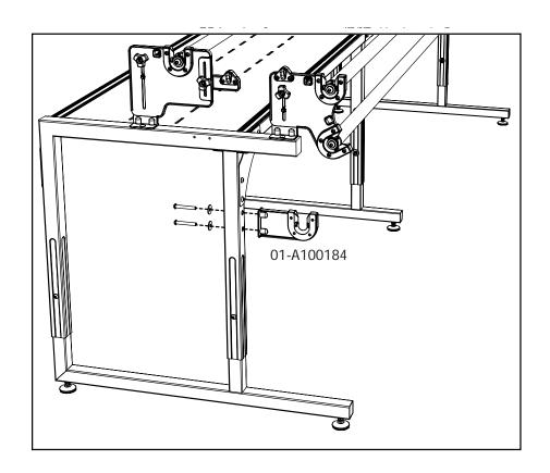
**Geared Rail Assembly** 2 01-A100181 A 04-11005 01-A100175 04-11005 01-A100182 B 04-11005 \*INS-LP008 03-10167 03-10167 Note: Leave the connector bolts attached to the coupler and unscrew the connector bolt inside the sleeve of the rail until tight. 100022 C \*INS-LP008 01-A100181 03-10742 D \*INS-LP008
