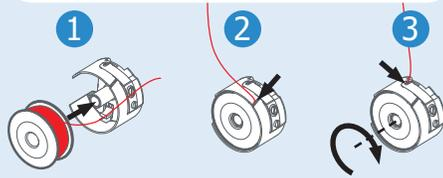
**Tension Test:** Hold the bobbin case in your hand and pull the thread up.
