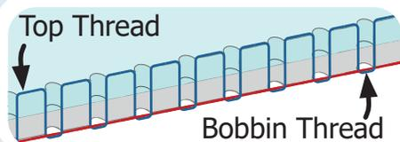
If the top thread is pulled through the bottom layer of fabric, increase tension.
