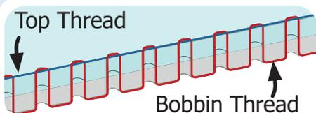
If the bobbin thread is pulled through the top layer of fabric, decrease tension.
