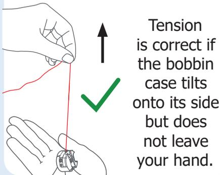
Tension is correct if the bobbin case tilts onto its side but does not leave your hand.
