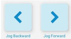
Press to move the needle up or down in small increments.
