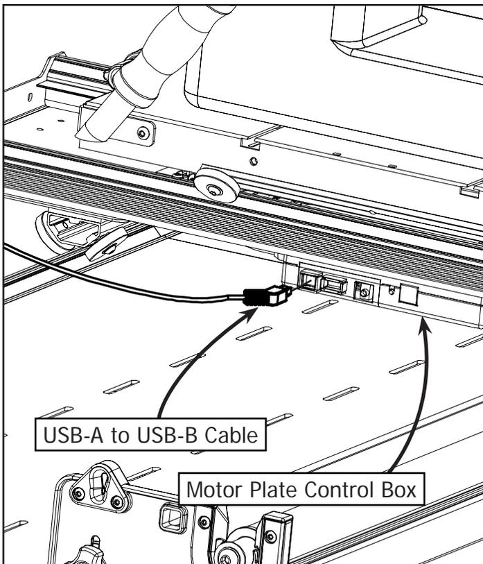
**2-1:** Connect the USB-A to USB-B Cable to the Motor Plate Control Box.
