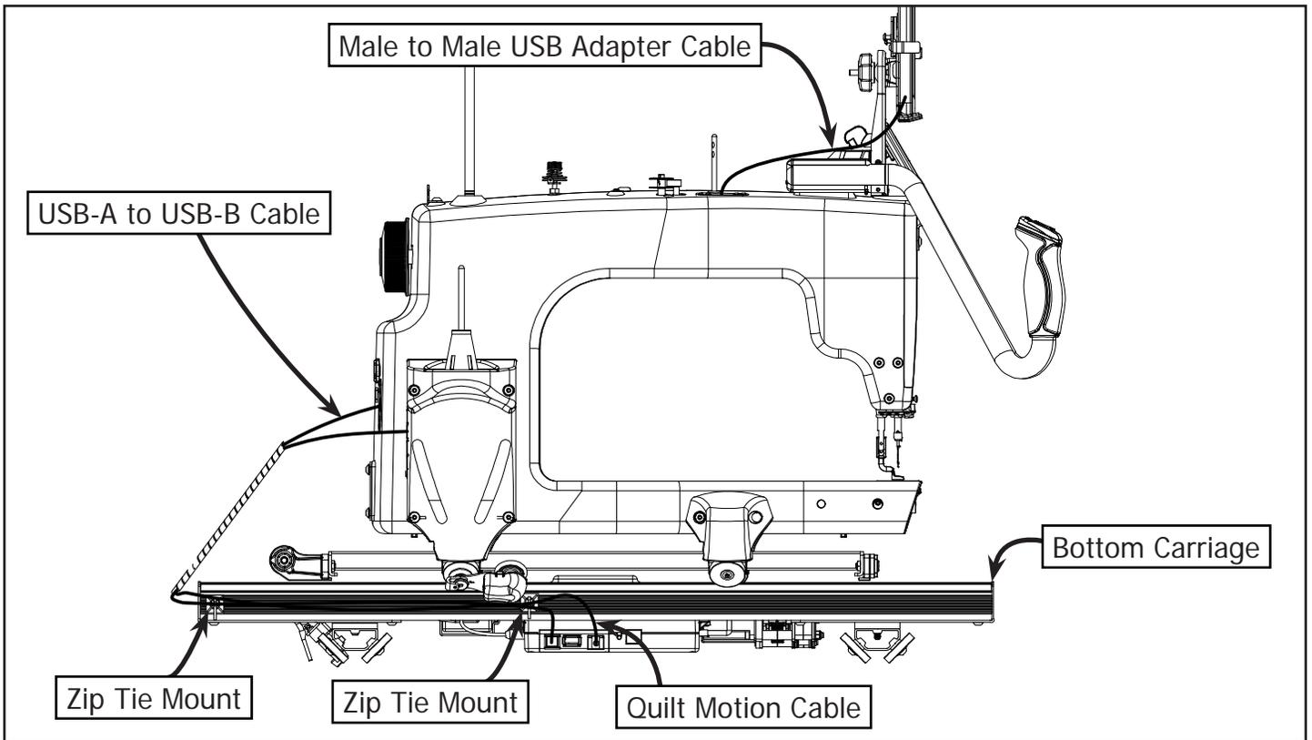
**2-6:** Secure Zip Tie Mounts to the Bottom Carriage. Wrap USB-A to USB-B Cable and Quilt Motion Cable together in the Cable Wrap and route cables as shown.
