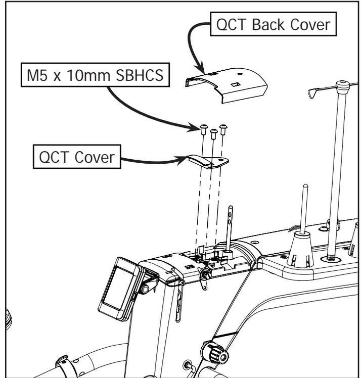
**1-1:** Remove the QCT Back Cover, (3) M5 x 10mm SBHCS, and the QCT Cover from the top of the sewing machine.
