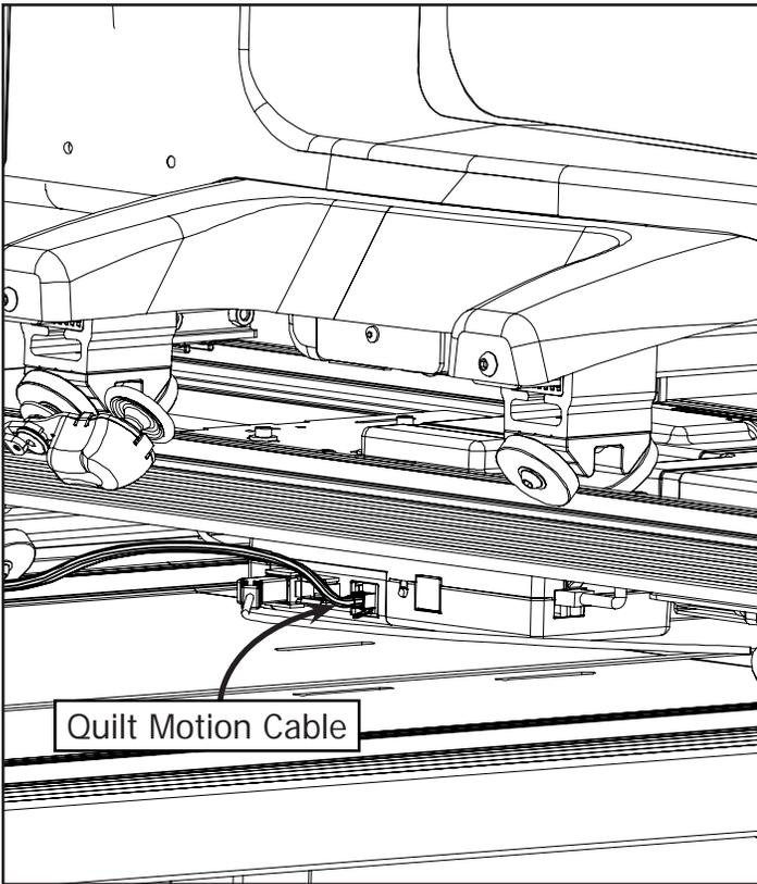
**2-3:** Connect the Quilt Motion Cable to the Motor Plate Control Box.
