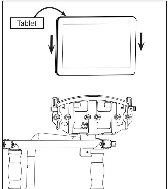
**1-5:** Slide your tablet into the Tablet Tray. Tighten the screws that were loosened in Step 1-4.
