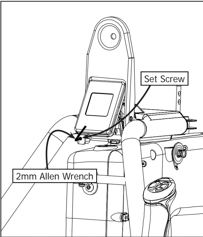
**1-4:** Use the 2mm Allen Wrench to tighten the (2) set screws on the front of the QCT Bracket Q'nique 15.
