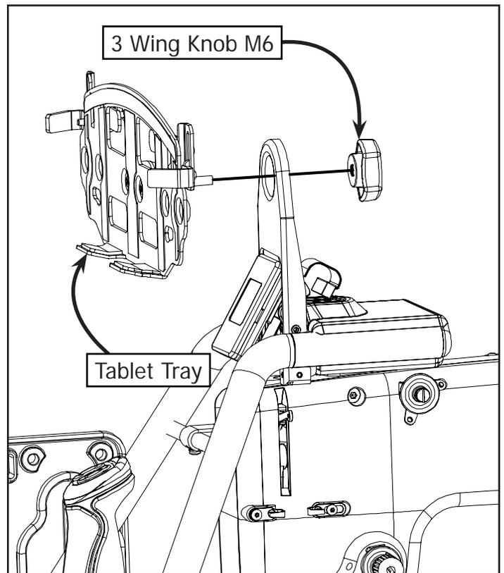
**1-5:** Install the Tablet Tray to the QCT Bracket Q'nique 15 using the 3 Wing Knob M6.
