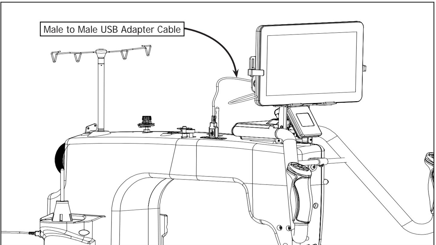
**2-5:** Connect the Male to Male USB Adapter Cable to the port on the top of your machine. Connect the opposite end to your tablet.
