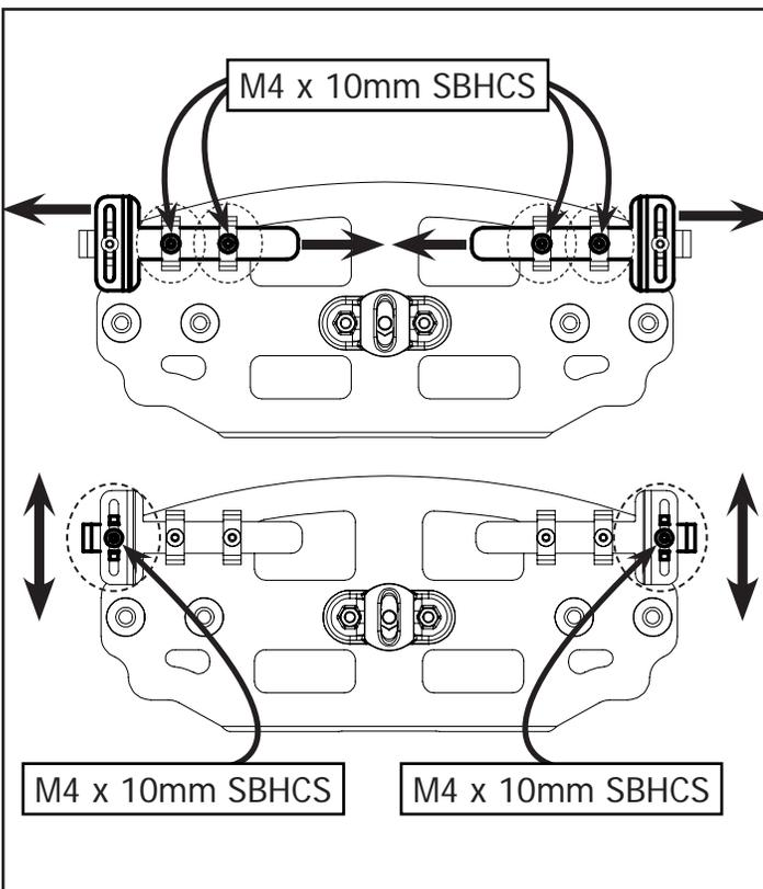
**1-6:** Loosen the circled M4 x 10mm SBHCS in order to adjust the arms of the Tablet Tray to fit your tablet.
