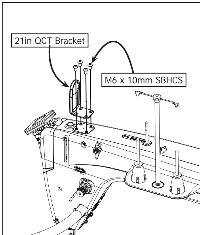
**1-2:** Install the 21in OCT Bracket using (4) M6 x 10mm SBHCS.
