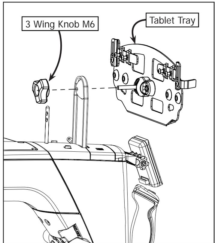
**1-3:** Install the Tablet Tray to the QCT Bracket Q'nique 19 using the 3 Wing Knob M6.
