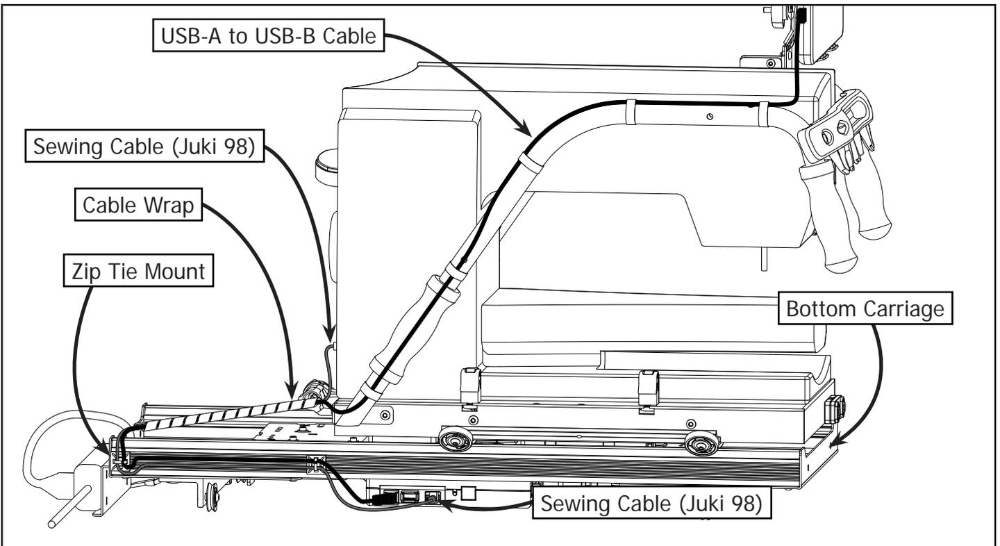
**2-6:** Secure Zip Tie Mounts to the Bottom Carriage. Wrap the USB-A to USB-B Cable and Sewing Cable (Juki 98) together in the Cable Wrap and route cables as shown.
