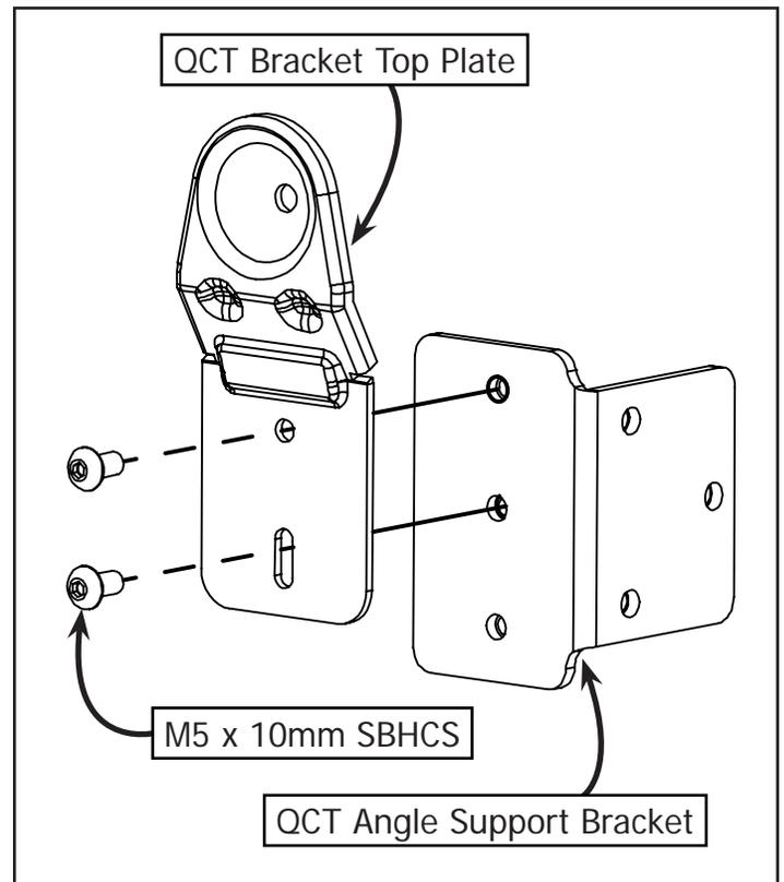
**1-1:** Attach the QCT Bracket Top Plate to the QCT Angle Support Bracket using (2) M5 x 10mm SBHCS.
