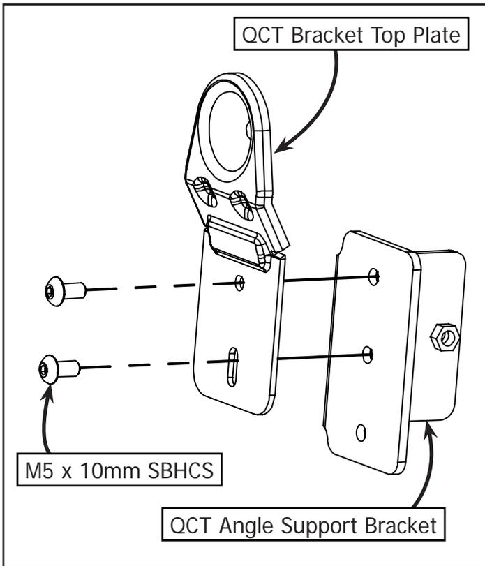
**1-3:** Attach the QCT Bracket Top Plate to the QCT Angle Support Bracket using (2) M5 x 10mm SBHCS.
