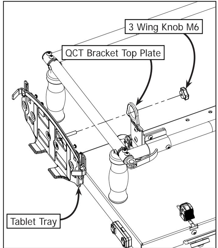
**1-3:** Install the Tablet Tray using the 3 Wing Knob M6 to the QCT Bracket Top Plate.
