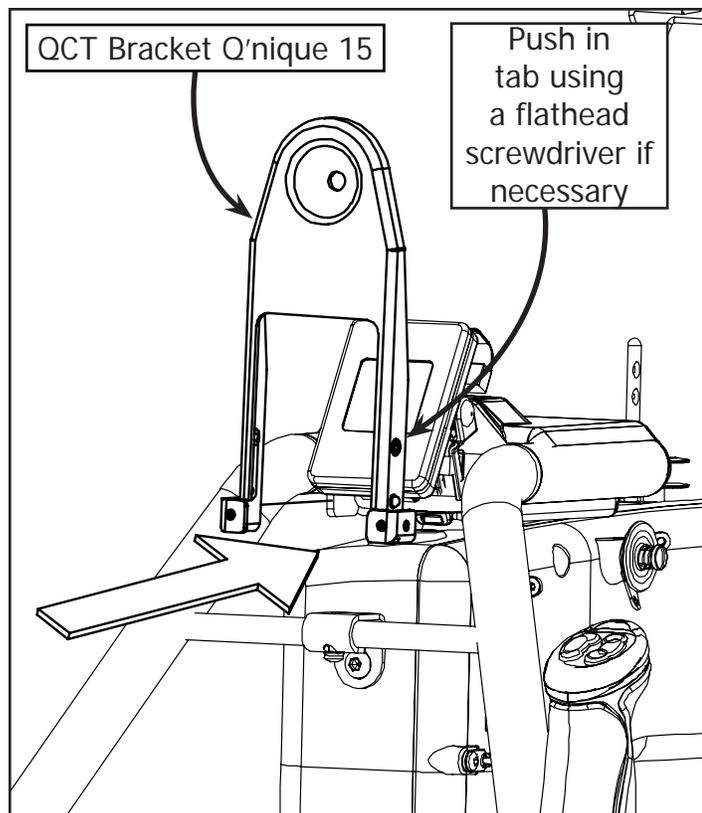
**1-2:** Place the QCT Bracket Q'nique 15 onto the handle bars as shown until the locator tabs snap into place.
