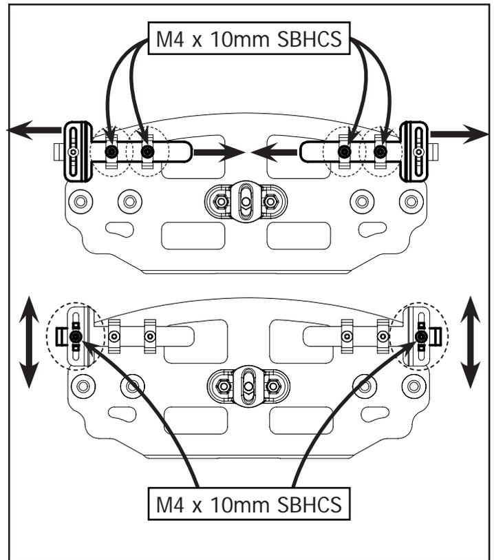
**1-4:** Loosen the circled M4 x 10mm SBHCS in order to adjust the arms of the Tablet Tray to fit your tablet.
