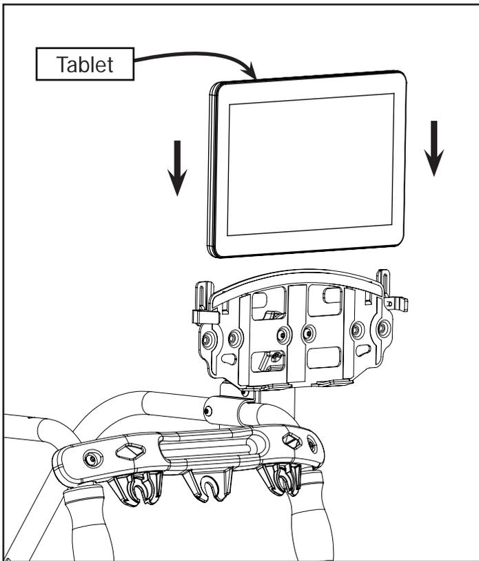
**1-7:** Slide your tablet into the Tablet Tray. Tighten the screws that were loosened in Step 1-6.
