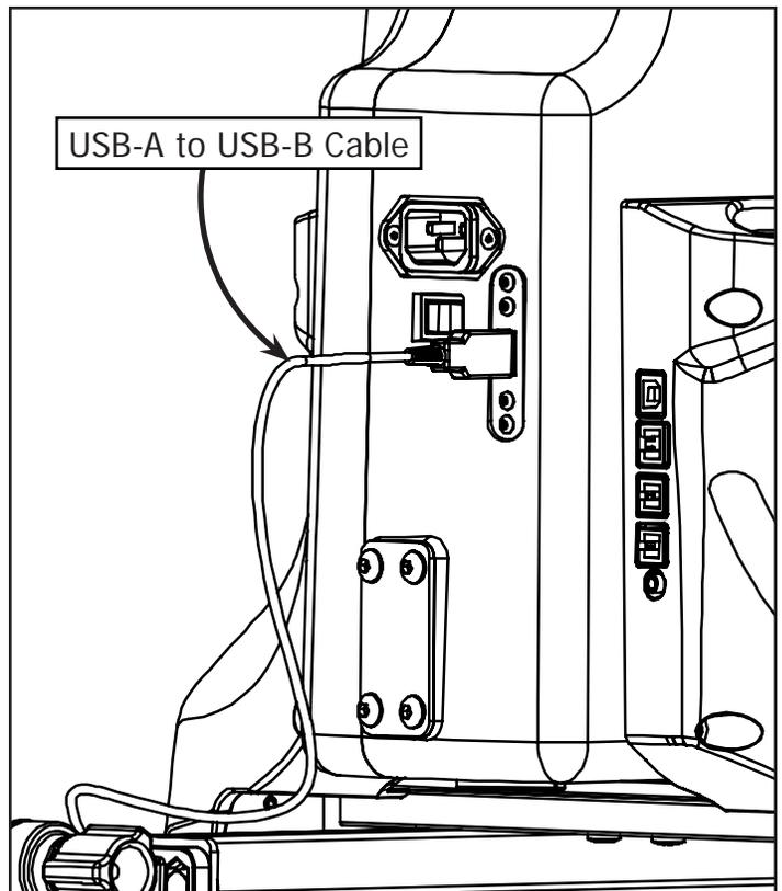
2-2: Connect the opposite end of the USB-A to USB-B Cable to the USB Port on the back of your machine.
