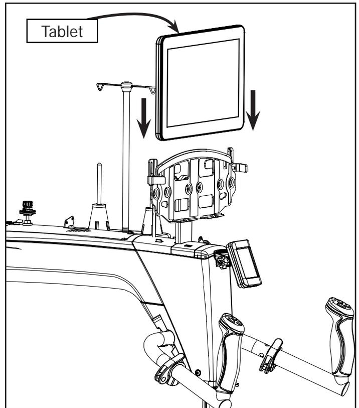
**1-5:** Slide your tablet into the Tablet Tray. Tighten the screws that were loosened in Step 1-4.
