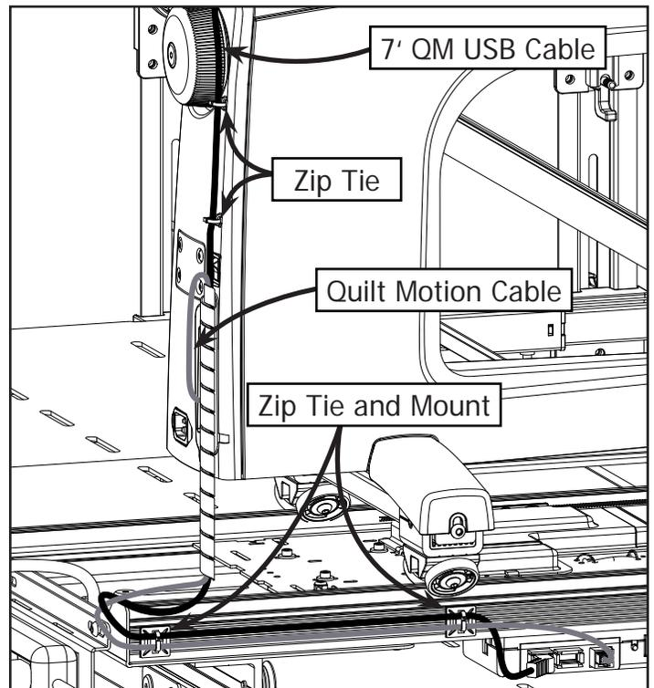
**2-3:** Secure the Quilt Motion Cable and the 7' QM USB Cable with Cable Wrap and (2) Zip Ties and Mounts to the carriage. Secure the 7' QM USB Cable to the back of the machine using an additional (2) Zip Ties.
