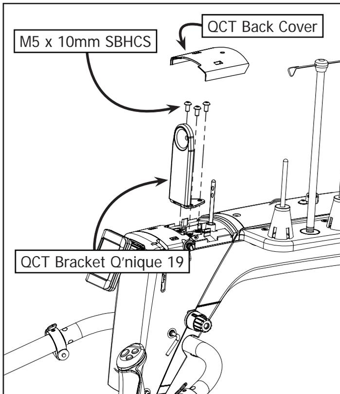
**1-2:** Install the QCT Bracket Q'nique 19 using the (3) M5 x 10mm SBHCS from step 1-1. Reinstall the QCT Back Cover.
