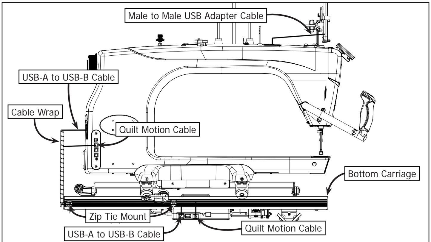
**2-6:** Secure Zip Tie Mounts to the Bottom Carriage. Wrap the USB-A to USB-B Cable and Quilt Motion Cable together in the Cable Wrap and route cables as shown.
