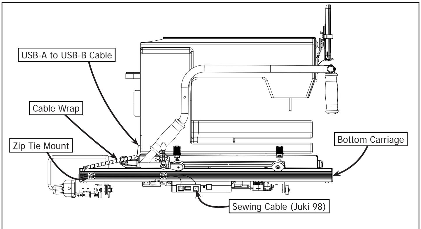
**2-5:** Secure Zip Tie Mounts to the Bottom Carriage. Wrap the USB-A to USB-B Cable and Sewing Cable (Juki 98) together in the Cable Wrap and route cables as shown.
