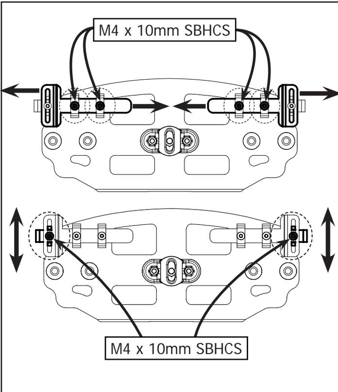
**1-4:** Loosen the circled M4 x 10mm SBHCS in order to adjust the arms of the Tablet Tray to fit your tablet.
