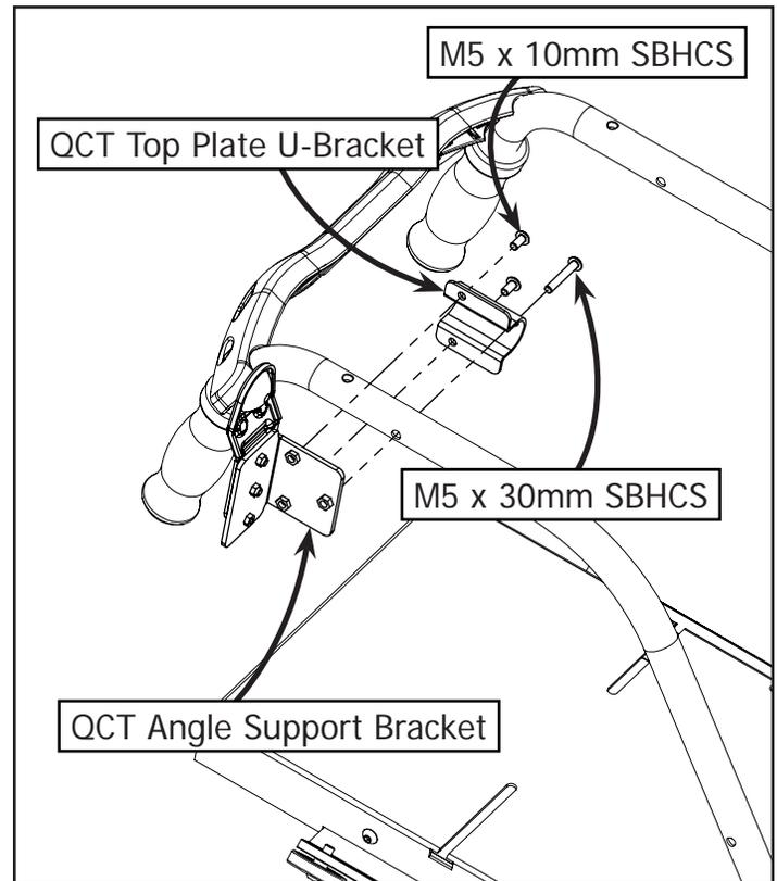
**1-4:** Attach the QCT Angle Support to the Top Plate using the QCT Top Plate U-Bracket, (2) M5 x 10mm SBHCS, and (1) M5 x 30mm SBHCS.
