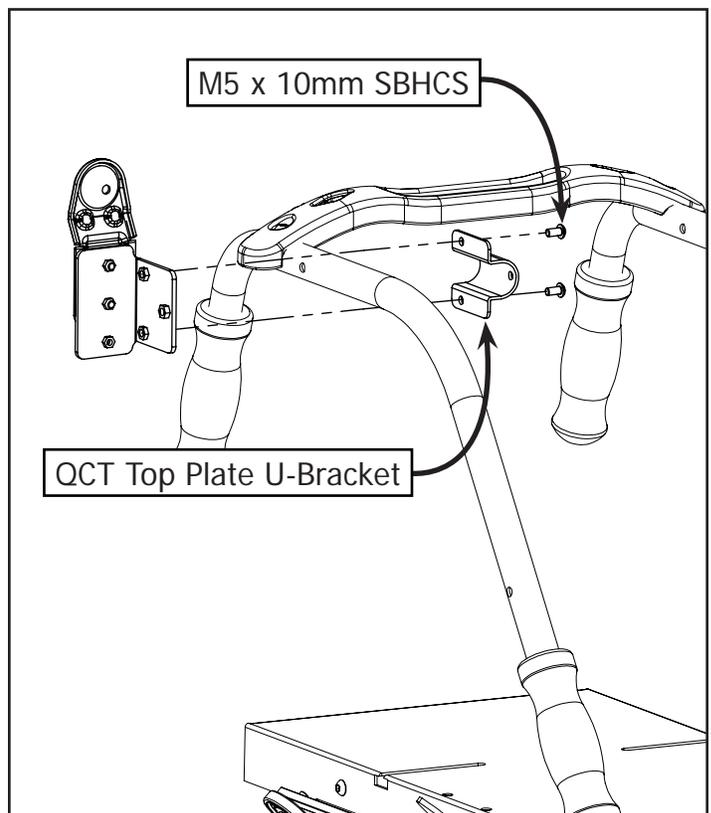
**1-1:** Attach the QCT Bracket Top Plate to the QCT Angle Support Bracket using (2) M5 x 10mm SBHCS.
