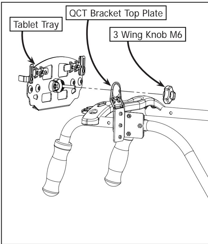
**1-3:** Install the Tablet Tray to the QCT Bracket Top Plate using (1) 3 Wing Knob M6.
