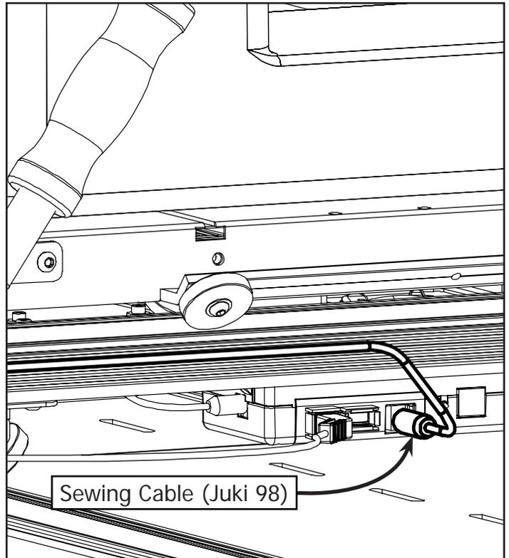
**2-4:** Connect the Sewing Cable (Juki 98) to the Motor Plate Control Box. Connect the opposite end to the foot pedal port of your sewing machine.
