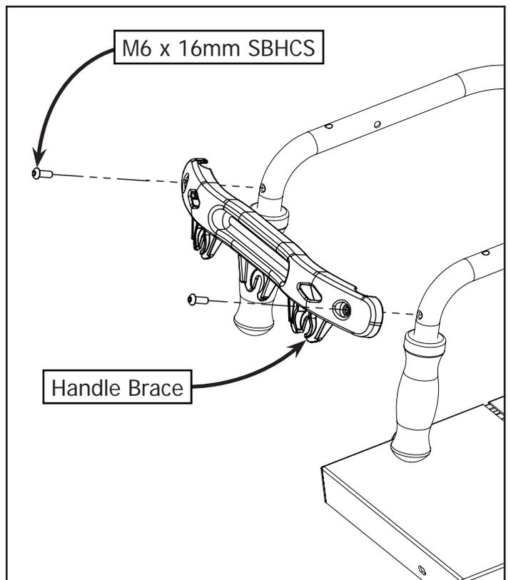
**1-2:** Reinstall the Handle Brace using the (2) M6 x 16mm SBHCS from Step 1-1 to the front holes on the handles.
