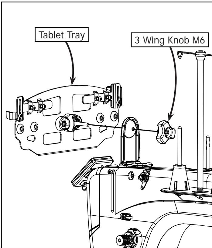
**1-3:** Install the Tablet Tray to the 21in QCT Bracket using the 3 Wing Knob M6.
