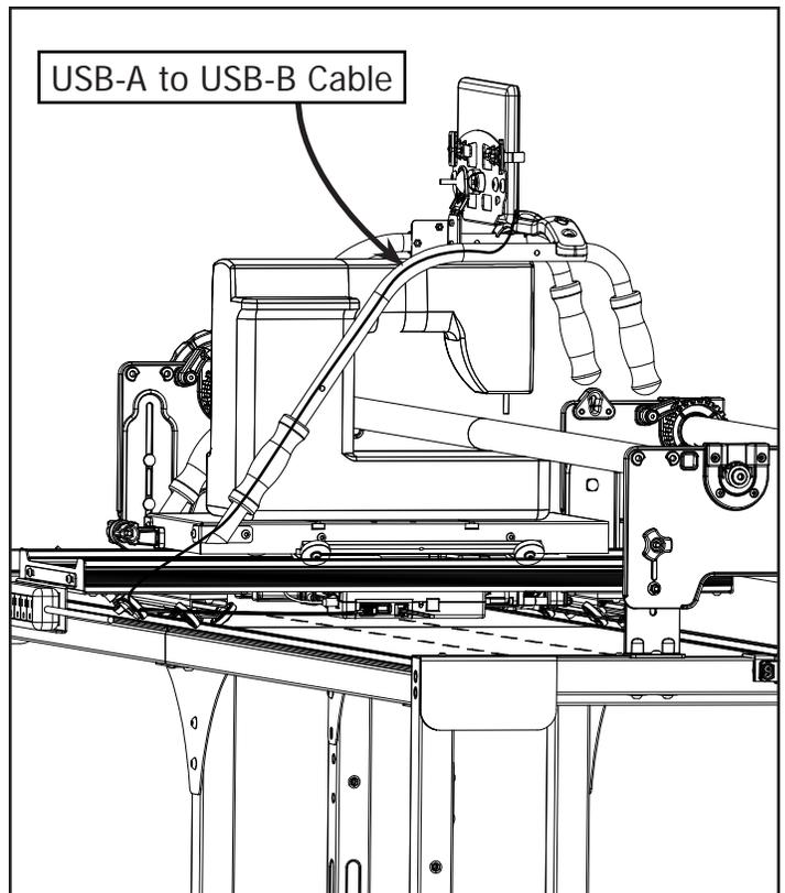
**2-2:** Connect the opposite end of the USB-A to USB-B Cable to the USB Port on your tablet.
