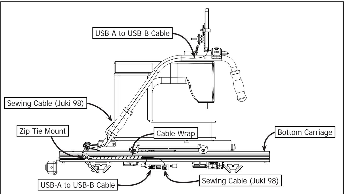
**2-4:** Secure Zip Tie Mounts to the Bottom Carriage. Wrap the USB-A to USB-B Cable and Sewing Cable (Juki 98) together in the Cable Wrap and route cables as shown.
