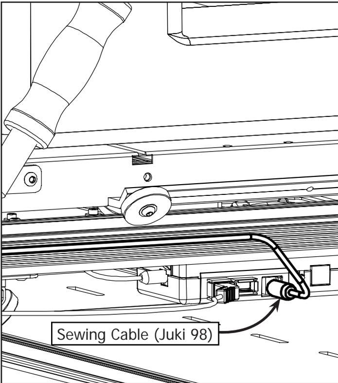
**2-3:** Connect the Sewing Cable (Juki 98) to the Motor Plate Control Box. Connect the opposite end to the foot pedal port of your sewing machine.
