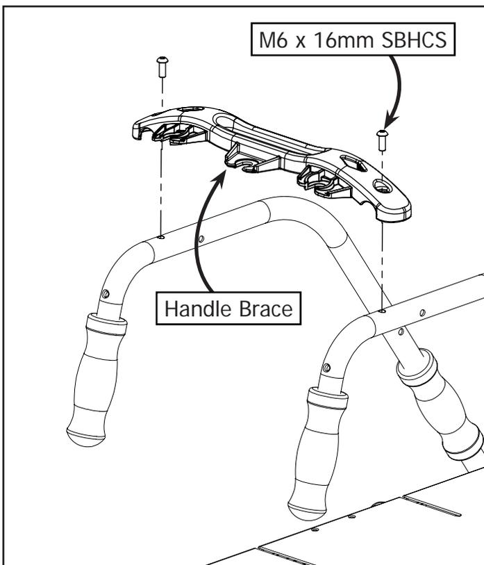
**1-1:** Remove the (2) M6 x 16mm SBHCS and the Handle Brace.
