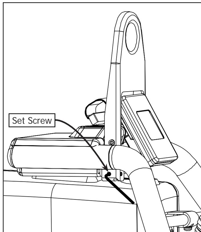
**1-3:** Use the 2mm Allen Wrench to tighten the (2) set screws on each side of the QCT Bracket Q'nique 15.
