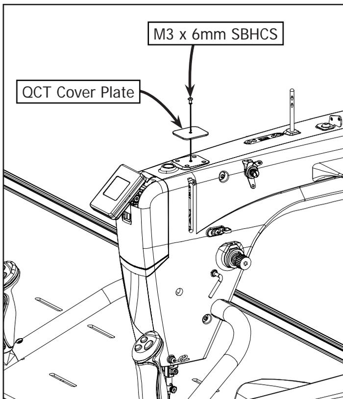
**1-1:** Remove the M3 x 6mm SBHCS and the OCT Cover Plate.
