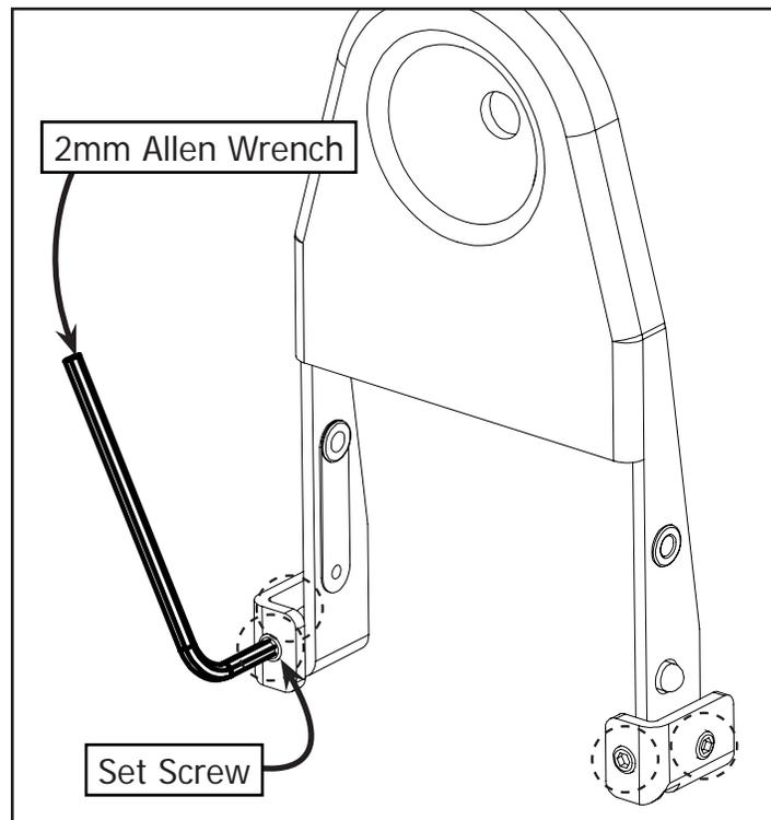
**1-1:** Using the 2mm Allen Wrench loosen all (4) set screws on the QCT Bracket Q'nique 15.
