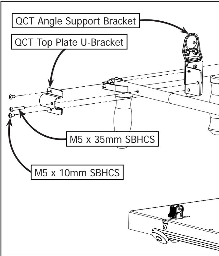
**1-2:** Attach the QCT Top Plate U-Bracket and the QCT Angle Support Bracket using (2) M5 x 10mm SBHCS and (1) M5 x 35mm SBHCS.
