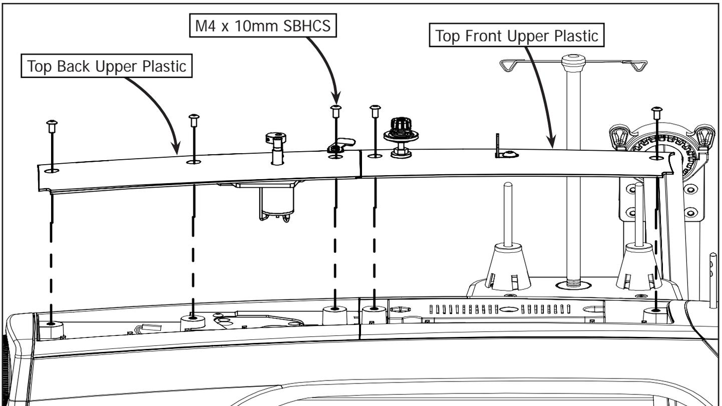
**2-1:** Remove the Top Front Upper Plastics and the Top Back Upper Plastics from your machine by removing the (5) M4 x 10mm SBHCS.
