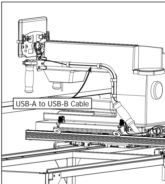
**2-3:** Connect the opposite end of the USB-A to USB-B Cable to the USB Port on your tablet.
