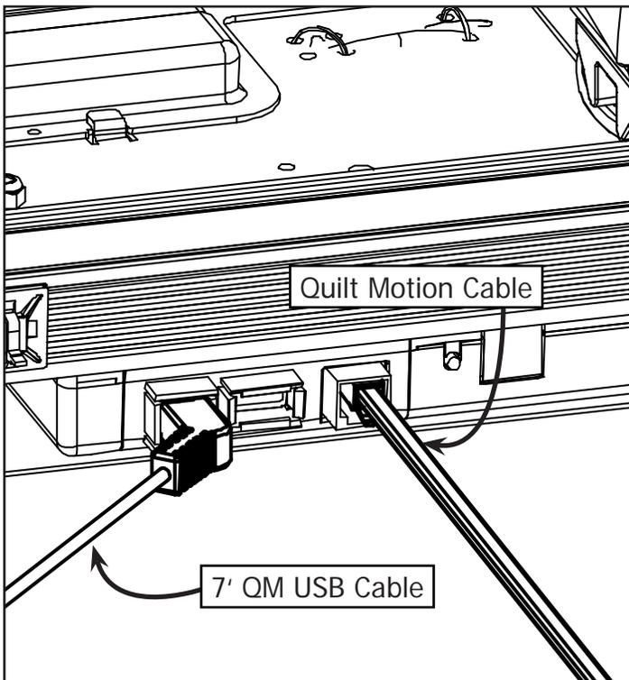
**2-2:** Connect the 7' QM USB Cable and the Quilt Motion Cable to the Motor Plate Control Box.
