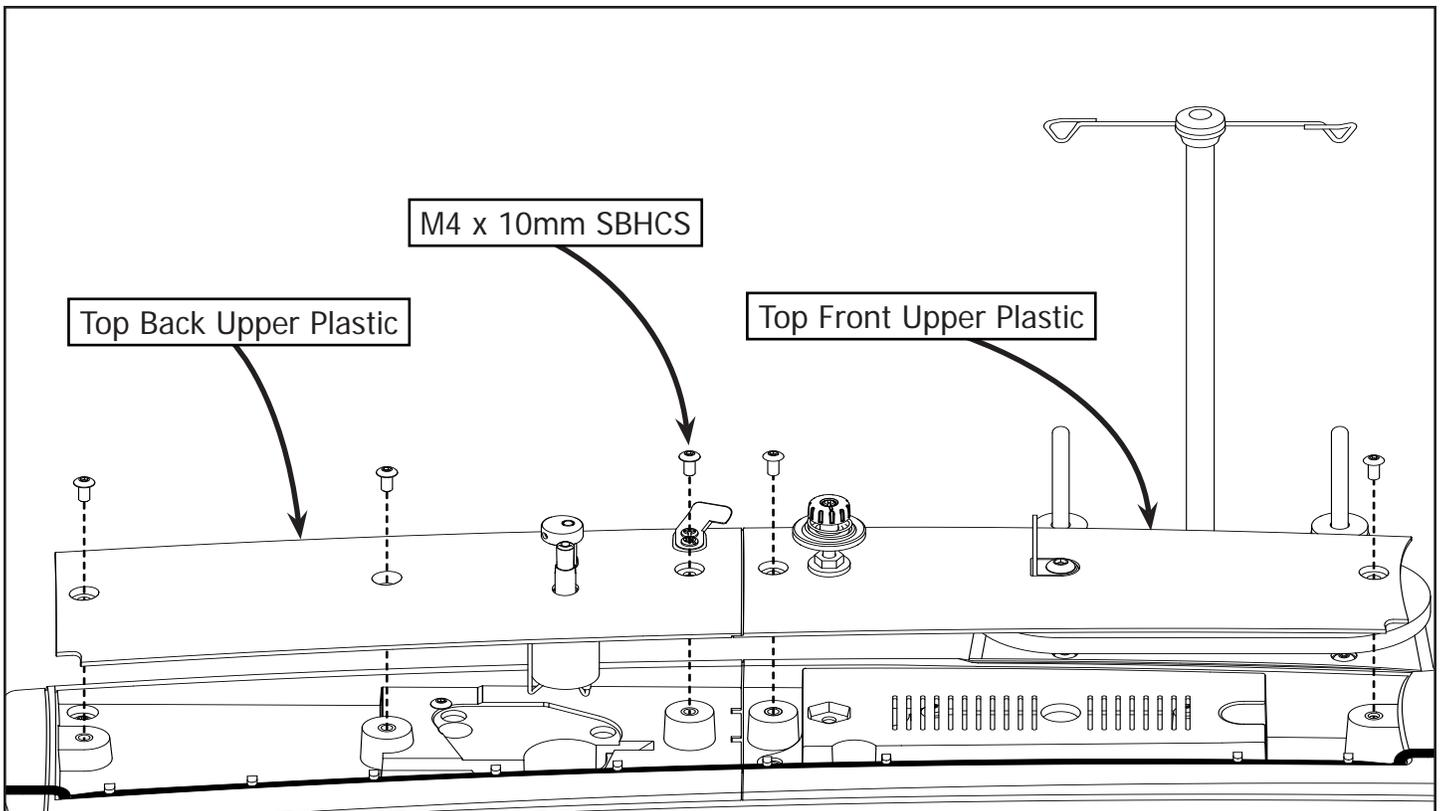
2-6: Reinstall the Top Front Upper Plastics and the Top Back Upper Plastics from your machine using the (5) M4 x 10mm SBHCS from Step 2.1 making sure to not pinch the 7' QM USB Cable.
