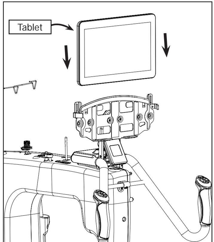
**1-7:** Slide your tablet into the Tablet Tray. Tighten the screws that were loosened in step 1-6.
