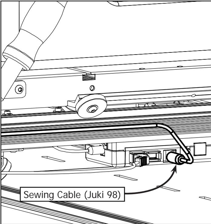
**2-3:** Connect the Sewing Cable (Juki 98) to the Motor Plate Control Box. Connect the opposite end to the foot pedal port of your sewing machine.
