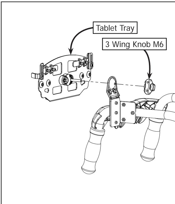
**1-5:** Attach the Tablet Tray to the QCT Bracket Top Plate using (1) 3 Wing Knob M6.
