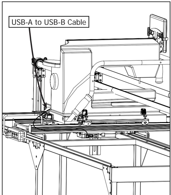
**2-2:** Route the USB-A to USB-B Cable long the side of the Top Plate as shown.
