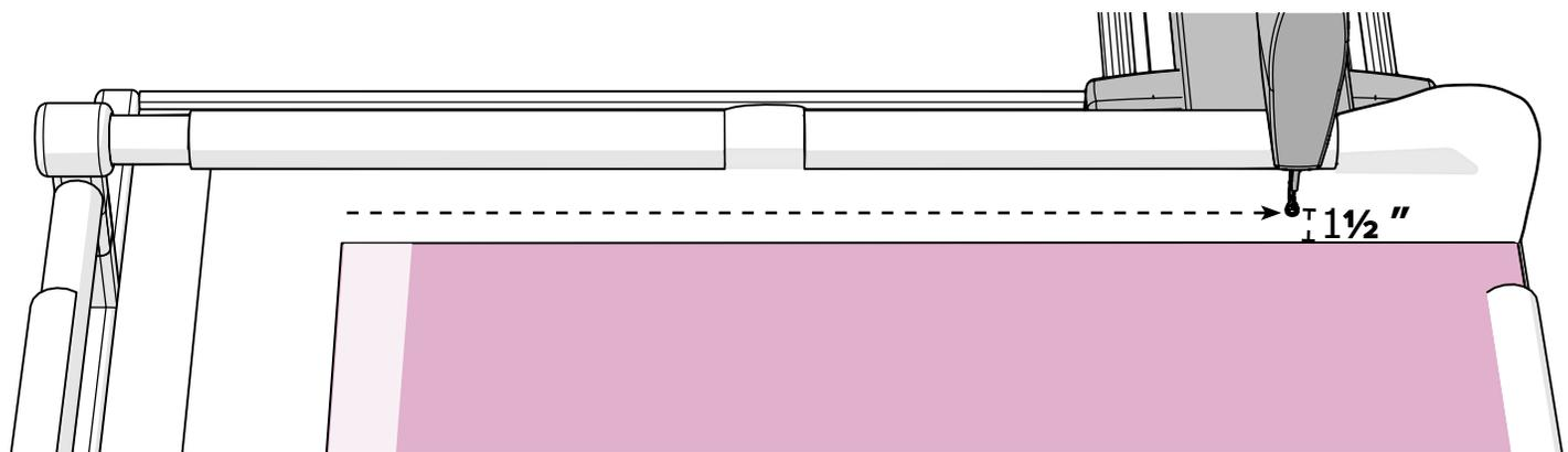
If your machine can do this without bumping into anything on the take-up rail, your fabric is positioned very well on the frame.
