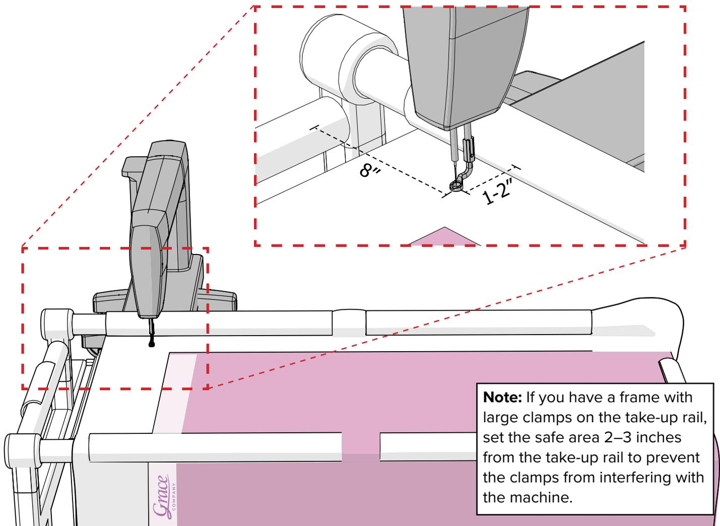
The software tracks your needle as you move it across the frame. In essence, you're using the needle as a pointer to tell the software where you want the back-left corner of the safe area to be.
