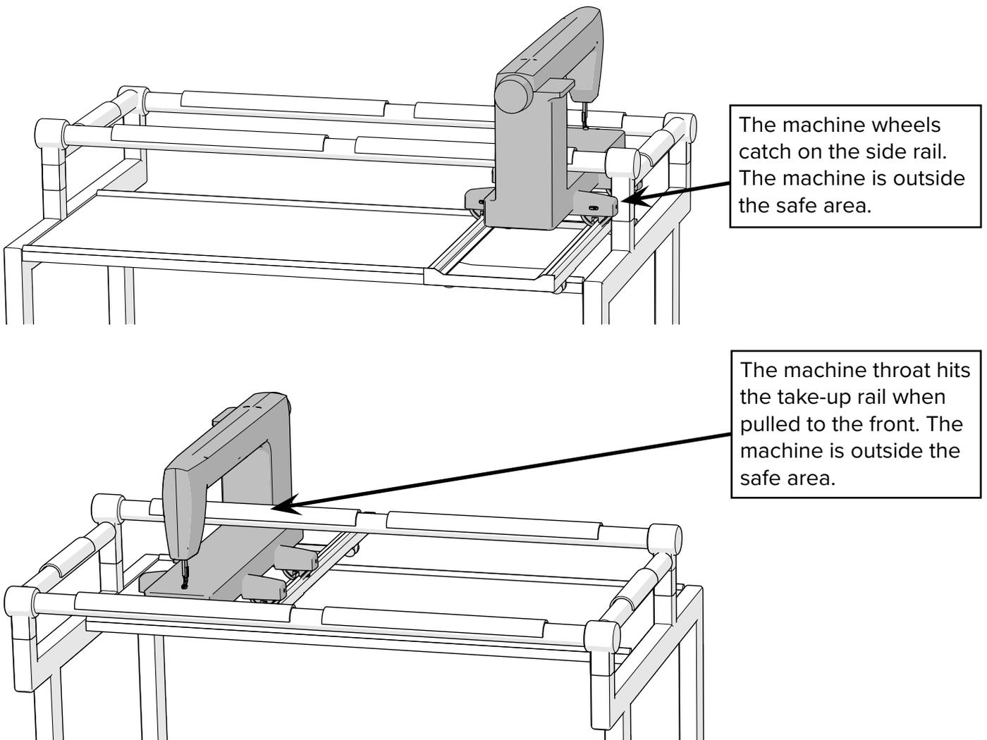
The safe area is different for every quilting setup, which is why the automation software can't tell where the safe area is on your frame without your help. In the following practice steps, you will use your machine to communicate the boundaries of your safe area to the software.
