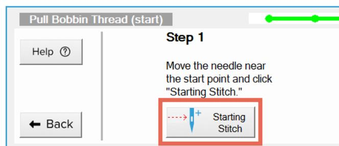
**IMPORTANT:** The machine moves when you press Starting Stitch on this screen.
