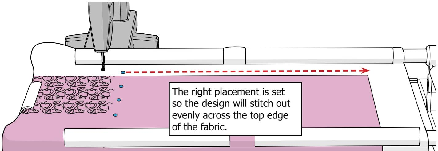
On the screen, tap **Move Right**. The machine travels to the corresponding right placement point.
