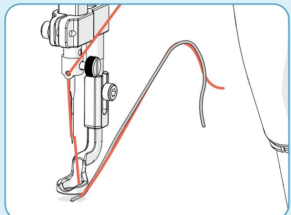
**Important:** When you move your machine back to the original stitch, slack bobbin thread builds up right under the fabric. Pull on bobbin thread tail until the resistance slightly increases.
