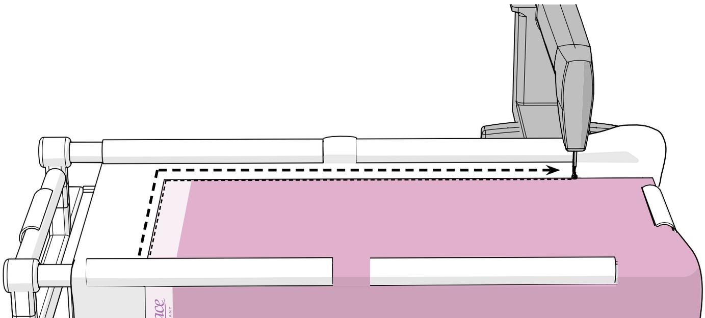
5 The bobbin thread must be pulled up at the end of a line of stitching as well.
