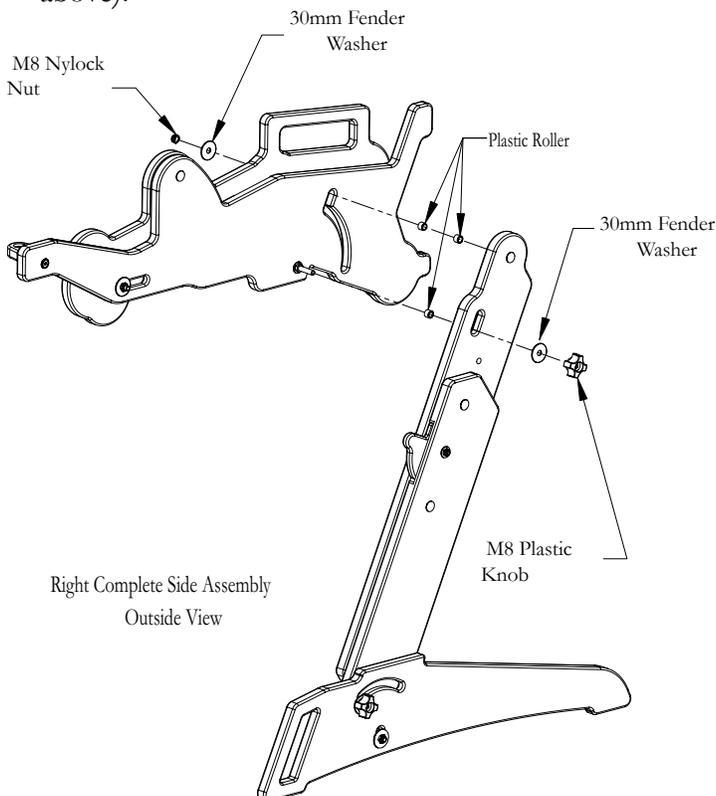
➤ With these parts together, place a fender washer onto each bolt.
