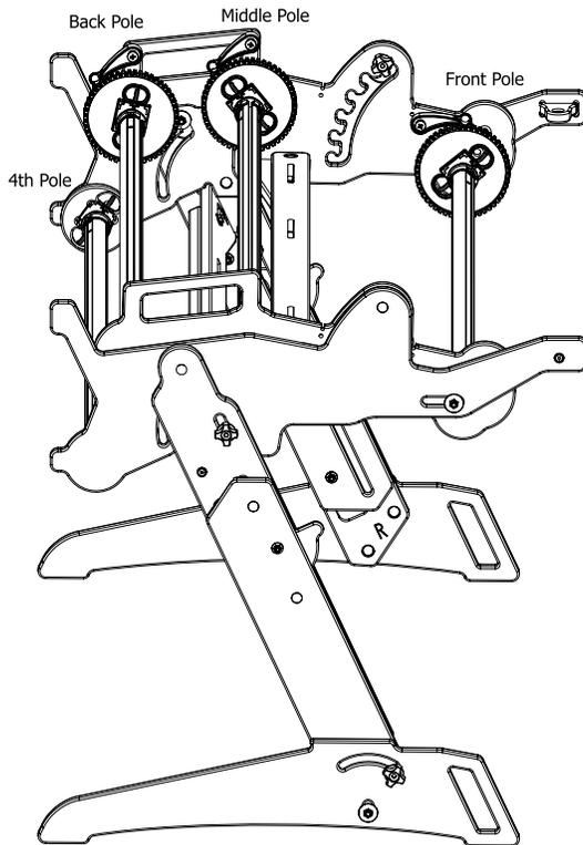
**\*\*\*IMPORTANT:** Before completing the next step, keep in mind that the truss bolt should be about 1/4” too long. **THE TRUSS BOLT SHOULD NOT BE TIGHTENED WITH ANY TOOL. TIGHTEN THIS BOLT WITH YOUR FINGERS ONLY, TO AVOID DAMAGE.**
