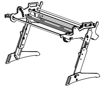
STEP 2: Lift the pole assembly up, and allow it to slide down. *When frame is set up in bigger sizes, it is recommended you do this one side at-a-time.*
