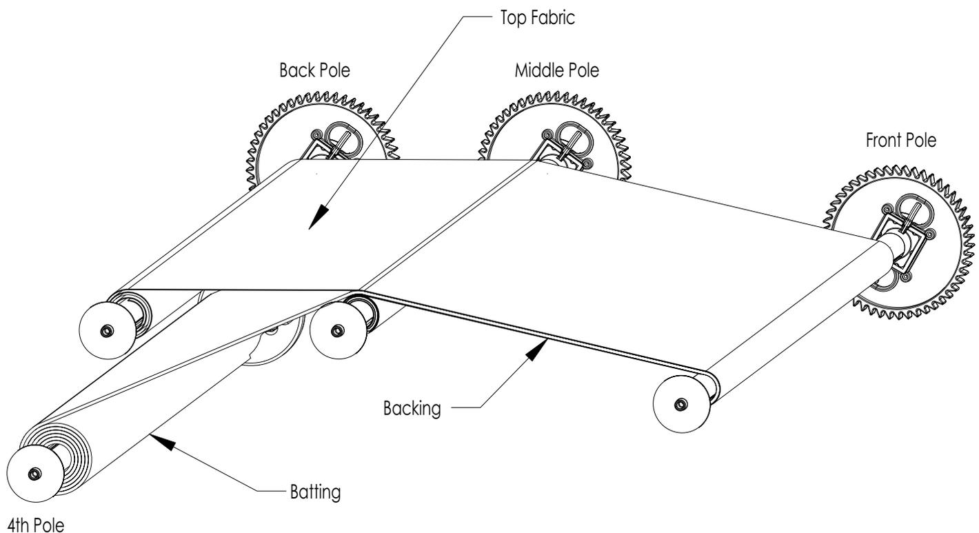
7. Measure the quilt top edge to the end boards. This measurement should be the same distances as on the front pole.
