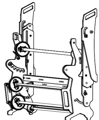
**\*\*\*NOTE: IF THE FRAME PARTS DO NOT MOVE AT THE JOINTS SMOOTHLY, CHECK THE NYLOCK NUTS AND MAKE SURE THEY ARE NOT OVERTIGHTENED.**
