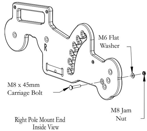
**STEP 2: HARDWARE AND LAMP HOLDERS TO LEFT AND RIGHT PIVOT SECTIONS**
