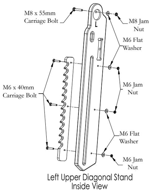
➤ First, put a M8 x 55mm carriage bolt through the top hole of the Left Upper Diagonal Stand. The head of the bolt should be on the outer side of this part.
