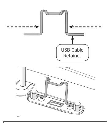
**Note:** The retainer may slide side to side once in the holes, and you may need to re-insert one of the ends into the screw. It will stay in place once the USB is plugged in.
