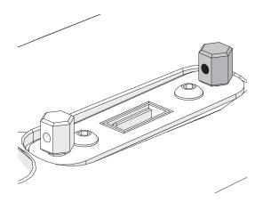
5 Pinch the sides of the **USB cable retainer** and insert the ends into the holes in the retainer screws.
