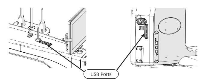
2 Use the 2 mm Allen wrench to remove **one** of the **outside screws** for the top USB port.
