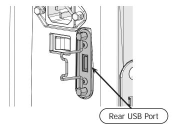
8 Plug the USB end of the Q'nique to QuiltMotion cable into the rear USB port and lift the retainer to wrap around the cable and hold it in place. Plug the other end of the cable into the left port of the motor plate.
