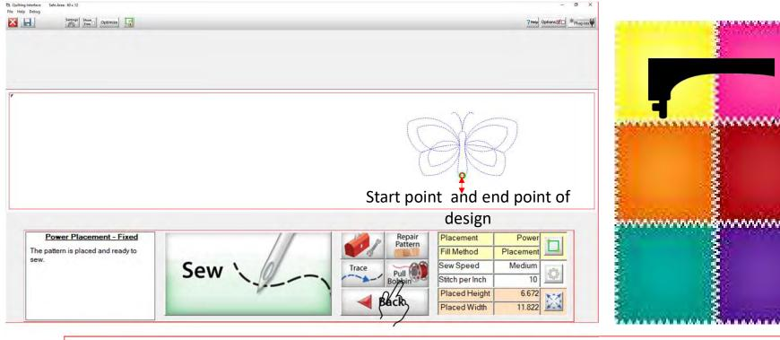
Once the machine has moved to where it will start sewing, your needle will automatically go down into the fabric to catch your bobbin thread. After it has finished going down into your fabric you will see the prompt again asking if your needle is up. Click "OK."
