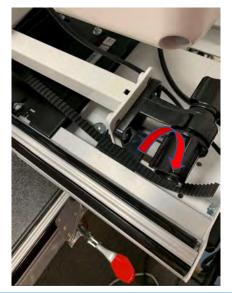
6. Using the left knob of the bracket, unscrew the belt out of the bracket.
