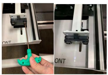
2. Using the M3 allen wrench loosen the two screws on the front belt bracket.
