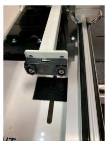
Retighten the screws and bracket without the belt.
