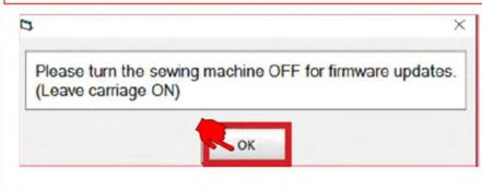
35. The "Firmware Load Button Push" window will appear. Push in the firmware button located on the bottom carriage under your sewing machine. Push the button two times, you will have 20 seconds to push it twice. Then click "OK" on your tablet screen.
