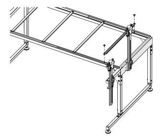
111 Press the extended plastic tracks onto both the front and back track supports.
