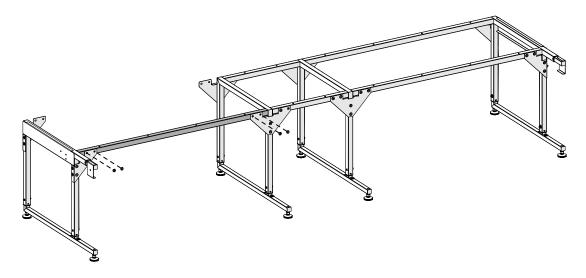
8 Loosely attach the final cross support tube to the back of the frame.
