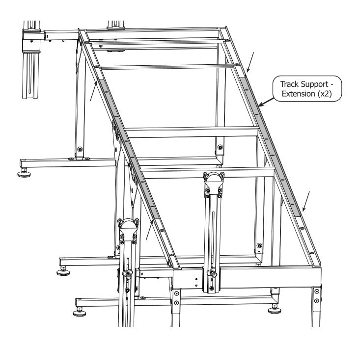
5 Attach a table support tightly to the left end of the extended track support. As you tighten the connector bolt, make sure the track support vertical edges stay aligned.
