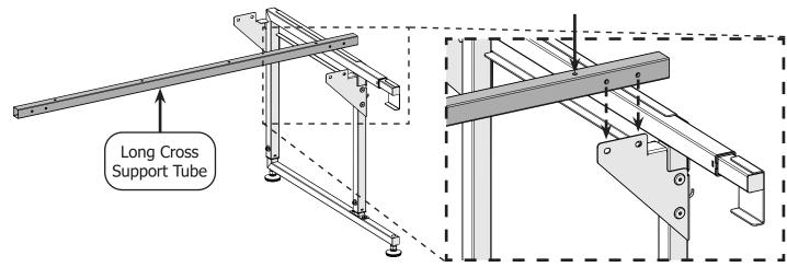
2 Loosely connect the cross support tube to the corner brace with two M6 x 10 mm connector bolts and the 4 mm Allen wrench. Again, do not fully tighten any connector bolts until instructed.
