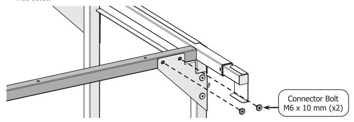
3 Loosely attach the other end of the cross support tube to the front brace on a middle leg assembly. Use two connector bolts.
