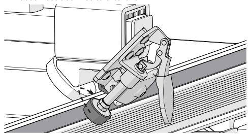
**Note:** If twisted too far, the handle will start to open, and eventually the foot will fall out. Reverse the direction you're twisting until the handle is pointing down, but the foot still reaches the track.
