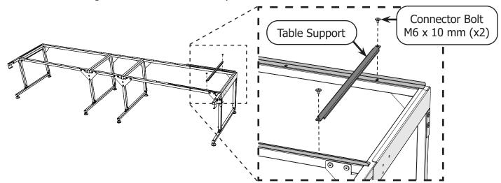
4 Loosely attach a second table support to the frame with two M6 x 10 mm connector bolts.
