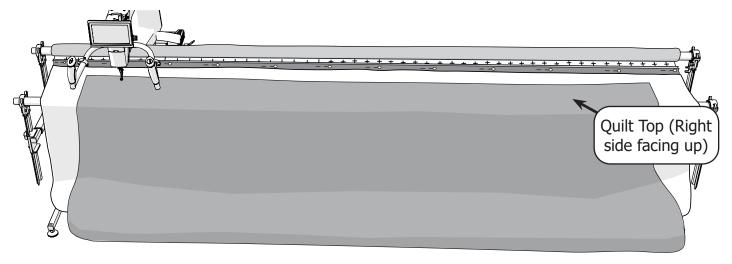
Repeat step 9 to move the fabric but this time position the quilt top so its top edge is 2–3 inches from the take-up rail (the back rail).
