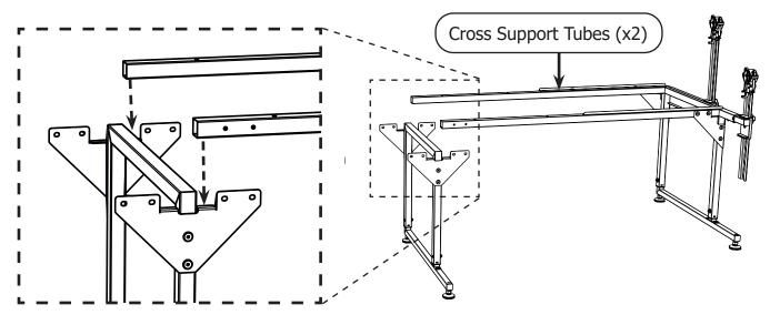
4 Loosely attach the cross support tubes with the four M6 x 10 mm connector bolts you removed earlier.
