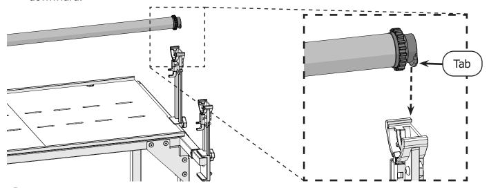
9 Slide the **ratchet cap** onto the top of the bracket.
