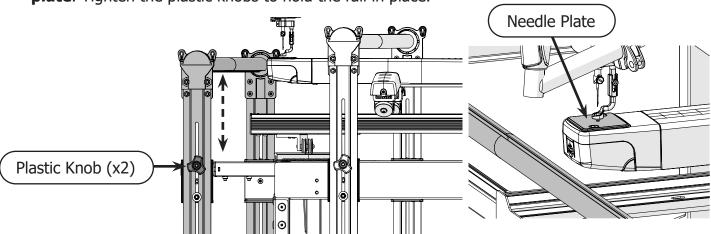
4 Adjust the height of the take up rail by loosening the **plastic knobs** on both rear rail holder brackets. Position the rail so that it is approximately **1/4 inch** above the throat of the machine. Tighten the plastic knobs to hold the rail in place.
