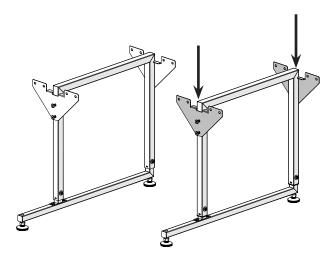
**Result:** The frame braces are loosely installed on all the legs. Do not tighten the connector bolts yet.
