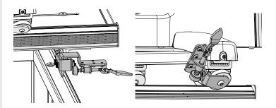
3 Move the machine to the left side of the frame and place the machine in the middle of the bottom carriage. Let go of the machine to see if it rolls and in which direction.
