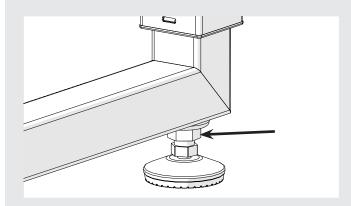
b Turn the bottom nut with the 14 mm Openend wrench until the desired height is set.
