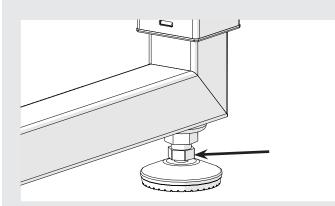
C Tighten the top nut with the 17 mm Openend wrench until it is firm against the frame leg.
