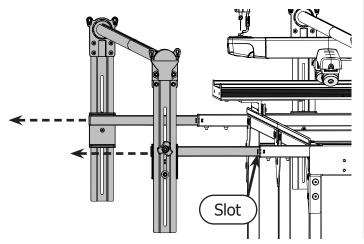
**Note**: If your machine has a throat length of less than 16 inches, move the machine as far forward as you can and then adjust the quilt-backing rail until it is 1 inch from the front of the machine. Tighten the set screws.
