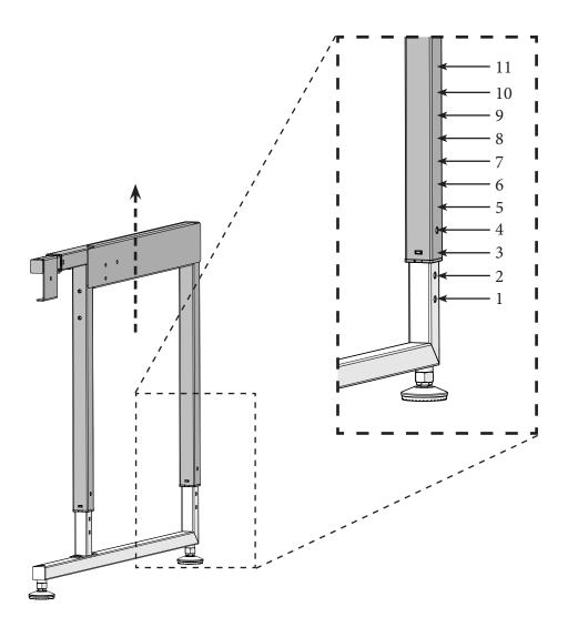
5 Reinstall the height screws through the selected height holes. Cap the screws with the washers, and nuts and tighten with the Allen wrench and 10 mm open-end wrench.
