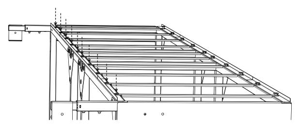
3 Press the two plastic tracks onto the vertical edge of the front and back track supports.
