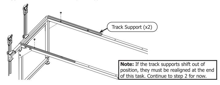
2 <u>Tightly</u> attach a **table support** onto the frame with the connector bolts you removed. As before, be careful not to shift the track supports.
