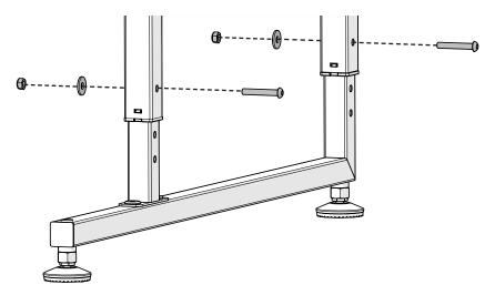
6 With the Allen wrench, tighten the connector bolts.
