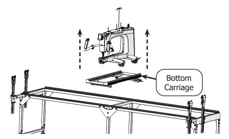
4 Pull the two **plastic tracks** off of the track supports. These plastic tracks do not fit on the extended frame and can be discarded.
