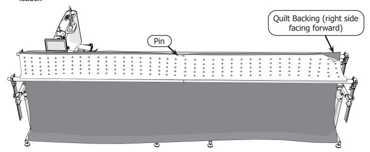
**Right Side/Wrong Side:** Some fabrics have a front side that has a print or other qualities that the back side does not have, or may look washed out on the back. The front of the fabric is called the "right side." The side that looks washed out or doesn't have the print/texture is called the "wrong side."
