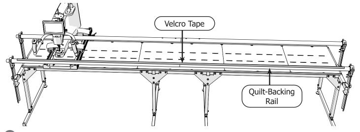
4 Repeat steps 2–3 to install the Velcro tape onto the take-up rail.
