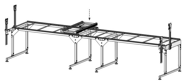
13 Test the track alignment. All four bottom carriage wheels should ride the track smoothly over the full length of the frame.
