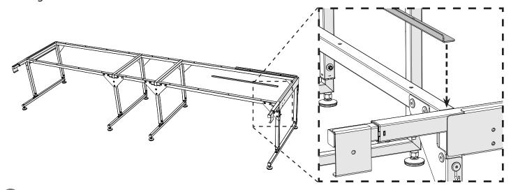
3 Use two **M6 x 10 mm connector bolts** to attach the **table support** and track supports to the frame. Do not tighten the connector bolts yet.
