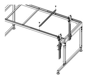
110 Repeat steps 8-9 on the remaining connector bolts on the right track supports.
