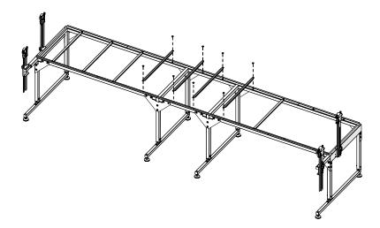
8 With a 4 mm Allen wrench, unscrew the connector bolts on the left end of each of the right track supports. Take care not to bump the supports or allow them to shift.
