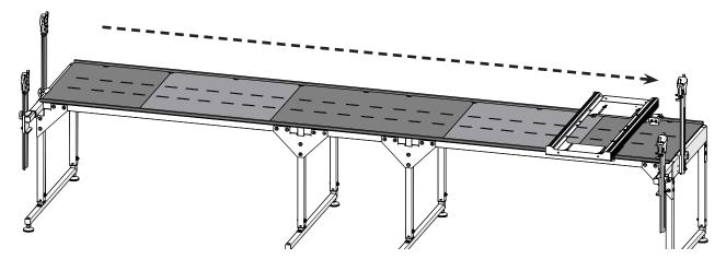
6 **Result:** The plastic table surfaces are installed and do not interfere with the movement of the bottom carriage.
