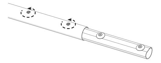
3 Slide a **2-ft extension ratcheting rail assembly** onto the other side of the rail coupler so the holes and screws align.
