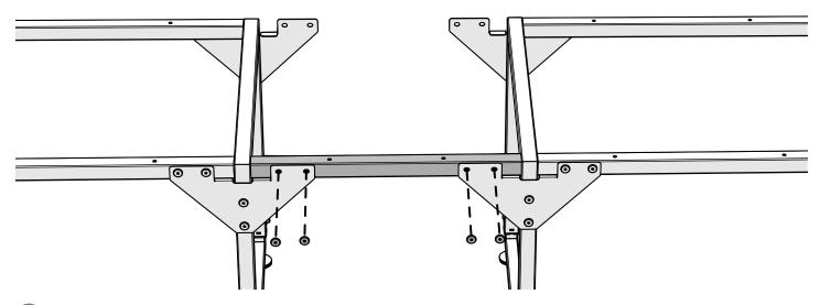
6 Repeat steps 4-5 to loosely attach the second 2 ft cross support tube to the middle braces on the back of the frame.
