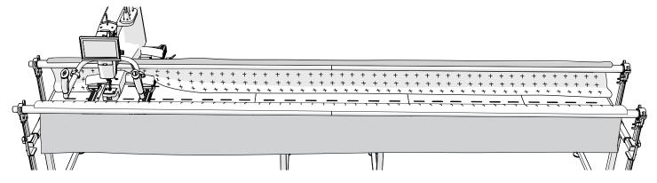
8 **Result:** The cloth leaders are installed and fabric can now be loaded onto the frame for quilting.
