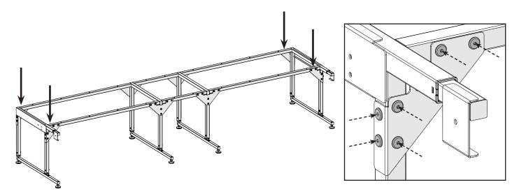
11 Tighten the six connector bolts on the four middle braces.
