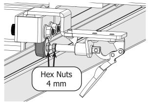
10 Result: The channel lock is installed on the back-right wheel of the bottom carriage.
