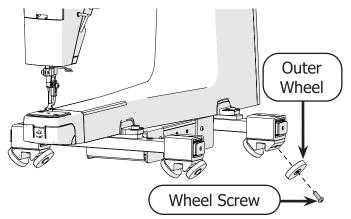
3 Place the **dual-wheel channel lock** onto the **M6 x 20 mm SBHCS.** Follow it with the wheel, with the **wheel hub** facing away from the channel lock.
