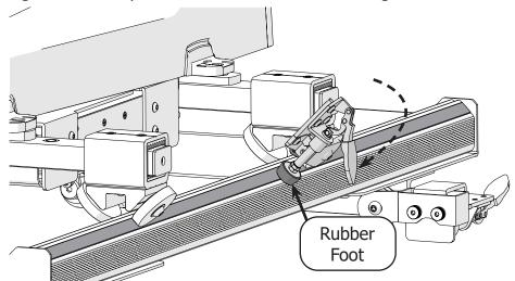
6 If the channel lock doesn't fully reach the track, or its grip on the track seems loose, twist the rubber foot clockwise to extend it.
