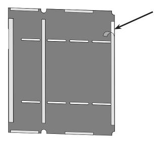
3 Carefully lower the table surface down onto the frame. Make sure the tape aligns with the supports and the table surface is centered between the two tracks.
