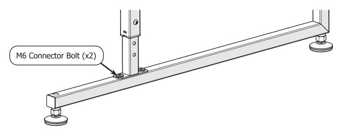
Repeat these steps (skipping step 3) to set the height on the **middle leg assemblies** and the **left leg assembly**. All four leg assemblies must be set to the same height.
