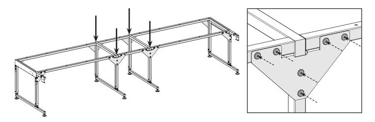
**Result:** The cross support tubes and braces are securely attached to the legs, creating the structure of the frame.
