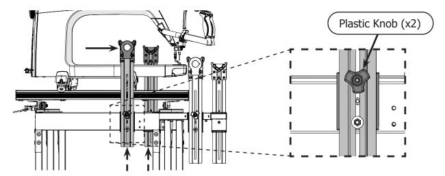
Slide one of the rails through the machine's throat and insert the end of the **floating rail** section into the hole in the rear **left rail holder bracket**.
