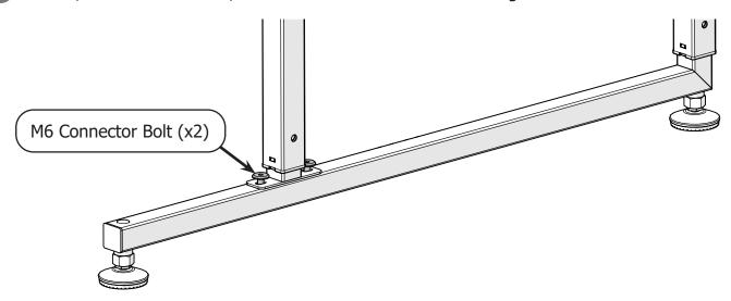
4 Lift the top of the leg so that it is set to the same height hole as the legs on your frame.
