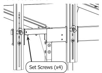
2 Pull on the brackets to extend the quiltbacking rail until you see the **slot** on the extension arms. Tighten the set screws.
