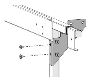
6 Loosely attach a **corner brace - A side** to the other side of the left leg with four connector bolts.
