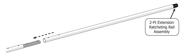
4 Loosen the screws with the 4 mm Allen wrench until they press firmly against the inside of the rail.
