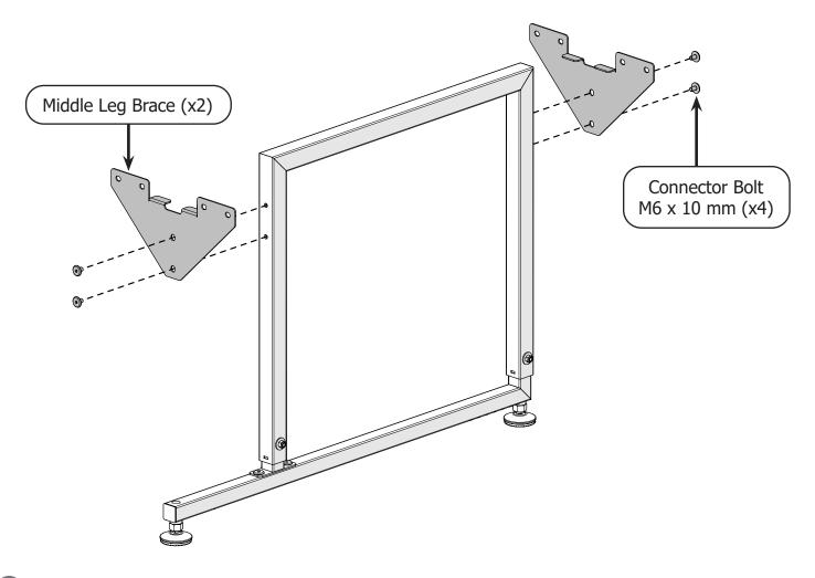
**Result:** The middle leg braces are loosely installed on the middle leg.
