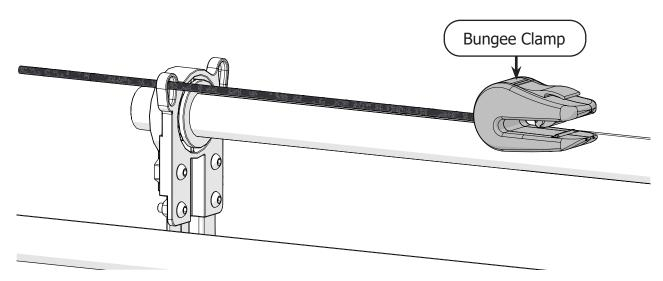
2 Press in the **bungee stop button** and thread the bungee clamp cord through the stop. Then release the stop.
