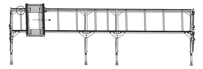
Note: Tighten the last connector bolt when the bottom carriage is just in front of it.
