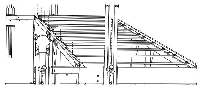
d Press down firmly on the bottom carriage and slide it across the frame a few times. This will align the loose track supports in the back.
