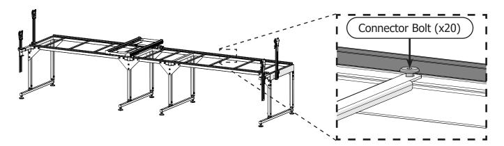
b Align the front track supports so they are flush with the front of the frame.
