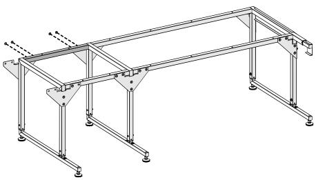
Loosely attach a long cross support tube to the front of the frame and left leg.
