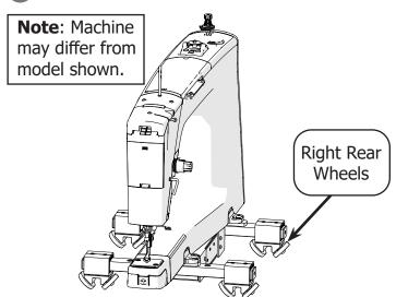
2 Use a 4 mm Allen wrench to remove the **outside wheel** and **wheel screw**. The wheel screw will not be needed again and can be stored with the packaging materials.
