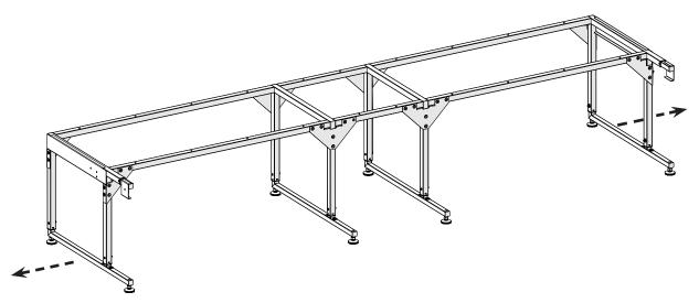
10 With the 4 mm Allen wrench, tighten the six connector bolts on each of the corner braces.
