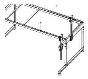
9 Tightly attach a table support onto the frame with the connector bolts you removed. As before, be careful not to shift the track supports.
