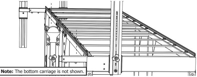
C Hold the front track supports in position and tighten the front connector bolts.
