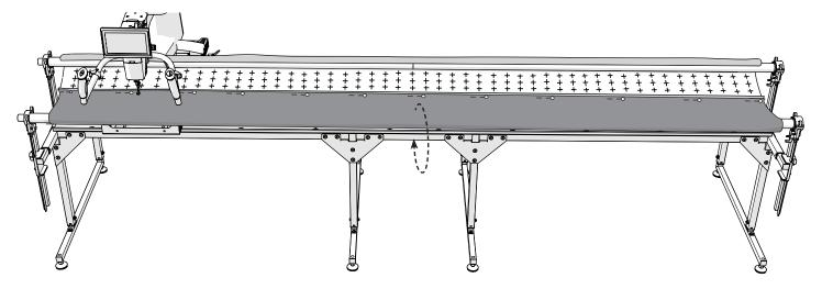
9 Pull the ratchet lever on the quilt-backing (front) rail down and hold it in place. Rotate the takeup rail forward and down to roll up all but a few inches of the cloth leader.
