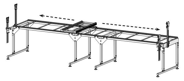
e Push the bottom carriage to the left side of the frame.
