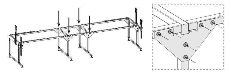
9 **Result:** The table is extended and all the cross support tubes are securely attached.
