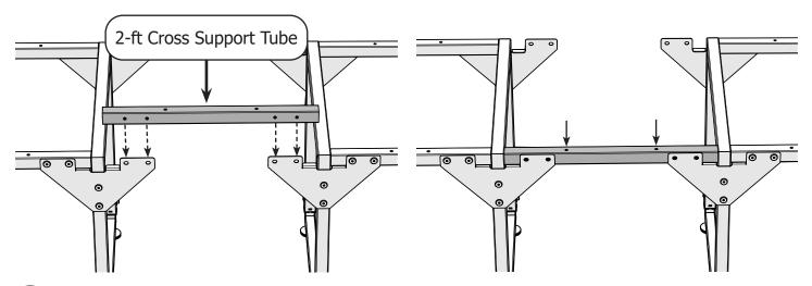
5 Loosely attach the cross support tube to the braces with four connector bolts.
