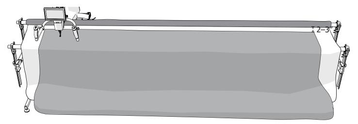
**Note:** Positioning the quit top 2–3 inches from the take-up rail ensures the machine's needle can reach all the quilt top edges within the frame. If the quilt top edge is too close to the take-up rail, the needle can not reach it. Keep this in mind whenever you roll your quilt to a new section.
