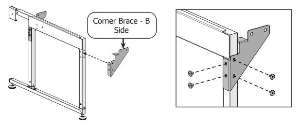
4 Use two connector bolts to loosely attach a **corner brace - B side** to the front of the **left leg assembly**.
