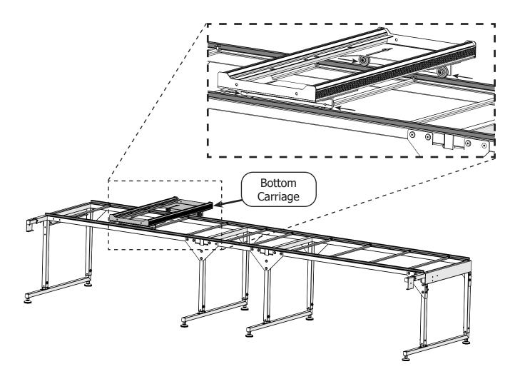
Press down firmly on the bottom carriage and slide it across the frame a few times. This will align the loose track supports in the back.
