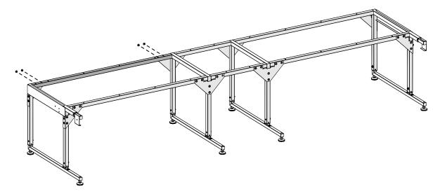
9 Pull the bottom of left and right legs outward to square up the frame.
