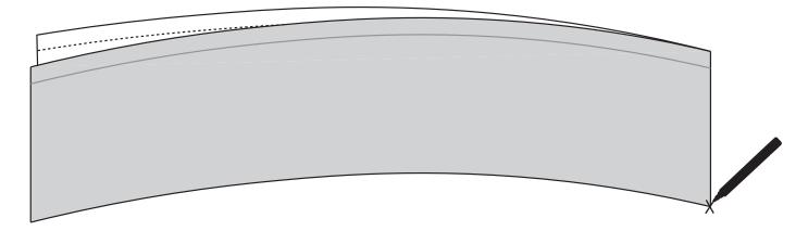
6 Attach one **cloth leader** to the Velcro on the take-up rail so the cloth drapes around the back of the rail. When attaching, start at the center of the rail and work your way outward one side at a time.
