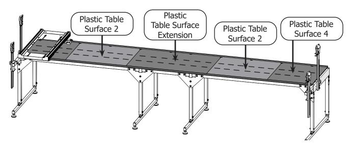
Test the spacing between the tracks and the table surfaces by rolling your bottom carriage across the frame. If the carriage wheels catch on the table surfaces, peel them up and reposition them to be more centered between the tracks.
