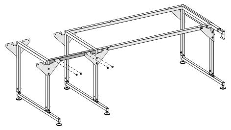
6 Loosely attach the second 2-ft cross support tube to the back of the frame with four connector bolts.
