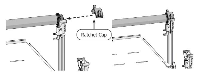
10 Repeat steps 7–9 to install the remaining rail into the front rail holder brackets, but do not pass the rail through the throat of the machine.
