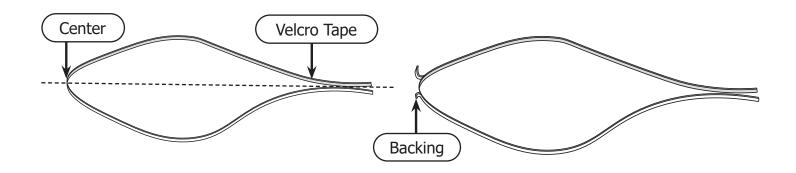
3 Stick the center of the Velcro tape over the **quilt-top rail** holes. Work from the center out and slowly spread the Velcro tape across the top of the quilt-backing rail.
