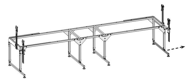
8 Use the 4 mm Allen wrench to tighten the sixteen connector bolts that you left loose task.
