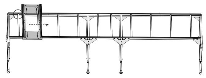
Note: Tighten the last connector bolt when the bottom carriage is just in front of it.
