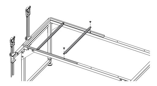
4 Place the **track support extensions** onto the middle of the frame. Align the vertical edges of the extended track supports with the vertical edges on the installed track supports.
