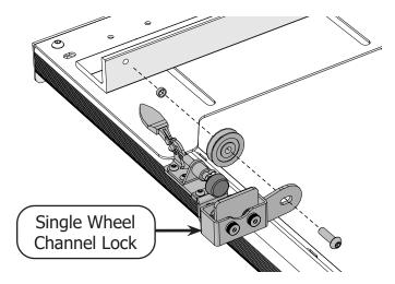
5 Press the channel lock against the wheel extrusion so it is square. Then fully tighten the screw.
