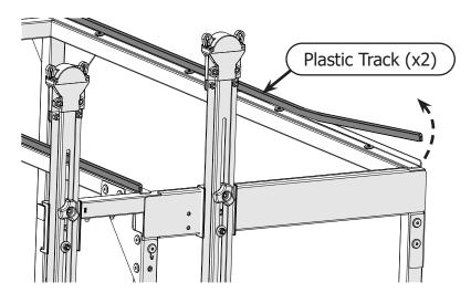
Use a 4 mm Allen wrench to remove the **connector bolts** and middle **track supports** from the frame. Set the eight connector bolts aside for later. The track supports can be discarded.
