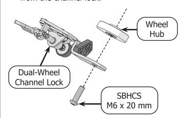
4 Screw the channel lock and wheel onto the machine so the channel lock body is toward the front of the machine. Use a 4 mm Allen wrench to attach.
