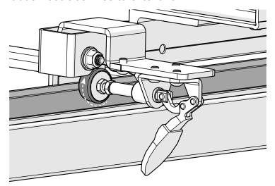
**Note:** If twisted too far, the channel lock handle will start to open, and eventually the foot will fall out. Reverse the direction you're twisting until the handle is pointing down, but the foot still reaches the track.
