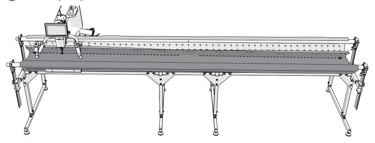
8 Roll the quilt-backing rail forward and down until the quilt backing is smooth and free of creases.
