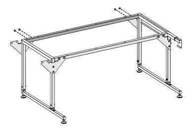
5 Loosely attach one of the 2-ft cross support tubes to the braces on the front of the frame and on the remaining middle legs. Use four connector bolts.
