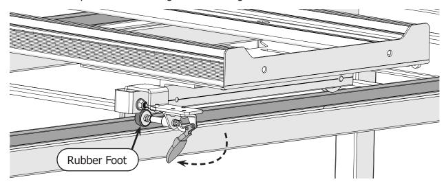
8 If the rubber foot doesn't fully reach the track or its grip on the track seems loose, twist the rubber foot clockwise to extend it.
