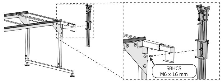
2 Attach the other right rail holder bracket to the right side of the frame.
