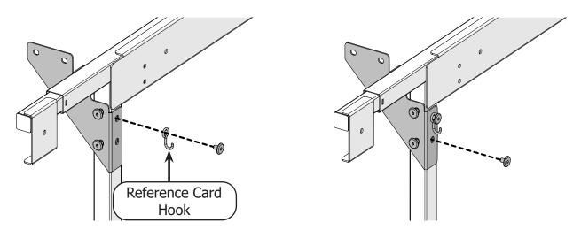
3 Loosely attach a **corner brace - B side** to the other side of the right leg with four connector bolts.
