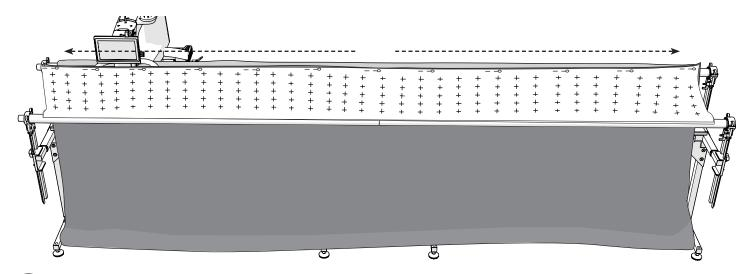
5 Roll the quilt-backing rail forward and down until there's only 1–2 feet of backing dangling under the rail.
