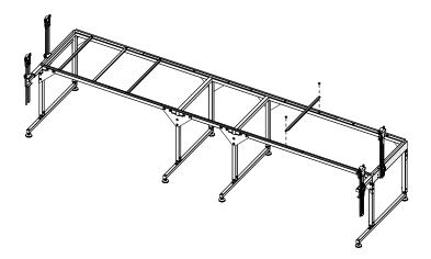
Tightly attach four more table supports onto the extended track supports.
