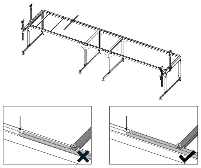
6 Repeat step 5 to attach a table support to the right end of the track supports, making sure the track support vertical edges stay aligned.
