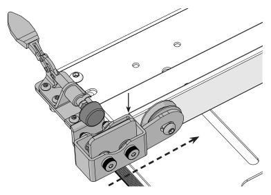
6 Place the bottom carriage back onto the frame so that the channel lock is toward the back. It should be on the right side of the bottom carriage.
