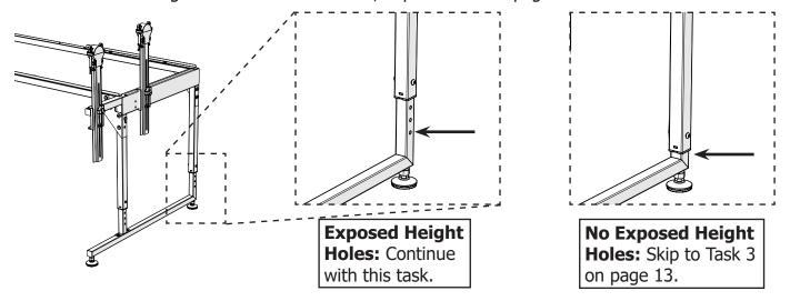
With the 4 mm Allen wrench and the 10 mm open-end wrench, remove the two sets of **height** screws, washers, and **nuts** from the new **middle leg assembly**.
