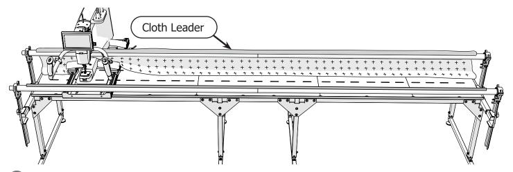
Attach the other cloth leader to the quilt-backing rail so the cloth drapes around the back of the rail. When attaching, start at the center of the rail and work your way outward.
