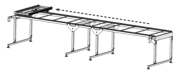
Slowly and firmly begin pushing the carriage to the other side of the frame. As you pass over each of the rear **M6 connector bolts**, tighten it with the 4 mm Allen wrench.
