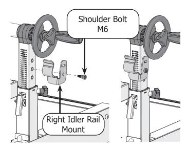
Pass the idler rail through the throat of the machine and place each end into the mounts.
