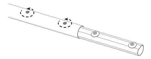
3 Slide one of the **2 ft rail sections** onto the other side of the rail coupler.
