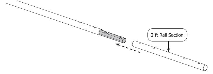
4 Align the holes with the coupler screws and turn the screws counter-clockwise with the 4 mm Allen wrench until they press firmly against the inside of the rail.
