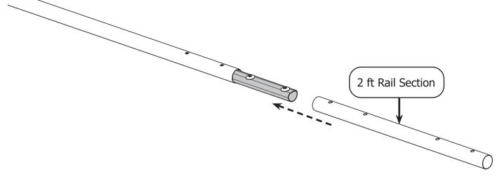
4 Align the holes with the coupler screws and turn the screws counter-clockwise with the 4 mm Allen wrench until they press firmly against the inside of the rail.
