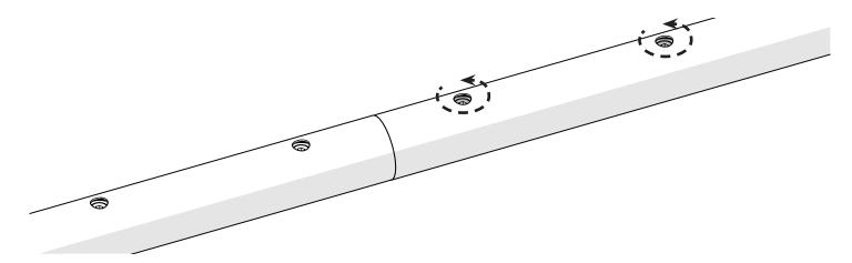
5 Loosen the 3-armed knobs on the take up rail arms on both sides of the frame.
