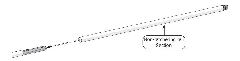
4 Align the holes with the coupler screws and turn the screws counter-clockwise with the 4 mm Allen wrench until they press firmly against the inside of the rail.
