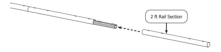
8 Slide the third rail coupler into the free end of the 2 ft rail section. Use the 4 mm Allen wrench to turn the screws counter-clockwise until the rail coupler is held firmly in place.
