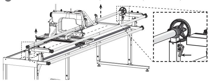
The mount holding the idler rail is installed on two of the 3 holes on the take-up rail arm. Choose whether to install the mount on the top two or bottom two holes by considering the size of your machine.
