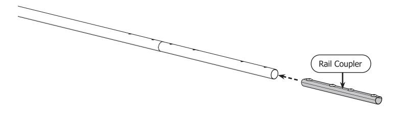
Once again, turn the screws counter-clockwise with the 4 mm Allen wrench until the rail and coupler are snug.
