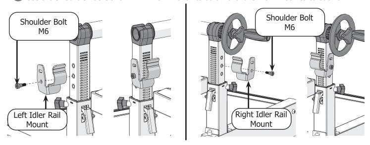
14 Pass the idler rail through the throat of the machine and place each end into the mounts.
