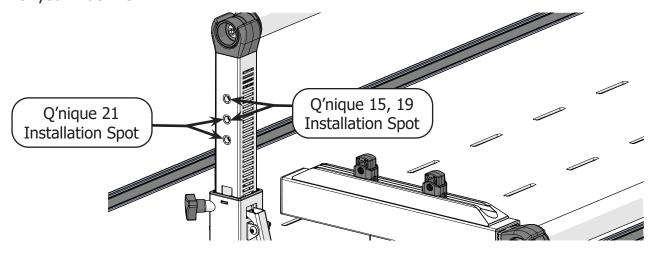
8 Use the **shoulder bolt** and 4 mm Allen wrench to screw the **idler rail mounts** to each arm.
