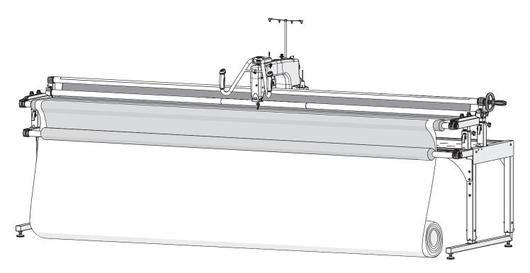
Check your rail hieght to make sure there is a finger's width of space between the idler rail and the floor of the machine. See "Setting the Rail Height" on page 29 for detailed instructions.
