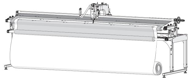
4 Twist the knobs on the two front rail arms to loosen the tension on the fabric.
