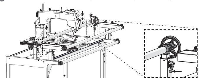
The mount holding the idler rail is installed on two of the 3 holes on the take-up rail arm. Choose whether to install the mount on the top two or bottom two holes by considering the size of your machine.
