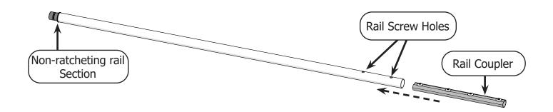
2 Use a 4 mm Allen wrench to turn the screws inside the rail counter-clockwise until they press firmly against the rail.
