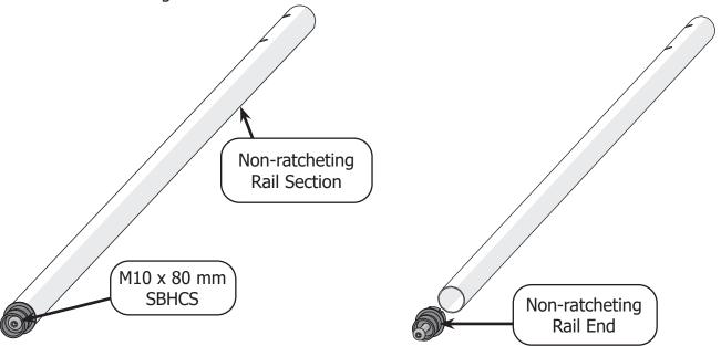
Use the 6 mm Allen wrench to screw the **non-ratcheting rail ends** to the free ends of one of the **5 foot rail segments** from your base frame.
