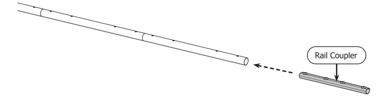
9 Install the remaining **non-ratcheting rail section** onto the other side of the rail coupler. Use the 4 mm Allen wrench to turn the coupler screws counter-clockwise.
