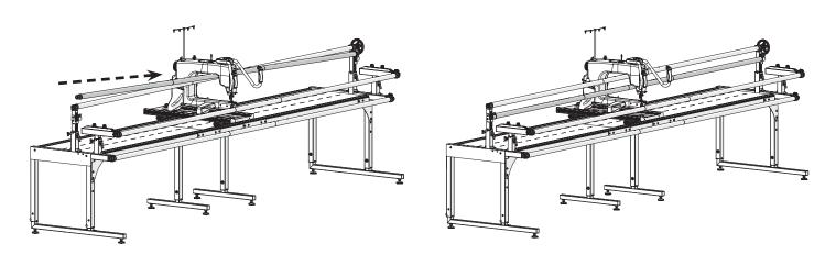
Push in on the mount and install the **3-armed knob**. To remove the frame in the future, simply loosen the **3-armed knob** and lift the rail out of the mounts.
