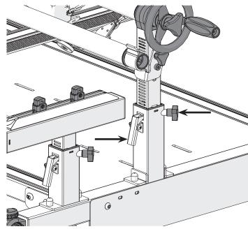
2 Set the idler rail so it has about a **finger's** width of space between it and the floor of the quilting machine.
