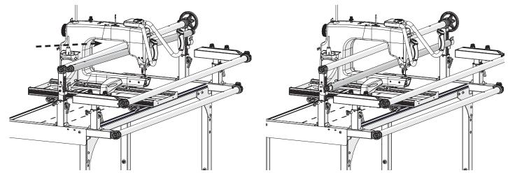
8 Push in on the mount and install the **3-armed knob**. To remove the frame in the future, simply loosen the **3-armed knob** and lift the rail out of the mounts.
