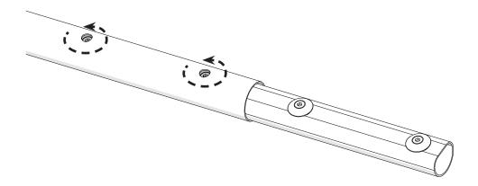
3 Slide the remaining **non-ratcheting rail section** onto the other side of the rail coupler.
