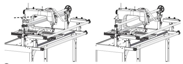
Push in on the mount and install the **3-armed knob**. To remove the frame in the future, simply loosen the **3-armed knob** and lift the rail out of the mounts.
