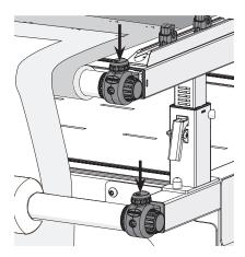
5 Re-install the idler rail into the idler mounts, over the top of the fabric.
