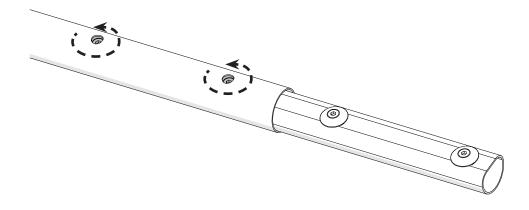
Install the remaining **non-ratcheting rail section** onto the other side of the rail coupler. Use the 4 mm Allen wrench to turn the coupler screws counter-clockwise.
