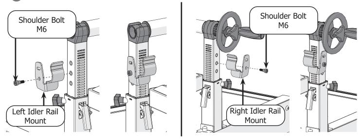
12 Pass the idler rail through the throat of the machine and place each end into the mounts.
