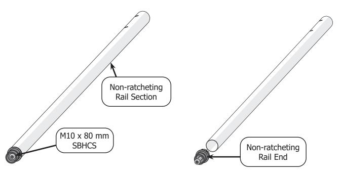
2 Screw the **non-ratcheting rail end** into the free end of the remaining **non-ratcheting rail section.**
