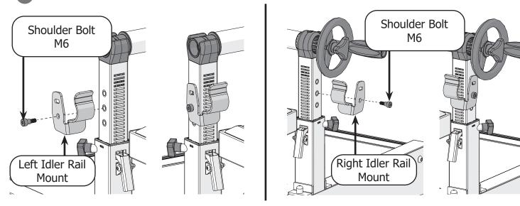
9 Pass the idler rail through the throat of the machine and place each end into the mounts.
