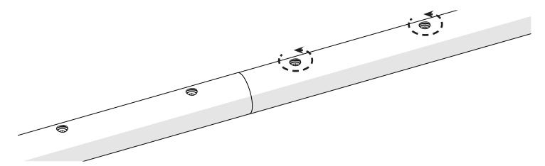
5 Now insert a second coupler into the 2 ft rail section.
